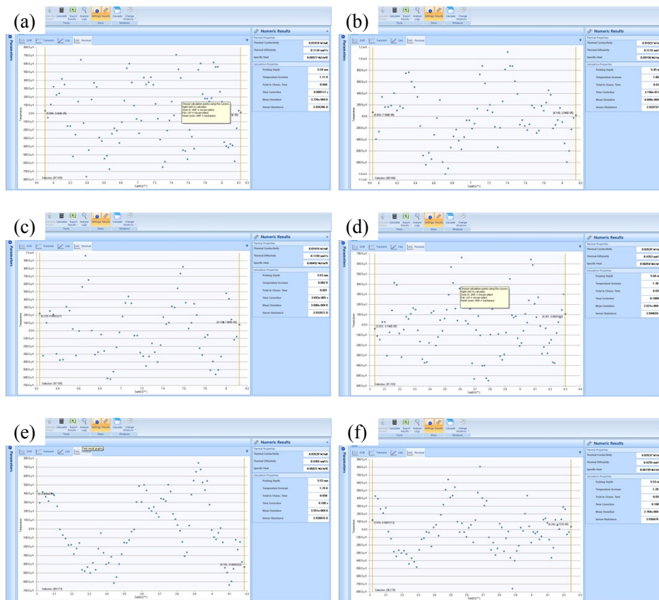
Fig. S2 Thermal conductivity measurement graph of N-doped graphene aerogels with 6 mg/ml GO suspension at 5Pa (a ~ c) and atmospheric pressure (d ~ f)
