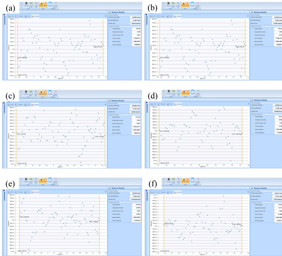
Fig. S3 Thermal conductivity measurement graph of N-doped graphene aerogels with 9 mg/ml GO suspension at 5Pa (a ~ c) and atmospheric pressure (d ~ f)
