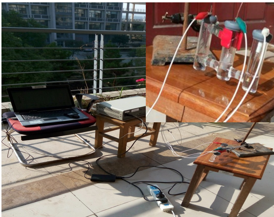
Figure S6 The photo of outdoor equipment of sunlight-driven PEC hydrogen production over g- C_3N_4/NiO photocathode during 4 h under sunlight irradiation in Wuxi city on Dec. 26, 2016. Outdoor temperature: 4–14 oC, time: 10:15–14:15.
