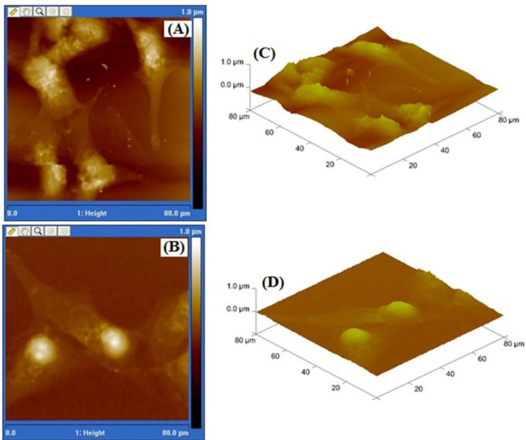
**Fig. S2.** 2-D (A and B) and 3-D (C and D) topographic AFM height images of U87-MG/RGDC/Gold/ITO (A and C) and U87-MG/TATC/Gold/ITO (B and D) modified electrode surface.
