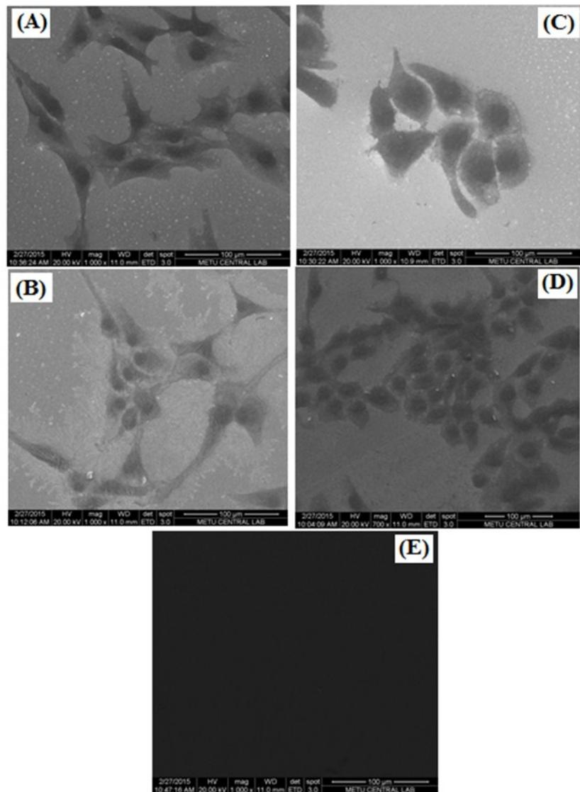
**Fig. S3.** Surface characteristics of (A) U87-MG/RGDC/Gold/ITO (B) U87-MG/TATC/Gold/ITO (C) Vero/RGDC/Gold/ITO (D) Vero/TATC/Gold/ITO and (E) Gold/ITO via SEM images.
