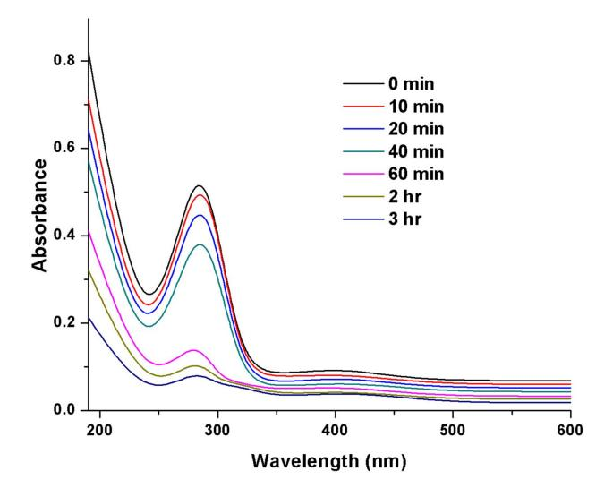
Fig S2: Absorbance spectrum of 4-CP with time in presence of ZFC under solar
