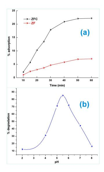
Fig S3 : (a) Adsorption of 4-CP onto ZF and ZFC in the dark experiment (b) Influence of initial ph on degradation of 4-CP in presence of ZFC under solar light
