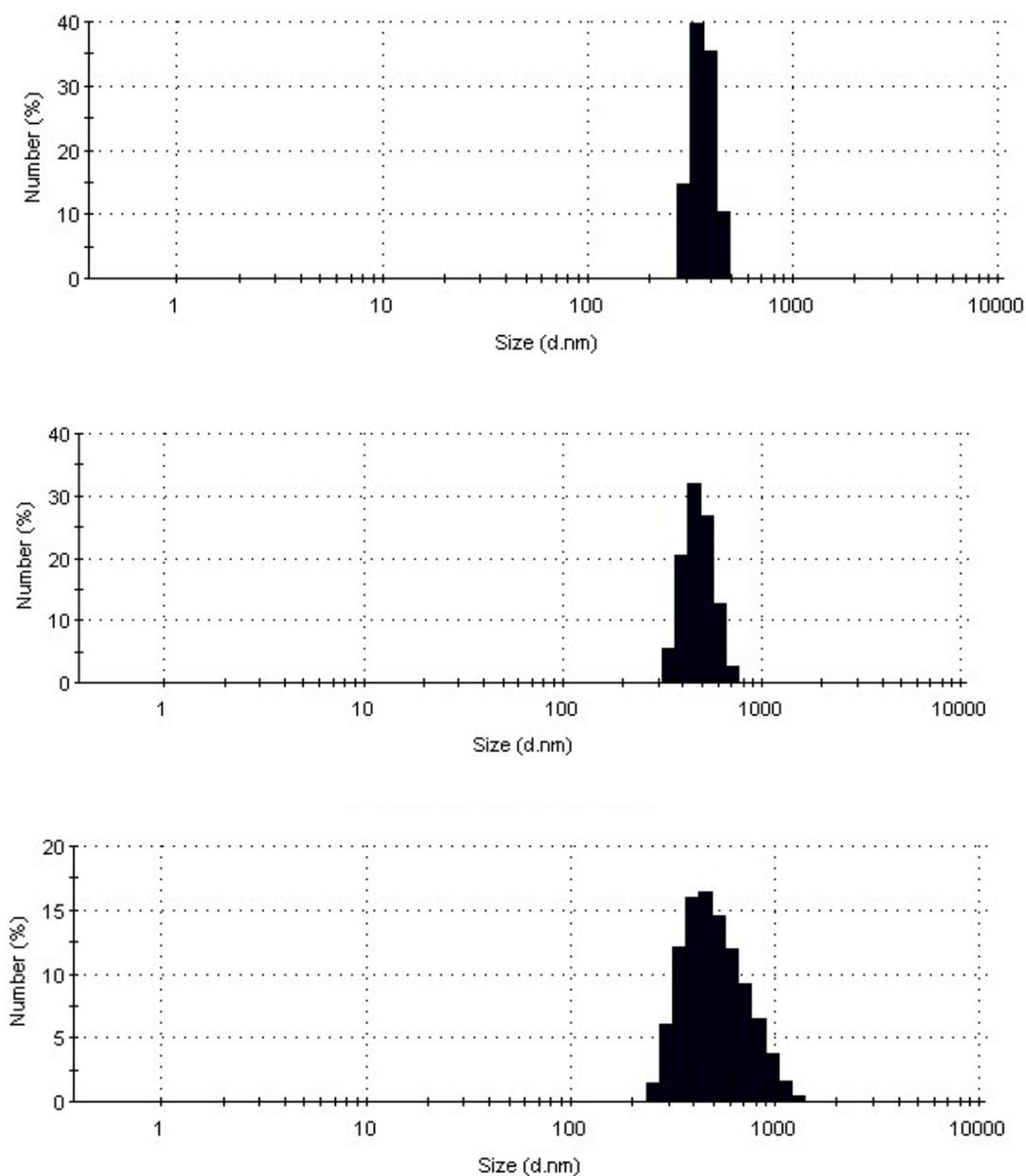
**Figure S8.** DLS histograms of PEG-*b*-PC copolymer in THF (0.5 mg/ml) after subsequent addition of water to obtain THF/water volumetric ratios of 4:1; 2:3 and 1:4 (top to bottom).
