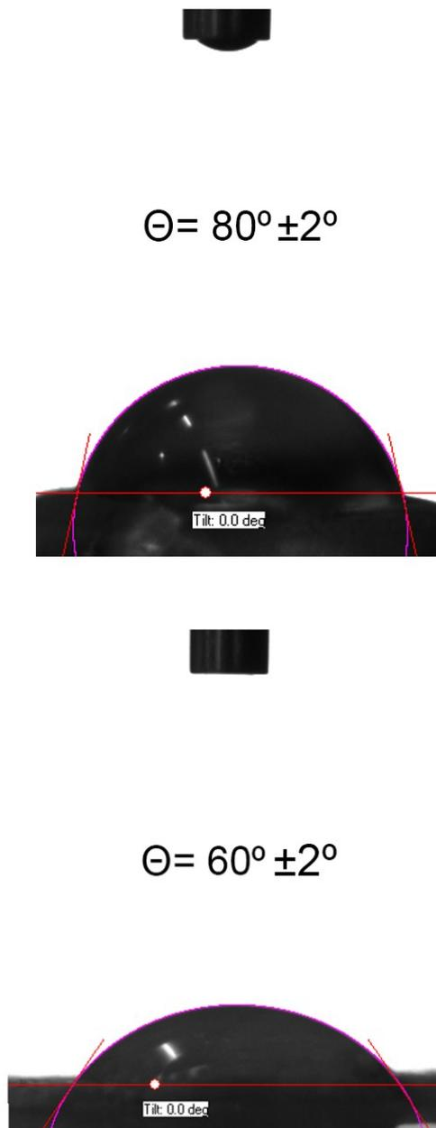
**Figure S1.** Contact angle of the polycarbonate starting materials (top) and PEG-*b*-PC copolymer (bottom).
