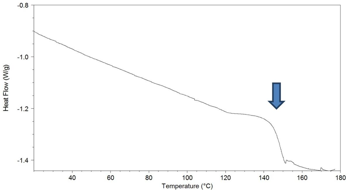
**Figure S4.** DSC trace (conventional mode) of the PC starting material.
