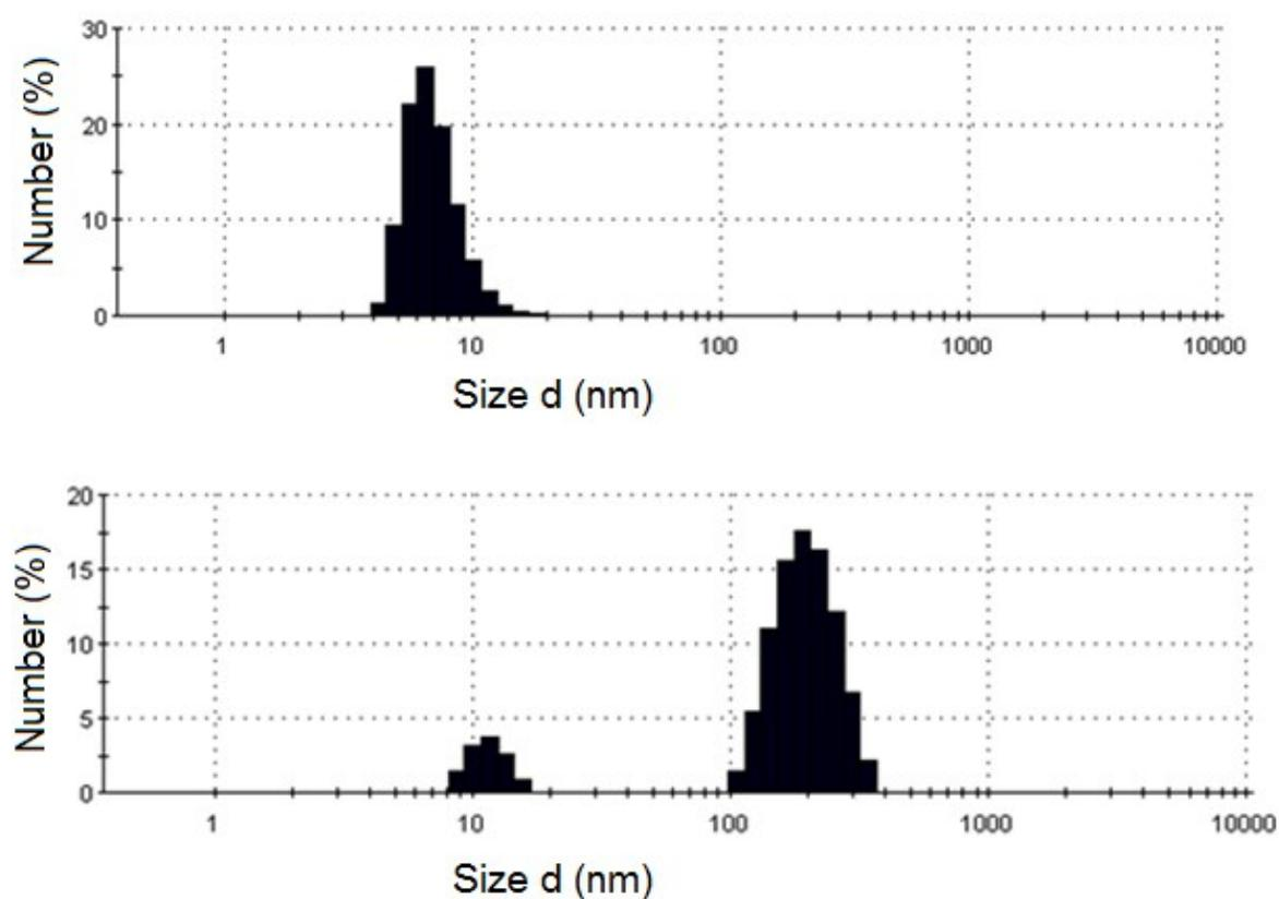
**Figure S7.** DLS histograms of PEG-*b*-PC copolymer in THF after ultrasonication (top) and after a rest period of ~2h (bottom).
