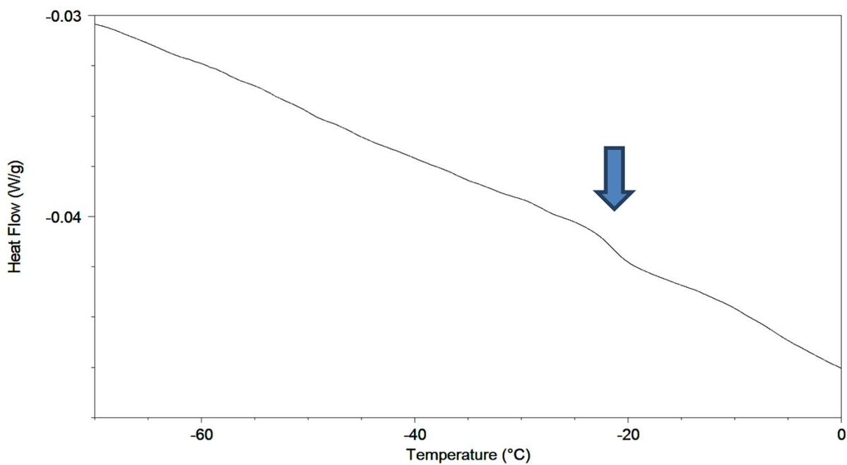
**Figure S6.** DSC trace (modulated mode) of the mPEG-OH starting material.
