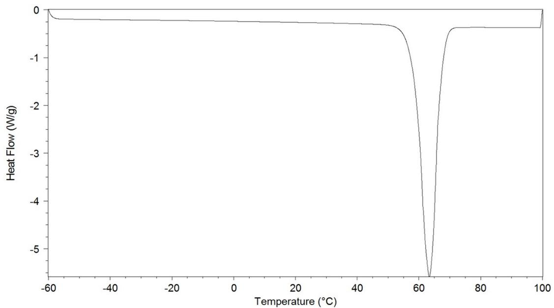
**Figure S5.** DSC trace (conventional mode) of the mPEG-OH starting material.
