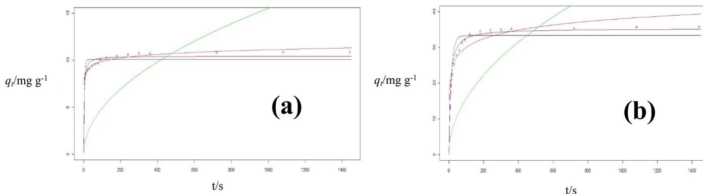
**Fig S5:** Comparison of kinetics models fitted to the experimental data for the adsorption of  $\text{Cu}^{2+}$  onto (a) MWCNT-COOH and (b) MWCNT-ttpy (pseudo-first order —, pseudo-second order —, intraparticle diffusion — and Elovich model —).
