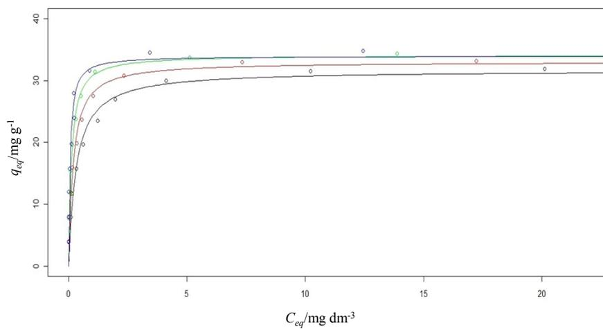
**Fig S7:** The Langmuir adsorption isotherm fitted to the experimental data for the adsorption of  $\text{Cu}^{2+}$  onto MWCNT-tpy at various temperatures (293 K —, 303 K —, 313 K — and 318 K — ).
