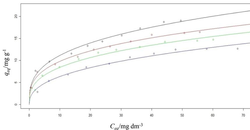
**Fig S6:** The Freundlich adsorption isotherm fitted to the experimental data for the adsorption of  $\text{Cu}^{2+}$  onto MWCNT-COOH at various temperatures (293 K —, 303 K —, 313 K — and 318 K — ).
