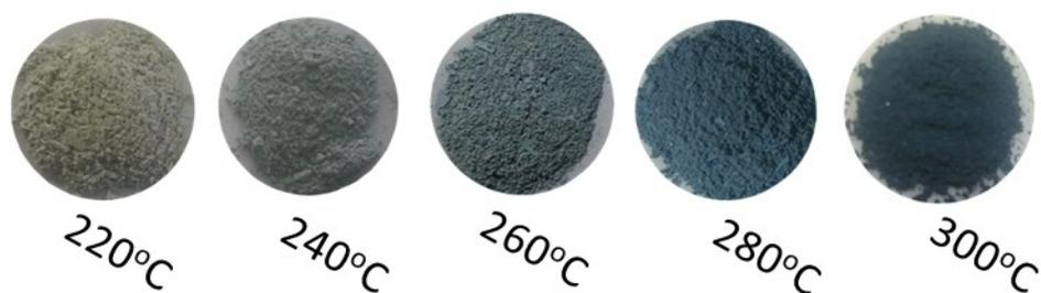
**Fig. S1.** The digital photos of the hydrogenated ultrathin  $\text{TiO}_2$  nanosheets.
