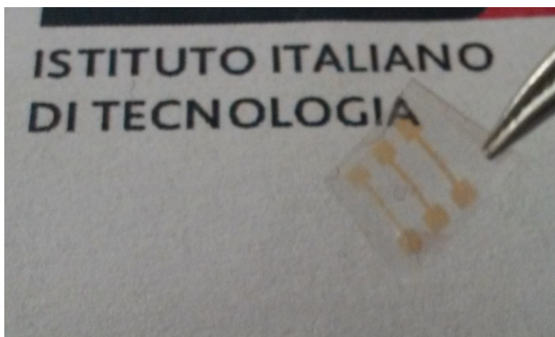
Figure S31 Free standing film in which different electrode-like structures were patterned
