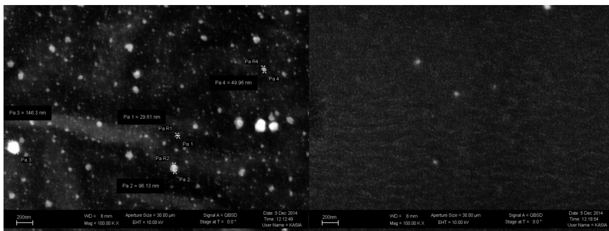
Figure S25 Magnification of Figure 6a: top (left) and bottom (right) part of the cross section of PEGDMA + 5 phr AgNO 3 after 10 minutes of UV irradiation: few NPS are present in the upper part while the rest is almost neat.
