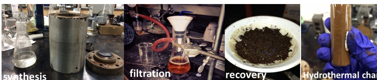
Figure SI-1. Photographs of HTC synthesis, filtration, recovery, and dried product.
