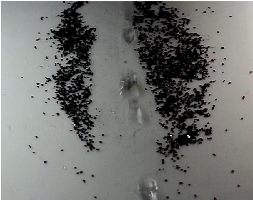
**Fig.S7** the digital picture of carbon black particles carried off from the LET-covered glass slide by the rolling water droplets.
