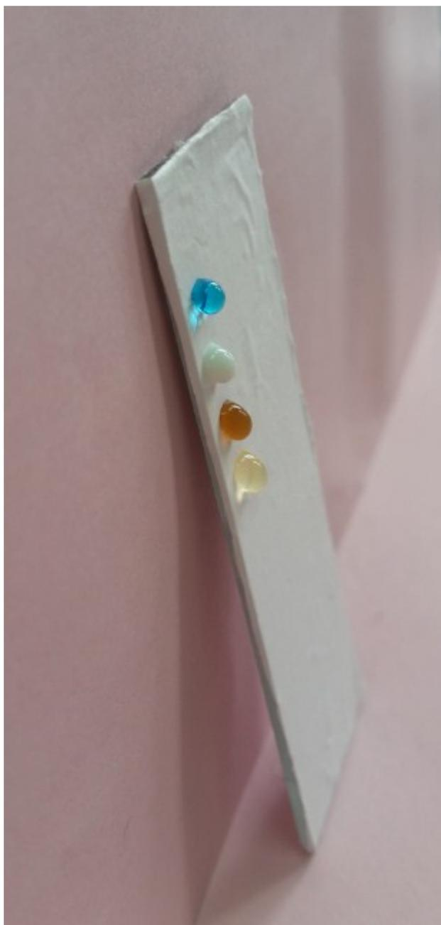
**Fig. S1** Sticking droplets of water, milk, coffee and juice on the almost upright surface of electrospun PVDF mat.
