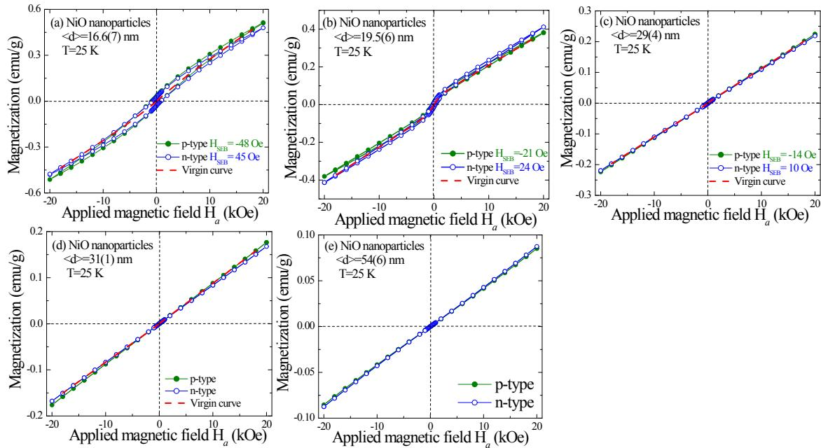
**Figures S3 (a)-(e)** Full magnetization hysteresis  $M(H_a)$  loops measured at different temperatures of 2, 25, 50, 100, 200 and 300 K with the *p*-type protocol after zero-field cooling for 16.6(7) to 54(6) nm NiO nanoparticles.
