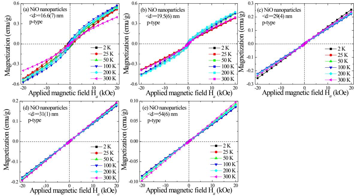
**Figures S4 (a)-(e)** Full magnetization hysteresis  $M(H_a)$  loops measured at different temperatures of 2, 25, 50, 100, 200 and 300 K with the *n*-type protocol after zero-field cooling for 16.6(7) to 54(6) nm NiO nanoparticles.
