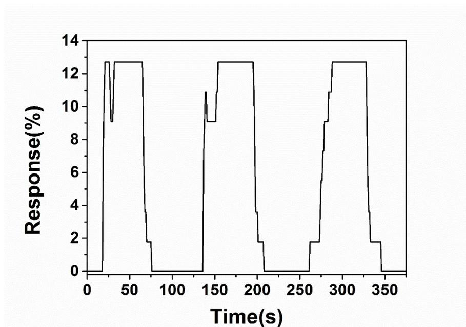
Figure S2. Gas response plot of CdO NFAs on glass substrate to 100 ppm DEE at the temperature of 215 °C
