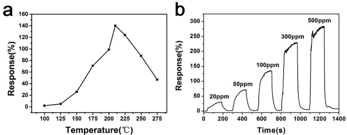
Figure S3. The gas sensing properties of DL400. (a) Response to 100 ppm DEE at different operating temperatures, (b) dynamic response to DEE at different concentrations ranging from 20 to 500 ppm at 215 °C.
