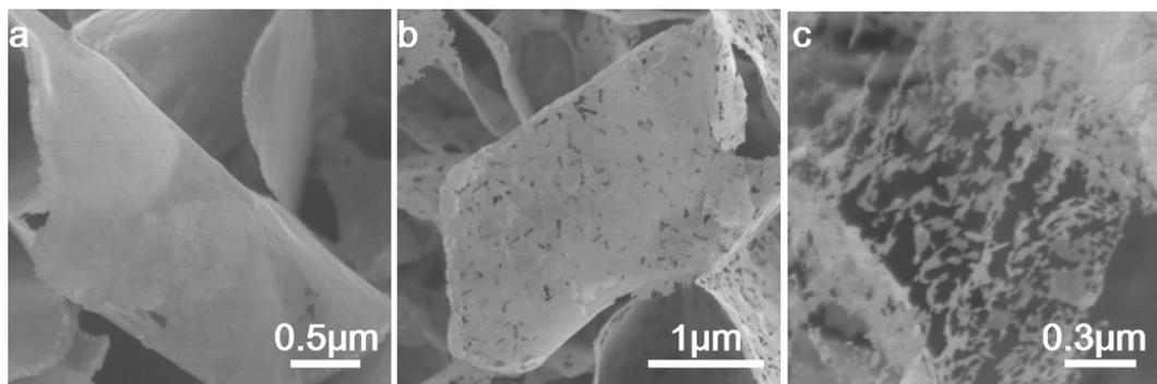
Figure S4. The SEM images of single nanoflake in (a) N-NFAs, (b) P-NFAs, and (c) S-structure.
