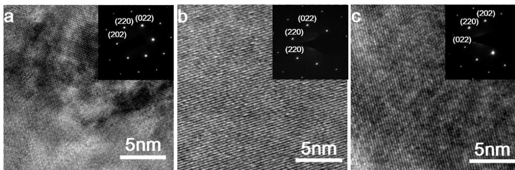
Figure S6. HRTEM images of (a) N-NFAs, (b) P-NFAs, and (c) S-structure and their diffraction patterns (insets).
