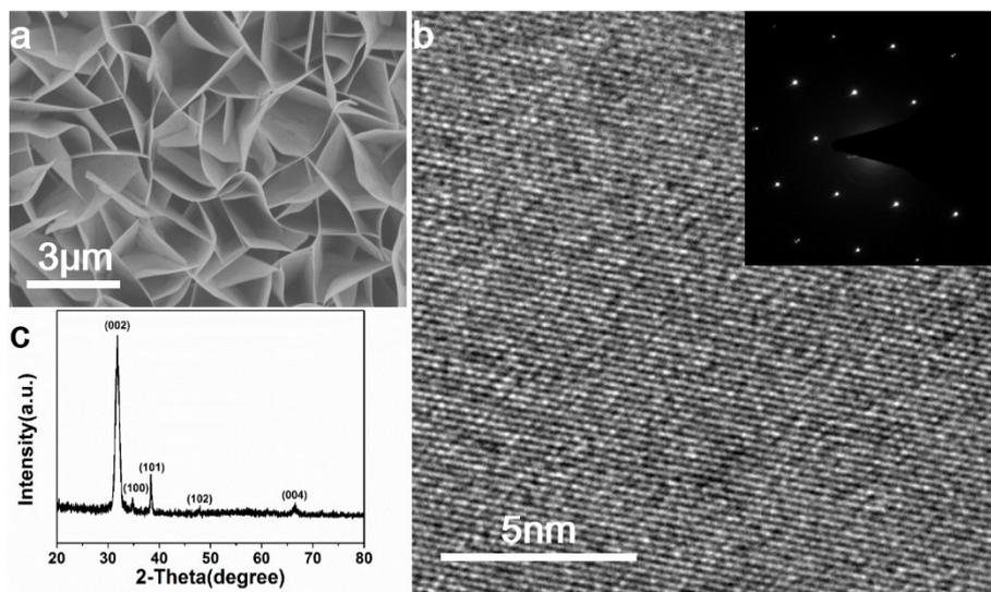
Figure S1.Characterizations of Cd NFAs. (a) SEM images of Cd NFAs from the top view, (b) HRTEM image and SAED pattern (insert), (c) XRD pattern of Cd NFAs.
