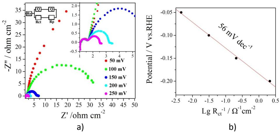
**Figure S8.** a) Nyquist plots and the equivalent circuit and b) The plots of overpotential vs.  $\lg R_{ct}^{-1}$  for MoP/N,P-CNT and its linear fitting for data obtained in 0.5 M H<sub>2</sub>SO<sub>4</sub>.
