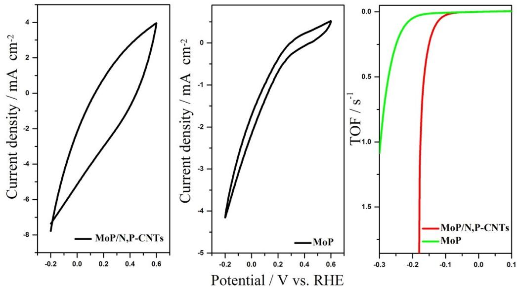
**Figure S10.** Cyclic voltammograms for MoP/N,P-CNTs a) and for b) bulk MoP in phosphate buffer, and c) TOF versus overpotential curves of MoP/N,P-CNTs and bulk MoP in 0.5 M H<sub>2</sub>SO<sub>4</sub>.
