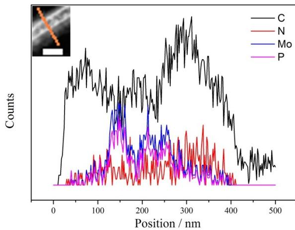
**Figure S1.** ADF STEM image and the corresponding EDX elemental scanning mappings of MoP/N,P-CNTs.
