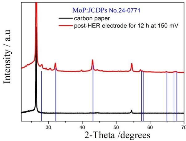
**Figure S11.** XRD pattern of the post-HER electrode after continuous water electrolysis at given overpotential of 150 mV for 12 h in 0.5 M H<sub>2</sub>SO<sub>4</sub>.
