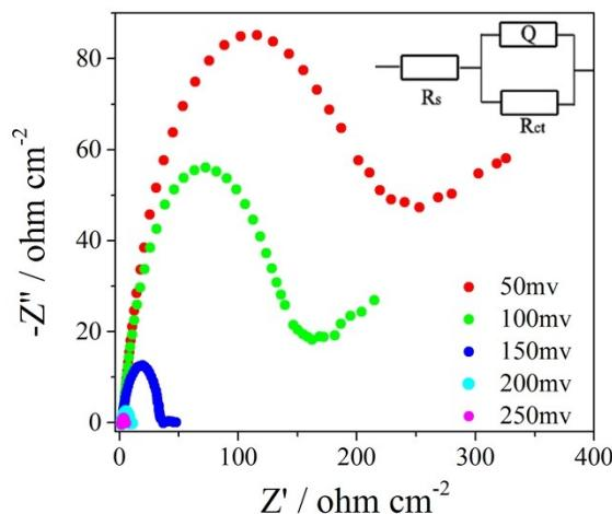
**Figure S13.** Nyquist plots and the equivalent circuit of the bulk MoP at various HER overpotentials in 0.5 M H<sub>2</sub>SO<sub>4</sub>.
