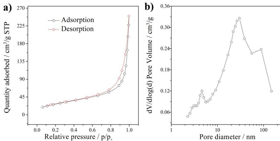
**Figure S4.** a) Nitrogen adsorption and desorption isotherms and b) the pore size distribution curve of MoP/N,P-CNTs.
