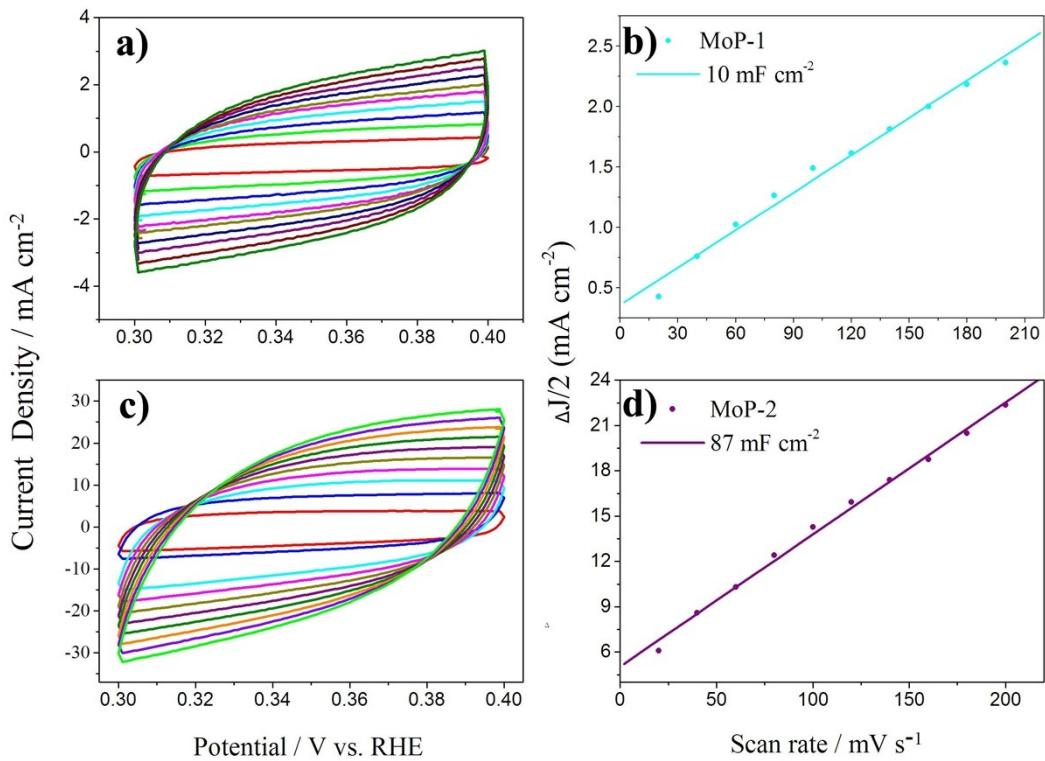
**Figure S19** Cyclic voltammograms for (a) MoP-1 and (c) MoP-2 in the region of 0.3–0.4 V vs. RHE in 0.5M H<sub>2</sub>SO<sub>4</sub>; The differences in current density ( $\Delta J = J_a - J_c$ ) for (b) MoP-1 and (d) MoP-2 at 0.35 V vs. RHE plotted against scan rate fitted to a linear regression allows for the estimation of C<sub>dl</sub>.
