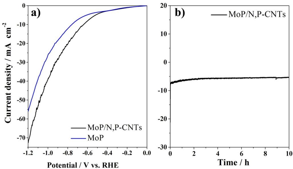
**Figure S9.** a) Polarization curves of MoP/N,P-CNTs in phosphate buffer and b) stability of MoP/N,P-CNTs at a given overpotential of 600 mV in phosphate buffer.
