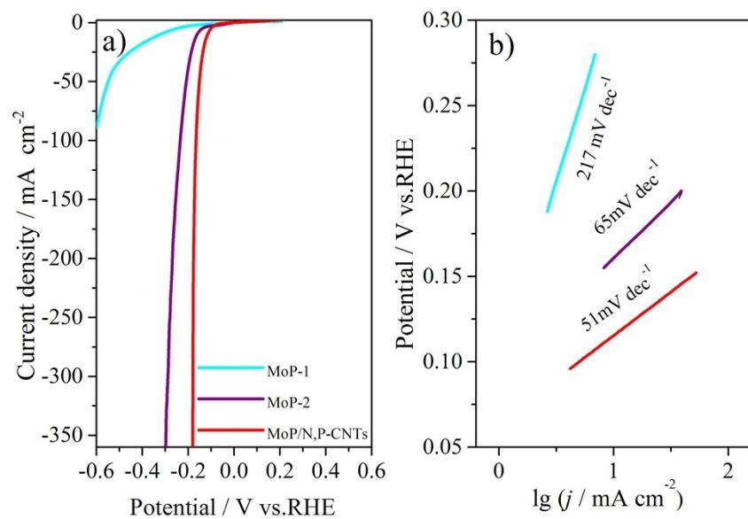
**Figure S17.** a) Polarization curves and b) Tafel plots of MoP/N,P-CNTs, MoP-1 and MoP-2 in 0.5 M H<sub>2</sub>SO<sub>4</sub> solution.
