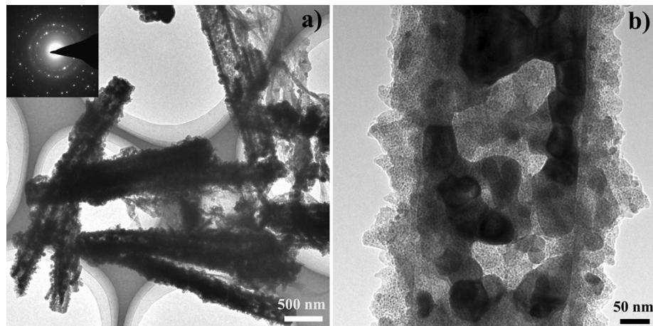
**Figure S12.** TEM images of MoP/N,P-CNTs scraped off from the post-HER electrode. a) Low-resolution TEM image and b) high-resolution TEM image, and the inset in a) shows the corresponding SAED pattern.
