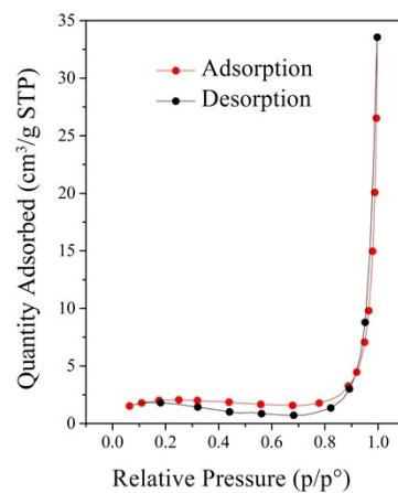
**Figure S7.** Nitrogen adsorption and desorption isotherms of P-PANI.
