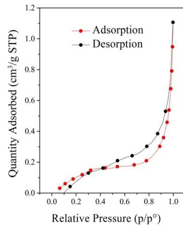
**Figure S6.** Nitrogen adsorption and desorption isotherms of bulk MoP.
