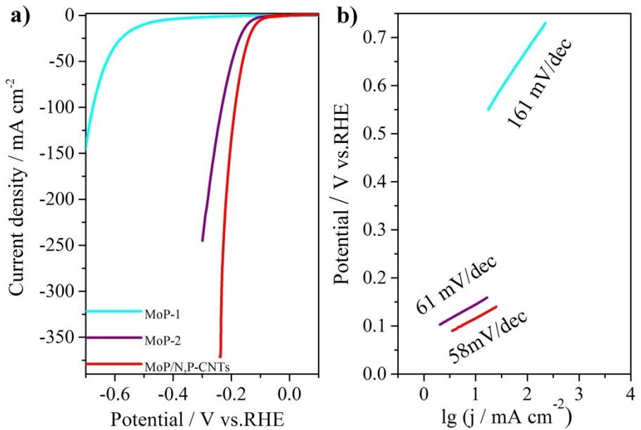
**Figure S18** a) Polarization curves and b) Tafel plots of MoP/N,P-CNTs, MoP-1 and MoP-2 in 1.0 M KOH solution.
