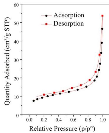
**Figure S5.** Nitrogen adsorption and desorption isotherms of MoO<sub>2</sub>/N,P-CNTs.
