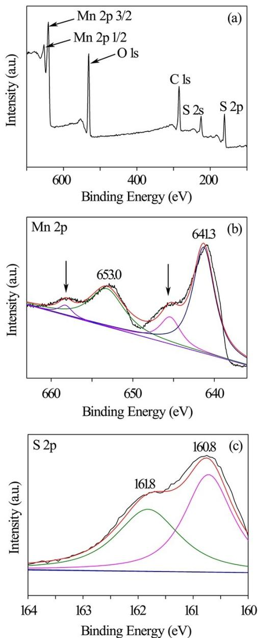
The X-ray photoelectron spectrometry (XPS) analysis of the MnS aggregations is shown in Figure S1. The molar ratio of Mn and S was calculated to be approximately
