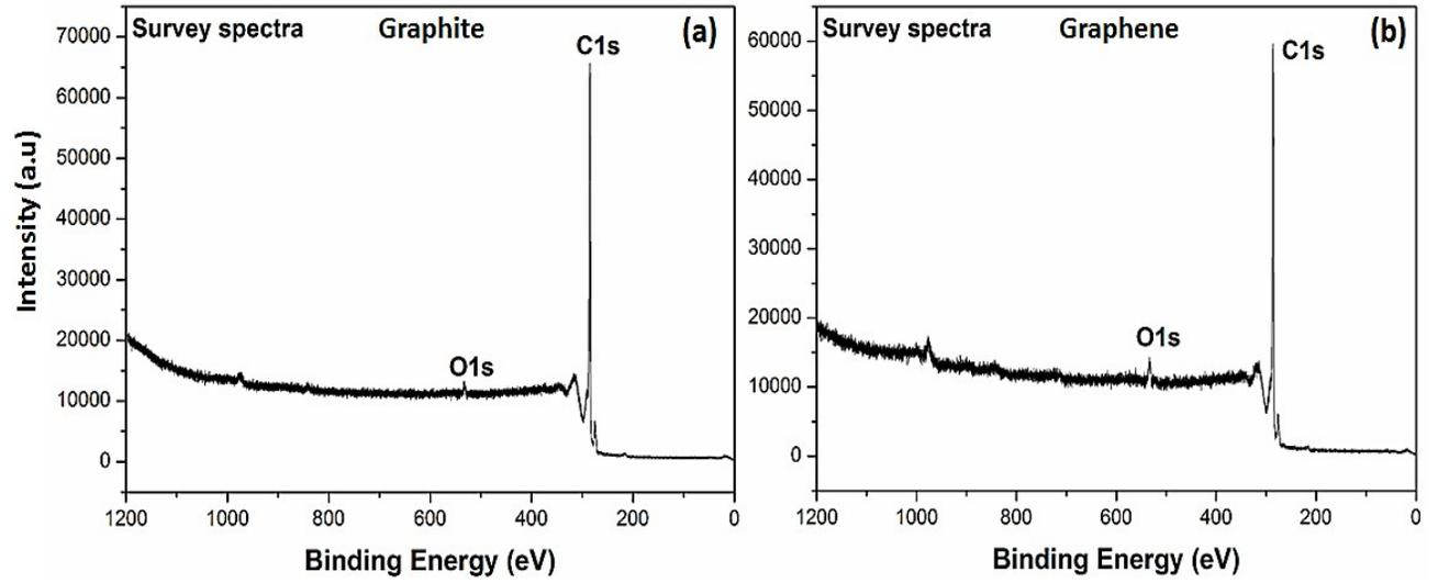
Figure S3. XPS Survey spectra of Graphite and Graphene
