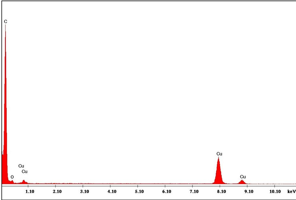
**Figure S2.** Energy Dispersive X-ray spectra of synthesized graphene sheets.
