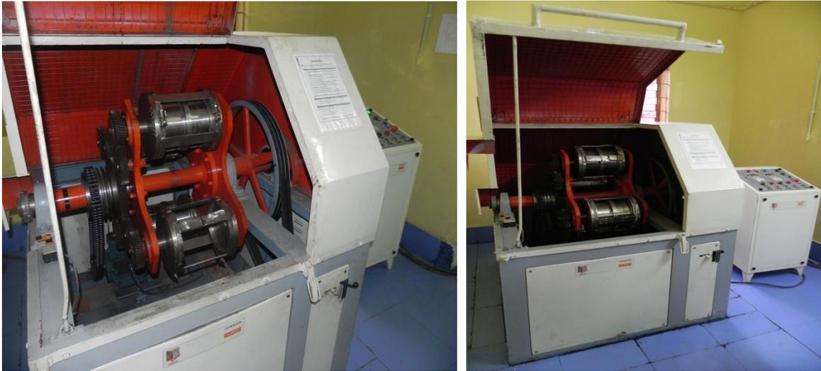
**Figure S1.** The Real image of Dual Drive Planetary Ball milling system used in this experiment.
