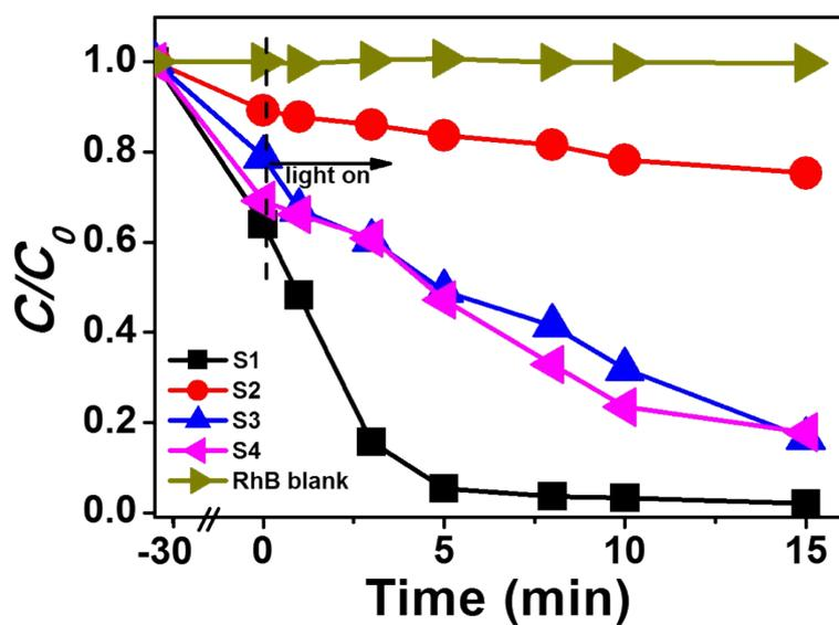
**Figure S3.** Photosensitization activity for RhB degradation over as-prepared BiOCl samples (S1~S4) under visible light irradiation ( $\lambda > 420$  nm).
