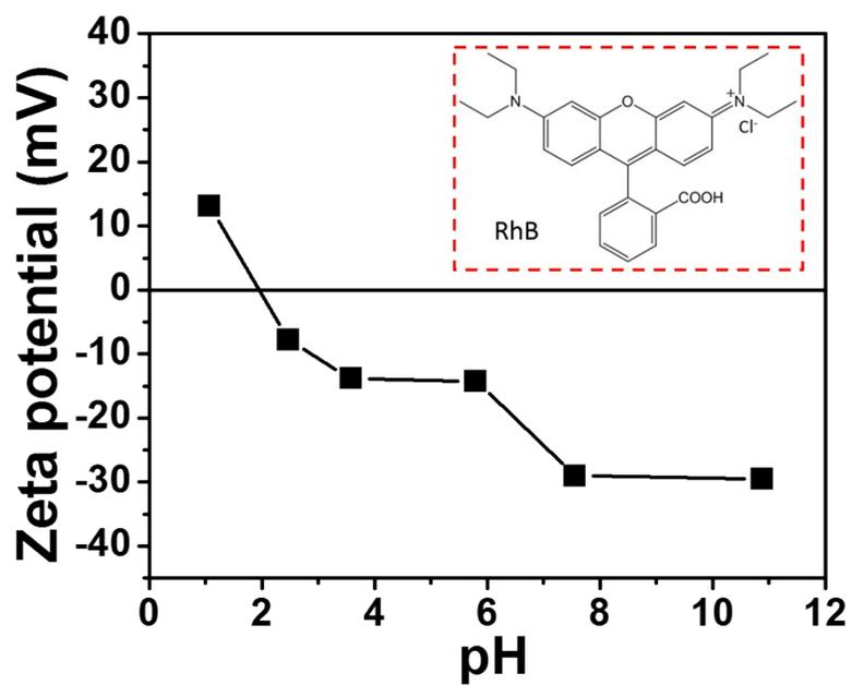
**Figure S4.** The zeta potential of BiOCl HN (S1) in the RhB ( $5 \times 10^{-6}$  M) solution under different pH values (inset is the molecular structure of RhB).
