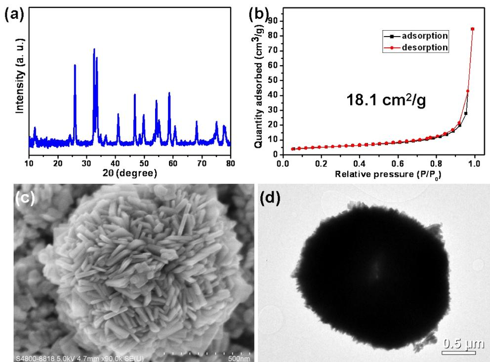
**Figure S2.** XRD pattern (a), nitrogen adsorption/desorption isotherm (b), SEM image (c) and TEM image (d) of the as-synthesized BiOCl hierarchical nanostructures using  $\text{CoCl}_2$  in the presence of 0.2 g citric acid (S4).
