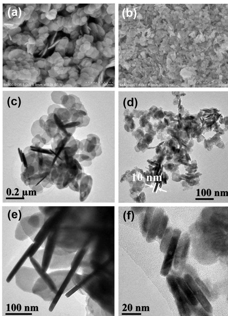
**Fig. S1** SEM images (a~b) and TEM images (c~f) of the as-synthesized BiOCl nanostructures using NaCl at different amounts of citric acid: 0 g (a, c and e, **S2**) and 0.05 g (b, d and f, **S3**).
