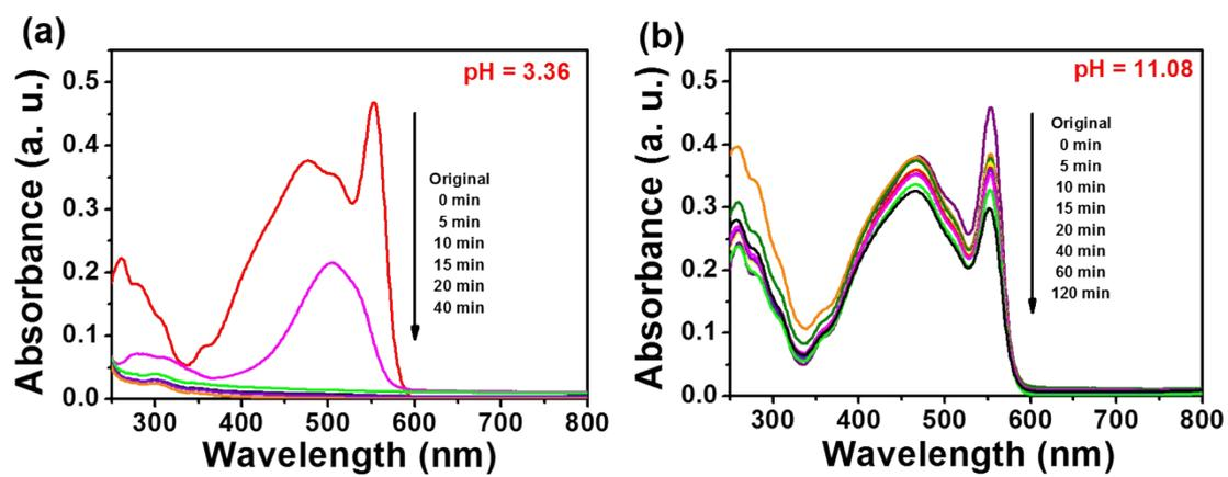
Figure S5. Photodegradation efficiency of the RhB-sensitized BiOCl HN (S1) for MO at different pH values.
