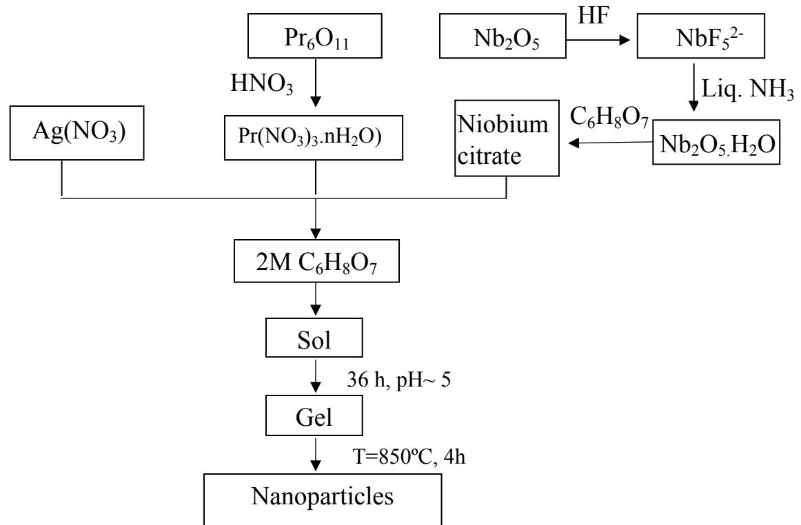
**Figure SF1.** Flow chart of the synthesis of  $\text{Ag}_{3(2+x)}\text{Pr}_x\text{Nb}_{4-x}\text{O}_{11+\delta}$
