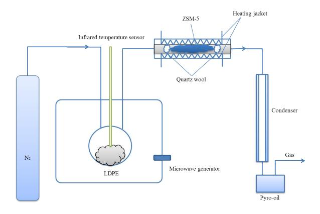
Fig. S1 The schematic diagram of the microwave-assisted degradation system integrated with catalysis process
