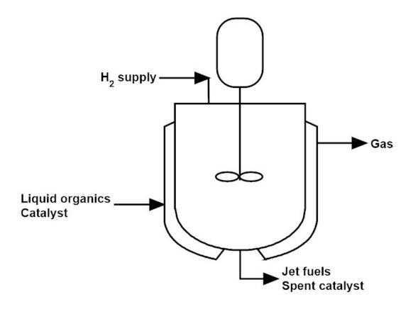
Fig. S2 The schematic overview of the hydrotreating process set-up
