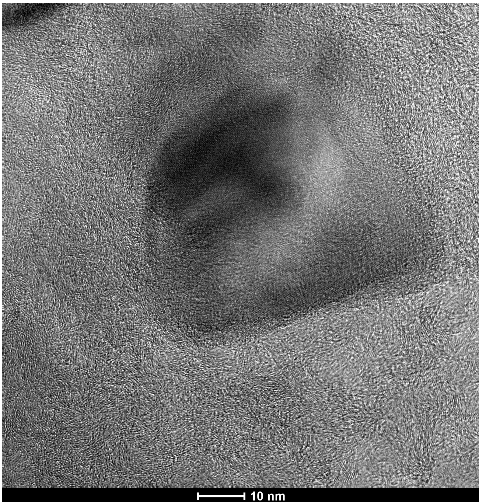
Fig. S1. The TEM image of the structure of Si nanoparticles wrapped in PAN-based turbostratic
