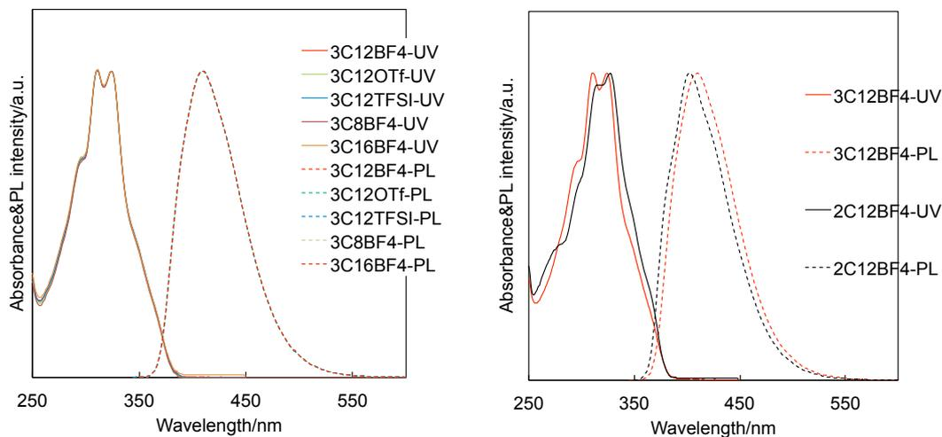
**Figure S48.** UV-vis and fluorescence spectra of five fused  $\pi$ -conjugated imidazolium compounds in DCM ( $10^{-5}$  M). Left: Influence of alkyl chain length and counter anion. Right: Influence of a number of alkoxy chains. The excitation wavelengths were that of the absorption maxima.
