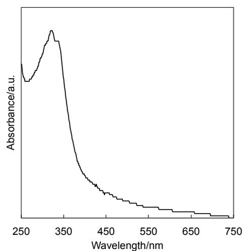
**Figure S50.** UV-vis spectrum of **3C12BF4** in solid state.
