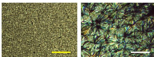
**Figure S38.** POM images of **3C12TFSI** at 25 °C. Images were captured after cooling from isotropic liquid and kept still standing for 1 day. Yellow and white scale-bars shown in images denote 200 $\mu$ m and 40 $\mu$ m, respectively.
