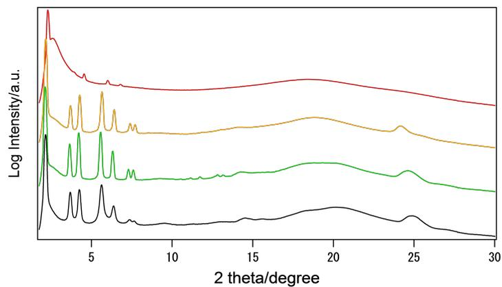
**Figure S42.** VT-XRD patterns of **3C16BF4** at 25 °C (black), 70 °C (green), 150 °C (orange), and 220 °C (red).
