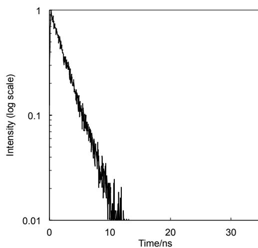
**Figure S52.** Fluorescence decay curve of **3C12BF4** in  $\text{CH}_2\text{Cl}_2$  by irradiating at 375 nm and monitoring at 420 nm.
