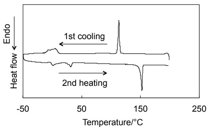
**Figure S35.** DSC thermogram of **3C12BF4ref** in first cooling and second heating processes at 5 °C/min.
