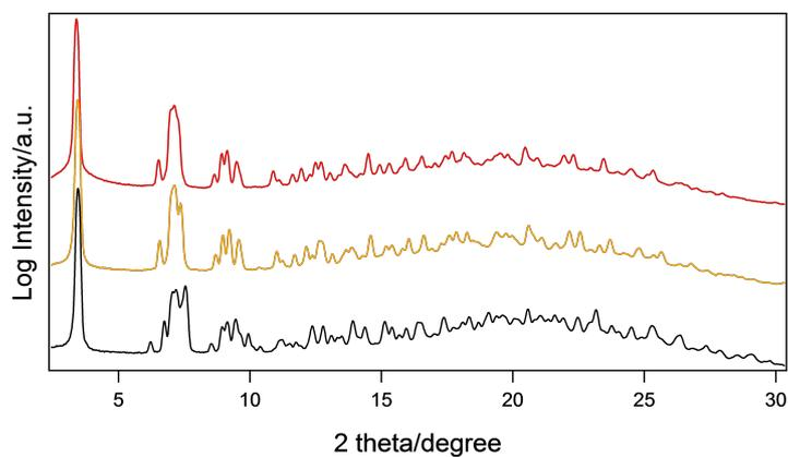
**Figure S43.** VT-XRD patterns of **3C8BF4** at 25 °C (black), 150 °C (orange), and 210 °C (red).
