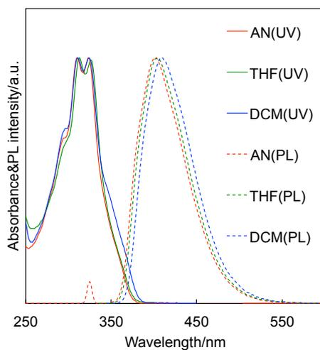
**Figure S49.** UV-vis and fluorescence spectra of **3C12BF4** in various solvents ( $10^{-5}$  M). AN: acetonitrile, THF: tetrahydrofuran, DCM: dichloromethane. The excitation wavelengths were that of the absorption maxima.
