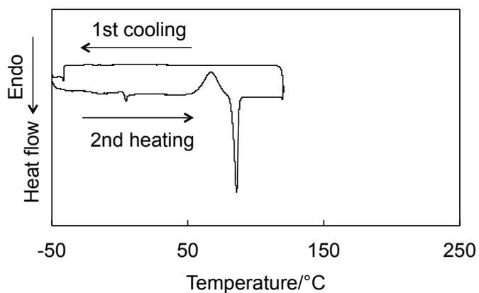
**Figure S34.** DSC thermogram of **3C12TFSI** in first cooling and second heating processes at 5 °C/min.
