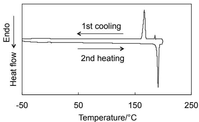
**Figure S33.** DSC thermogram of **2C12BF4** in first cooling and second heating processes at 5 °C/min.
