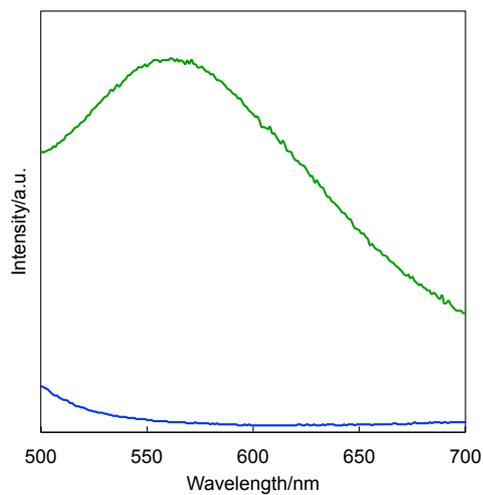
**Figure S51.** Fluorescence spectra of **3C12OTf** (blue line) and **3C16BF4** (green line) in solid state obtained by irradiating at 450 nm.
