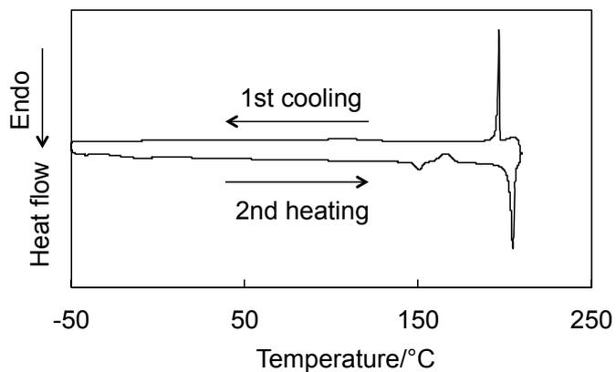
**Figure S32.** DSC thermogram of **3C8BF4** in first cooling and second heating processes at 5 °C/min.
