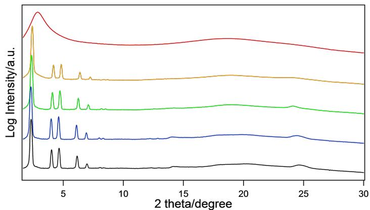
**Figure S40.** VT-XRD patterns of **3C12BF4** at 25 °C (black), 100 °C (blue), 140 °C (green), 180 °C (orange), and 220 °C (red).
