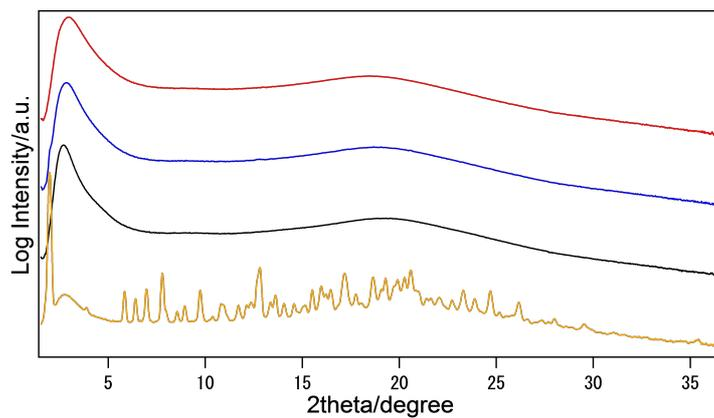
**Figure S45.** VT-XRD patterns of **3C12TFSI** at 25 °C (black), 75 °C (blue), and 120 °C (red). Orange line denotes a diffraction pattern of sample after standing at 75 °C for 1 h.
