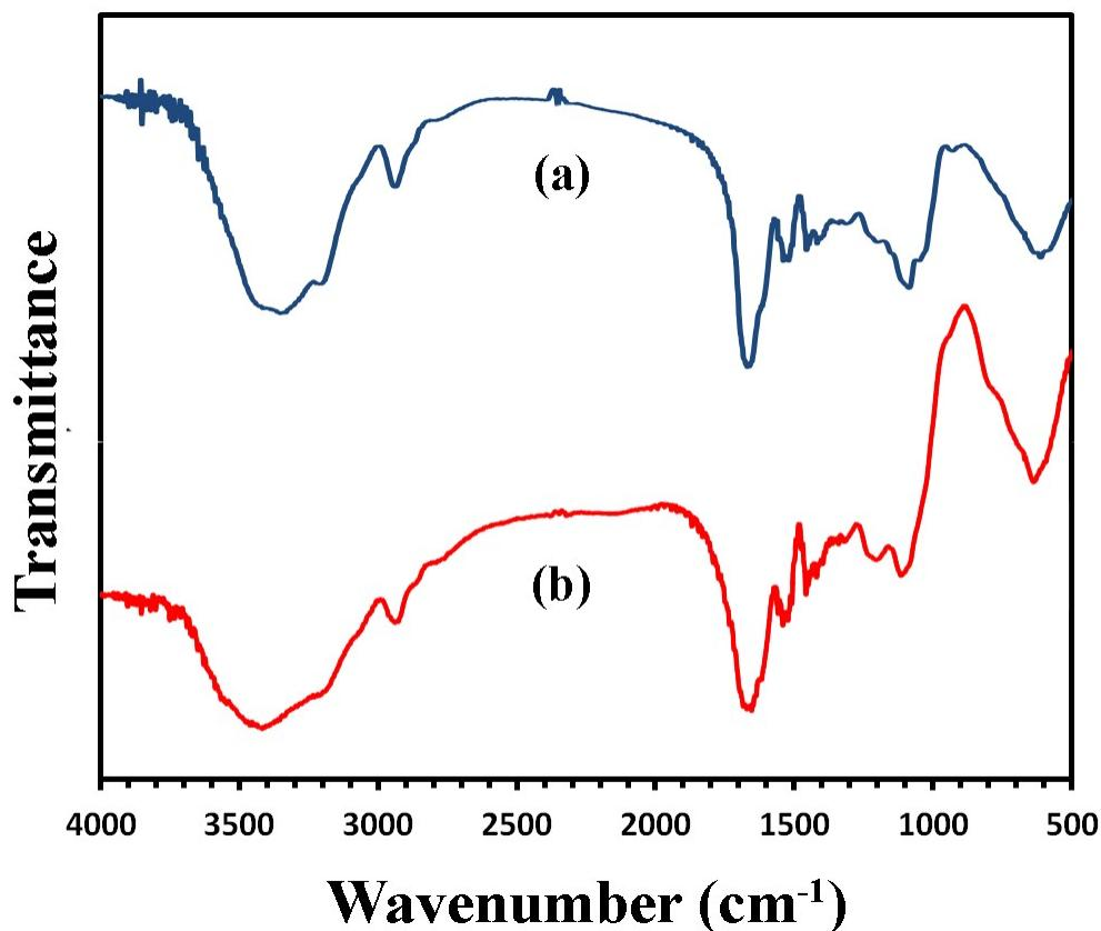
**Fig. S1** FT-IR spectra of fresh (a) and recycled (b) catalyst.
