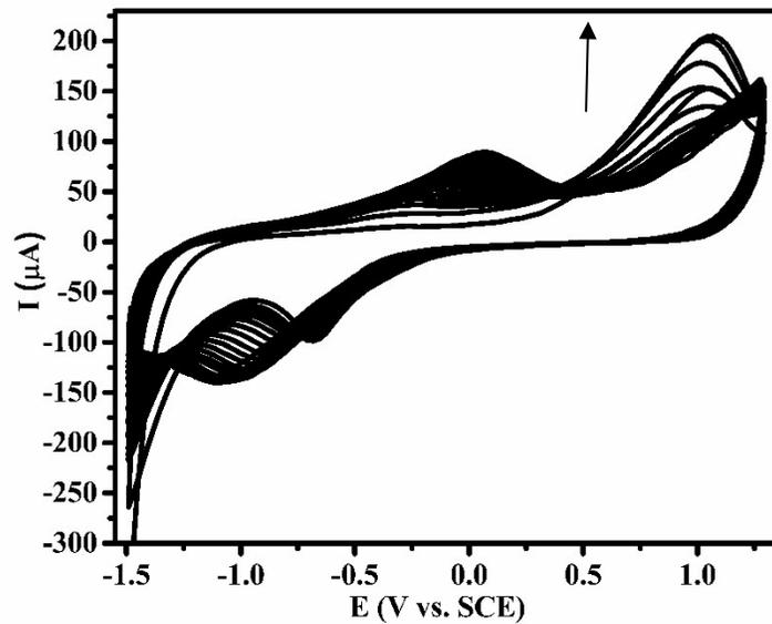
**Figure S2.** Electrochemical synthesis of ERG/PMB composite with 0.013 mM MB in pH 7.4 Buffer solution. Scan rate  $50 \text{ mV s}^{-1}$ .
