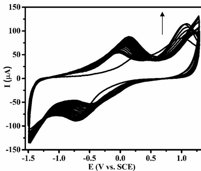
**Figure S1.** Electrochemical synthesis of ERG/PMB composite with 0.006 mM MB in pH 7.4 Buffer solution. Scan rate 50 mV s<sup>-1</sup>.
