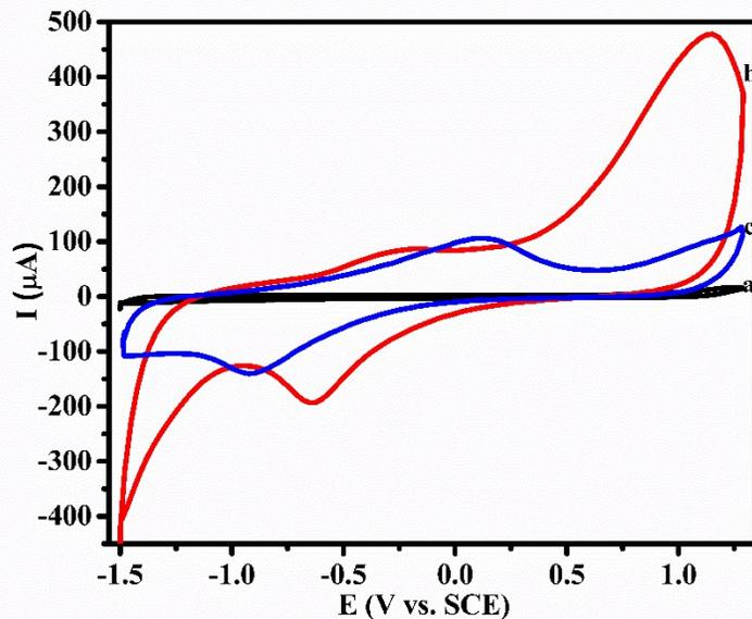
**Figure S6.** (a) GC, (b) GO and (c) ERG modified electrodes in pH 7.4 Buffer Solution. Scan rate 50  $\text{mV s}^{-1}$ .
