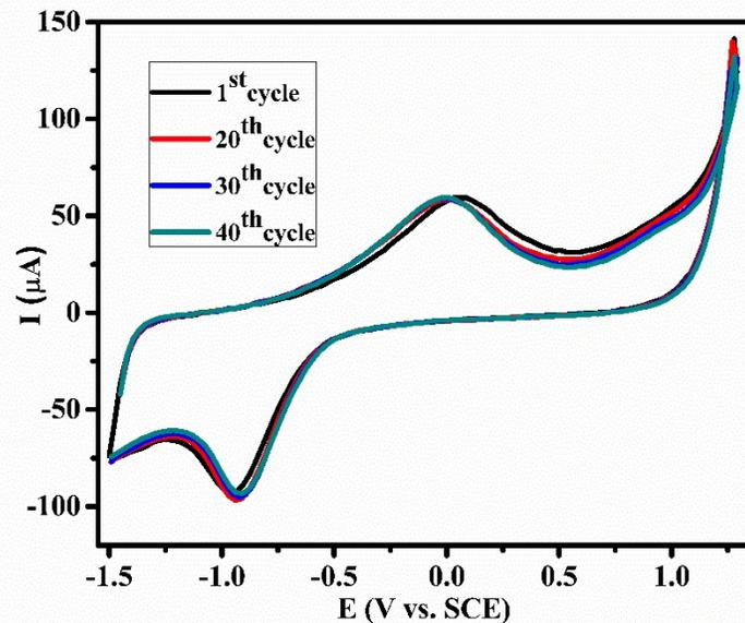
**Figure S8.** 1<sup>st</sup>, 20<sup>th</sup>, 30<sup>th</sup> and 40<sup>th</sup> cycles of ERG/PMB modified electrode in pH 7.4 buffer solution. Scan rate 50 mV s<sup>-1</sup>.
