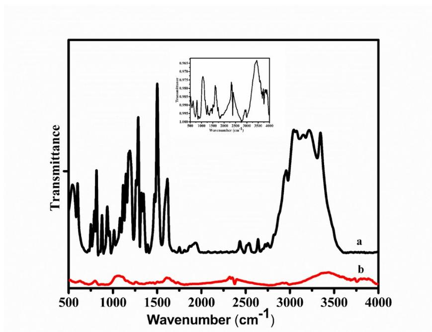
**Figure S14.** FT-IR Spectrum of (a) dopamine and (b) Oxidative Grafted dopamine on ERG/PMB modified electrode surface.
