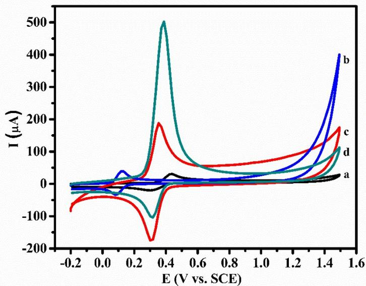
**Figure S11.** Cyclic Voltammograms of  $1 \times 10^{-3}$  mol L<sup>-1</sup> dopamine with (a) GC, (b) PMB, (c) ERG and (d) ERG/PMB modified electrodes in 0.1 M H<sub>2</sub>SO<sub>4</sub>. Scan rate 50 mV s<sup>-1</sup>.
