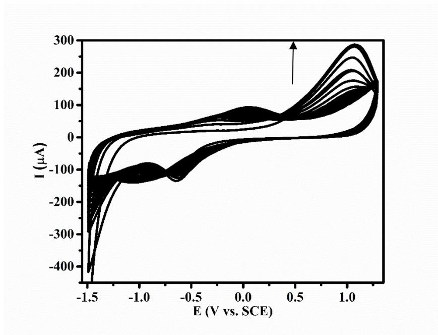
**Figure S3.** Electrochemical synthesis of ERG/PMB composite with 0.02 mM MB in pH 7.4 Buffer solution. Scan rate  $50 \text{ mV s}^{-1}$ .
