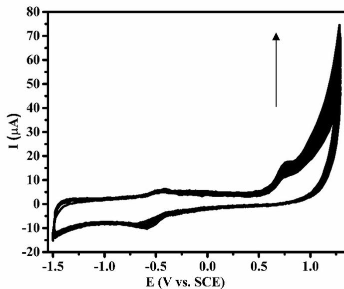
**Figure S4.** Electrochemical polymerization of Methylene Blue (MB) in pH 7.4 Buffer solution for 20 cycles. Scan rate  $50 \text{ mV s}^{-1}$ .
