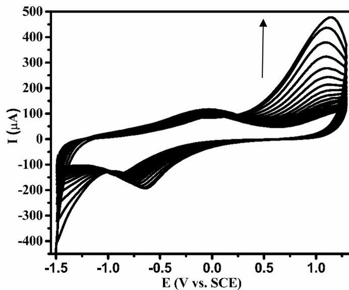
**Figure S5.** Electrochemical reduction of Graphene Oxide in pH 7.4 Buffer solution with continuous 20 cycles. Scan rate  $50 \text{ mV s}^{-1}$ .
