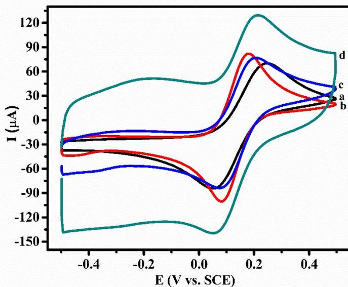
**Figure S9.** Cyclic Voltammograms of (a) GC, (b) PMB, (c) ERG and (d) ERG/PMB modified electrodes with 1 mM  $[\text{Fe}(\text{CN})_6]^{3-/4}$  in 0.1 M KCl. Scan rate 50 mV s<sup>-1</sup>.
