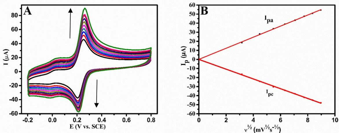
**Figure S13.** (A) Cyclic voltammogram of dopamine grafted ERG/PMB modified electrode after washing with Scan rates from 50, 80, 100, 120, 140, 160, 180, 200 and 250 mV s<sup>-1</sup> and (B) peak current vs square root of scan rate.
