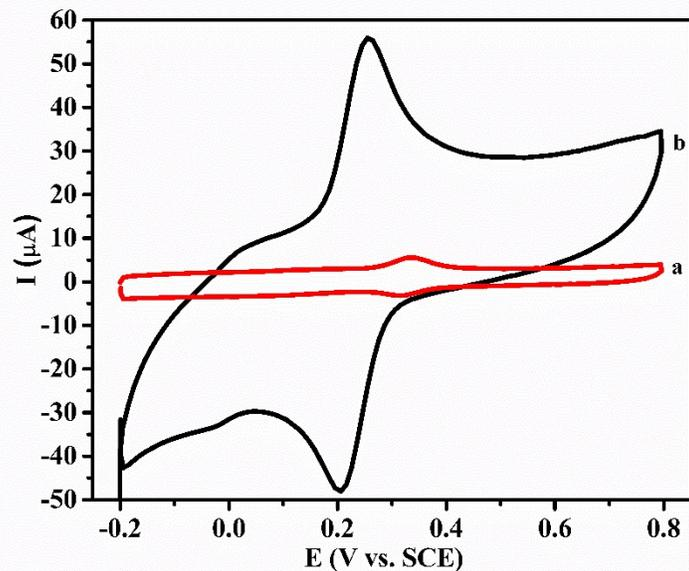
**Figure S12.** Cyclic Voltammograms of  $1 \times 10^{-3}$  mol L<sup>-1</sup> dopamine grafted (a) GC, (b) ERG/PMB modified electrodes in 0.1 M H<sub>2</sub>SO<sub>4</sub> after washing with water. Scan rate 50 mV s<sup>-1</sup>.
