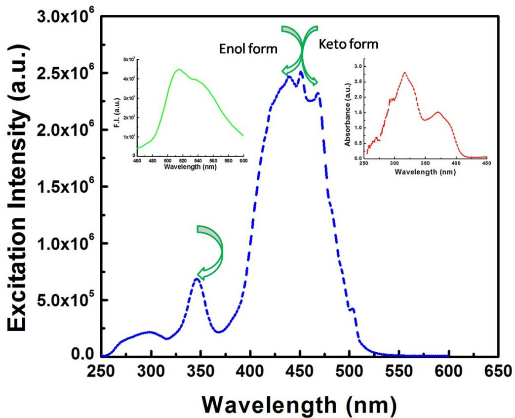
**Figure S11.**UV, Emission and Excitation plot of DFC-TS in non proton solution (DMSO).
