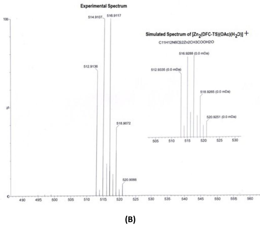
**Figure S9.** Mass spectrum of DFC-TS+Zn<sup>2+</sup>(1:2) in MeCN: (A) Full range spectrum and (B) simulated spectrum.
