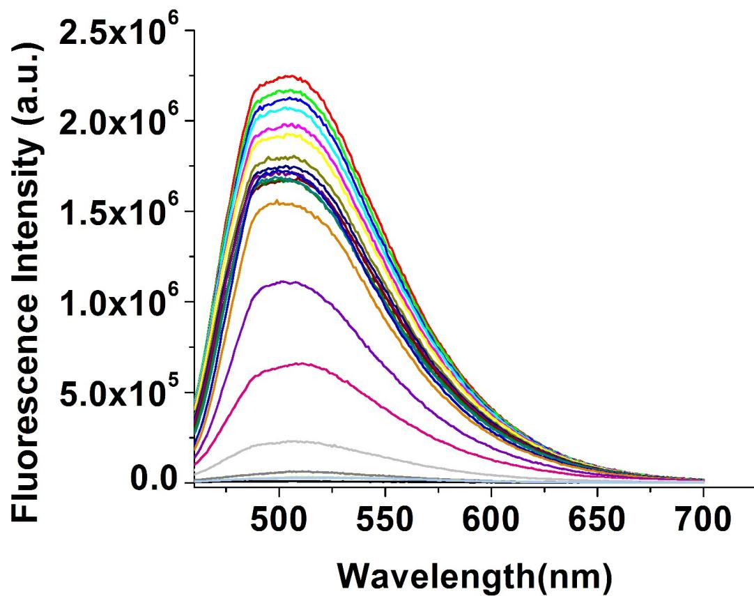
**Figure S14.** Competitive fluorescence titration plot for the displacement of Zn<sup>2+</sup> from Zn<sub>2</sub>(DFC-TS) ensemble (20  $\mu$ M with respect to DFC-TS) with Na<sub>2</sub>H<sub>2</sub>EDTA (0-50  $\mu$ M) in DMSO-H<sub>2</sub>O (9:1, v/v) at pH 7.2 (HEPES buffer).
