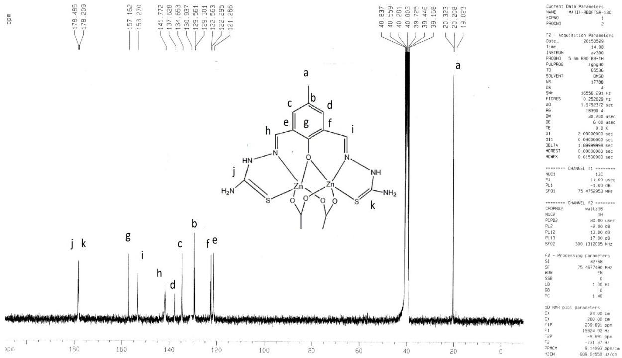
**Figure S5.**  $^{13}\text{C}$  NMR spectrum of DFC-TS +  $\text{Zn}^{2+}$ (1:2),in DMSO- $d_6$  in Bruker 300 MHz instrument.
