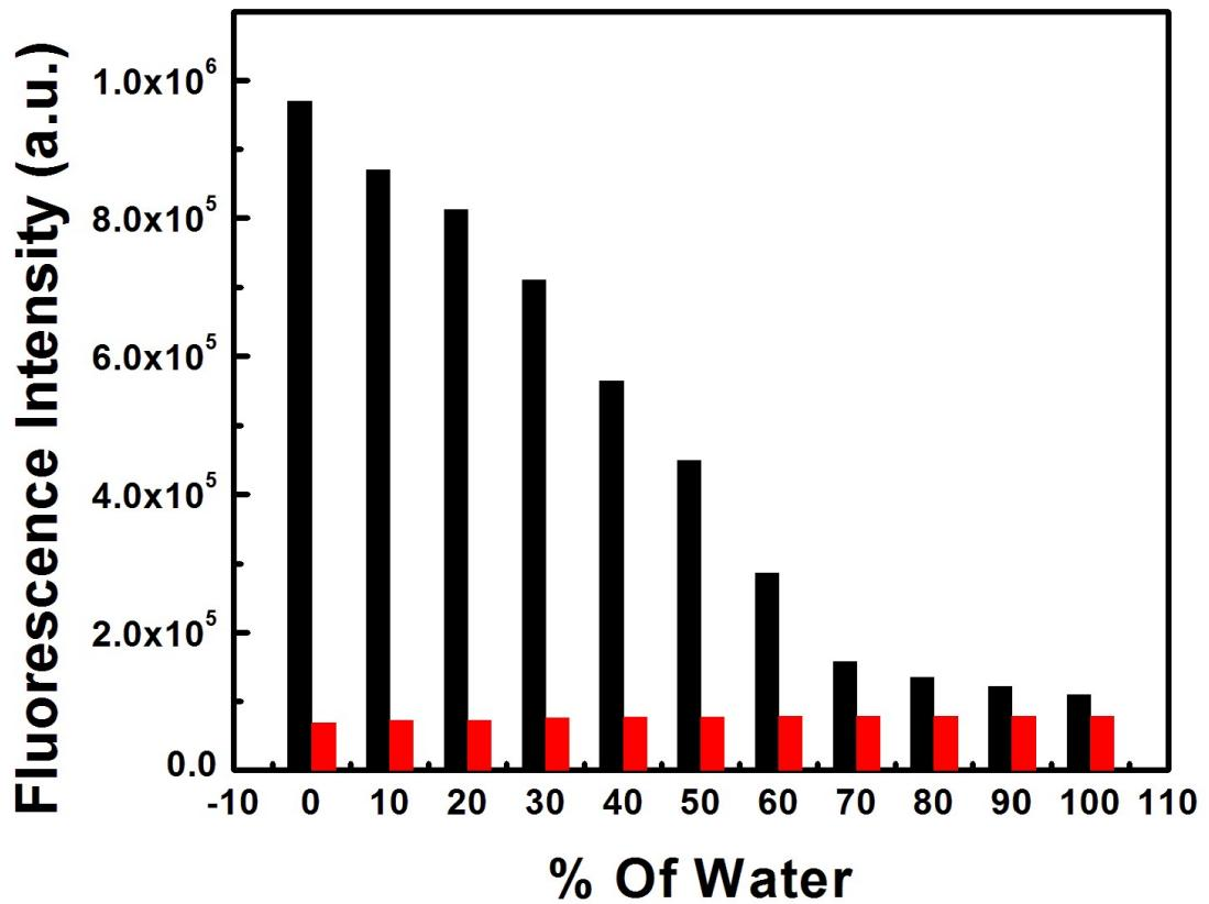
**Figure S13b** Fluorescence emission bar diagram of varying water,  $\lambda_{\text{ex}} = 390$  nm, red= DFC-TS and black= DFC-TS+ Zn<sup>2+</sup>.
