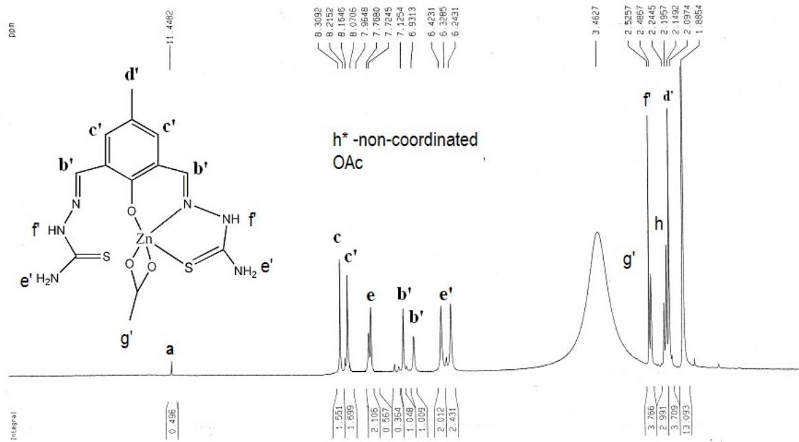
**Figure S2.**  $^1\text{H}$  NMR spectrum of DFCTS+  $\text{Zn}^{2+}$ (1:1), in  $\text{DMSO-d}_6$  in Bruker 300 MHz instrument.
