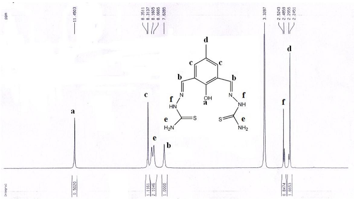
**Figure S1.**  $^1\text{H}$  NMR spectrum of DFC-TS, in  $\text{DMSO-d}_6$  in Bruker 300 MHz instrument.
