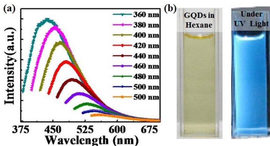
**Fig. S5** (a) The PL spectra of amine-GQDs at 340-480 nm excitation wavelengths. The photographs of the hexane dispersion of GQDs suspension: (b) without and (c) with illumination of UV light ( $\lambda = 336$  nm).
