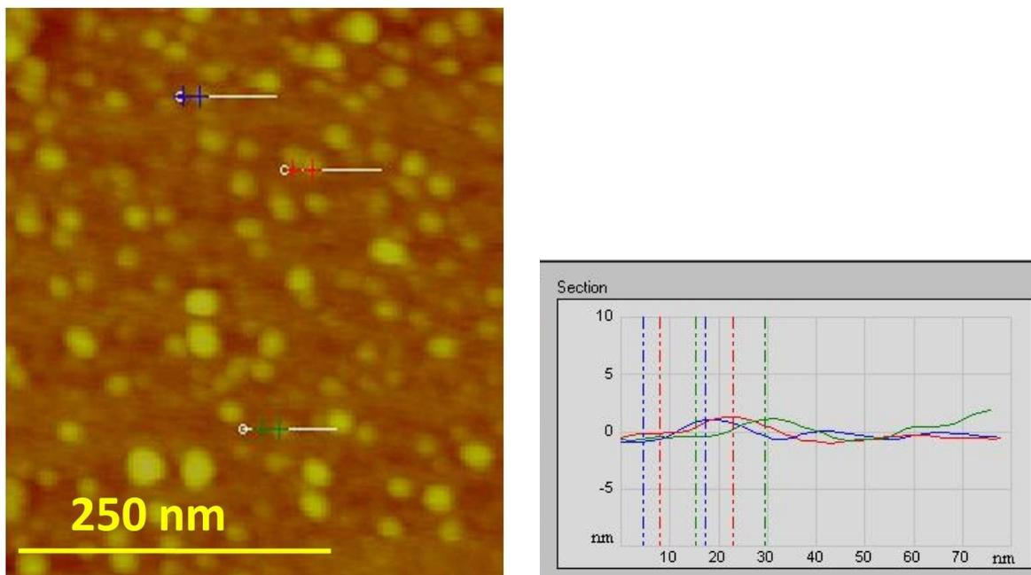
**Fig. S6** AFM images of 4 nm sized GQDs and (b) the corresponding cross-sectional analysis showing the average height of the GQDs to be 1-2 nm.
