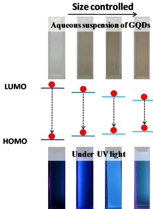
**Fig. S2** Shows the optical image of the GQDs along with the change in luminescence from blue to cyan under the UV light illumination ( $\lambda = 336$  nm) with the increase in size under the scheme of band gap change with size.
