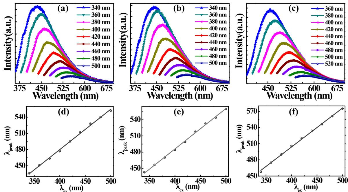
**Fig. S4** Excitation dependence PL spectra of GQDs of size: (a) 2 nm (b) 5.2 nm (c) 6.5 nm. Respective linear relationship between the emission wavelength  $\lambda_{\text{em}}$  and excitation wavelength,  $\lambda_{\text{exc}}$  of the GQD of size (d) 2 nm, (e) 5.2 nm and (f) 6.5 nm.
