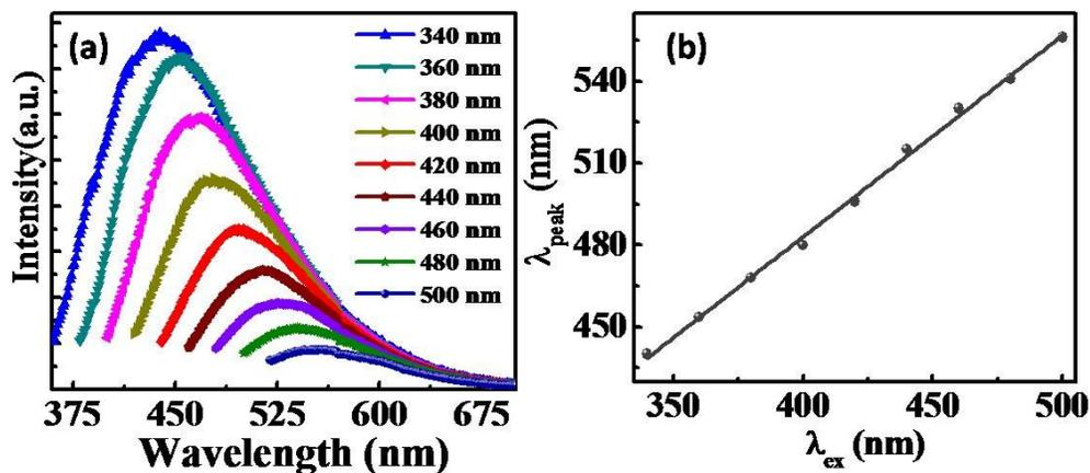
**Fig. S3** (a) Excitation dependence PL spectra of GQDs of size 4 nm and (b) Respective linear relationship between the emission wavelength  $\lambda_{\text{em}}$  and excitation wavelength,  $\lambda_{\text{exc}}$  of the GQD.
