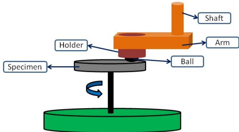
Fig. S2 The sketch of the ball-on-disk friction test apparatus
