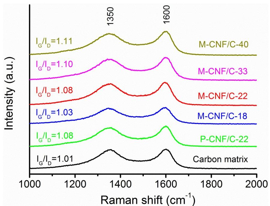
Fig. S4 Raman spectra of carbon matrix, P-CNF/C and M-CNF/C composites
