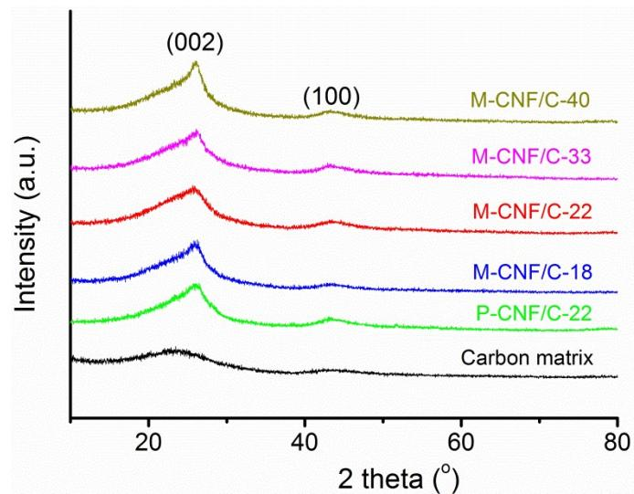
Fig. S3 XRD patterns of carbon matrix, P-CNF/C and M-CNF/C composites
