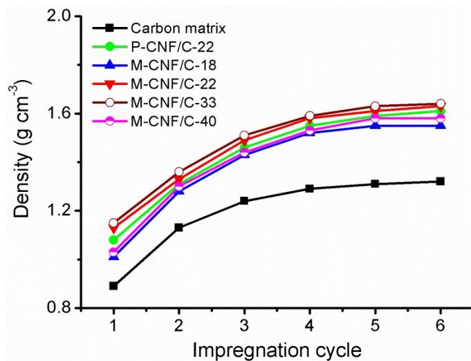
Fig. S1 Variation of density of carbon matrix, P-CNF/C and M-CNF/C composites with respect to impregnation cycle
