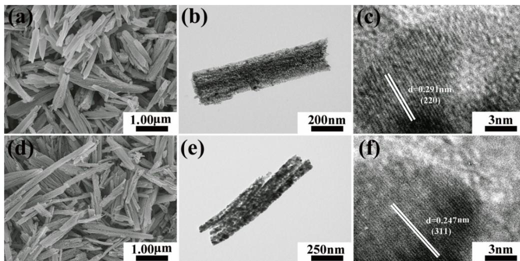
**Figure S6.** SEM images of MCO-1 (a) and MCO-2 (d). TEM and HRTEM images of MCO-1 (b and c) and MCO-2 (e and f).
