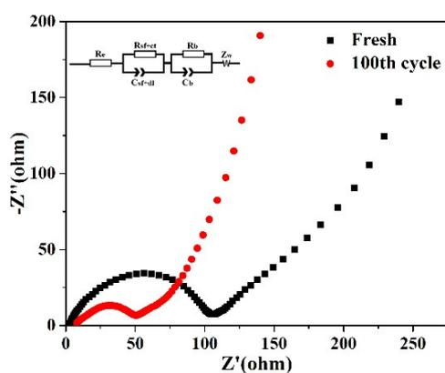
**Figure S5.** Nyquist plots of porous  $\text{MnCo}_2\text{O}_4$  nanorods before discharging and after
