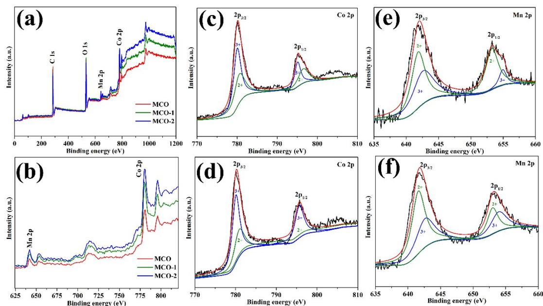
**Figure S7.** XPS spectra: (a) survey spectrum of three samples. (b) Magnification of survey spectrum in (a). (c) and (e) are Co 2p and Mn 2p for MCO-1. (d) and (f) are Co 2p and Mn 2p for MCO-2.
