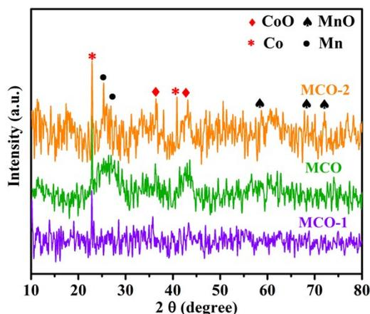
**Figure S9.** XRD pattern of MCO, MCO-1 and MCO-2 after discharge/charge.
