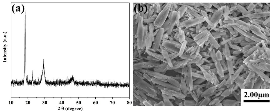
**Figure S1.** (a) XRD pattern of the precursor. (b) SEM image of as-prepared precursor.
