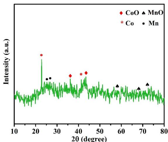
**Figure S3.** XRD pattern of MCO after discharge/charge.
