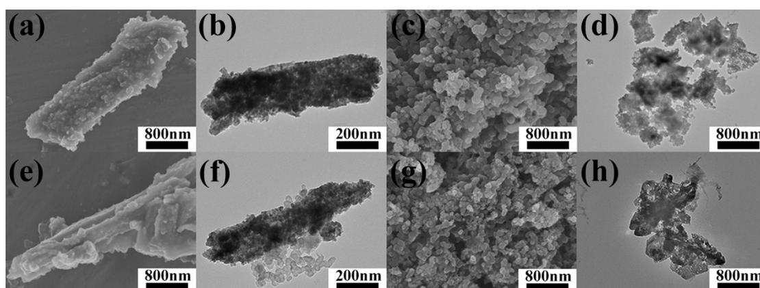
**Figure S4.** SEM and TEM images of MCO before and after discharge/charge with various binders. (a) and (b) are SEM and TEM images before cycle with CMC/SBR binder. (c) and (d) are SEM and TEM images after test with CMC/SBR binder. (e) and (f) are SEM and TEM images before cycle with PVDF binder. (g) and (h) are SEM and TEM images after cycles with PVDF binder.
