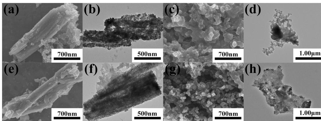
**Figure S10.** The SEM and TEM images of samples MCO-1 and MCO-2 before and after test. (a) and (b) are the SEM and TEM images of sample MCO-1 before the discharge/charge process. (c) and (d) are the SEM and TEM images of MCO-1 after the discharge/charge process. (e) and (f) are the SEM and TEM images of sample MCO-2 before the discharge/charge process (g) and (h) are the SEM and TEM images of sample MCO-2 after the discharge/charge process.
