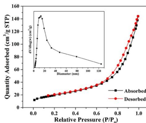
**Figure S2.** Nitrogen adsorption–desorption isotherm and the corresponding pore size distribution (inset) of the as-prepared  $\text{MnCo}_2\text{O}_4$  nanorods.
