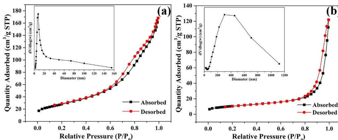
**Figure S8.** Nitrogen adsorption–desorption isotherm and the corresponding pore size distribution (insert) of MCO-1 (a) and MCO-2 (b).
