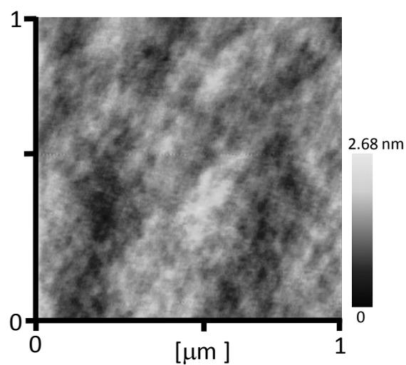
**Fig. S1.** AFM topographic image of the Chi alone prepared by casting Chi solution on **0w**-film in an observation area of  $1 \times 1 \mu\text{m}^2$ , which exhibits the  $R_{\text{rms}}$  value of  $0.86 \pm 0.11 \text{ nm}$ .
