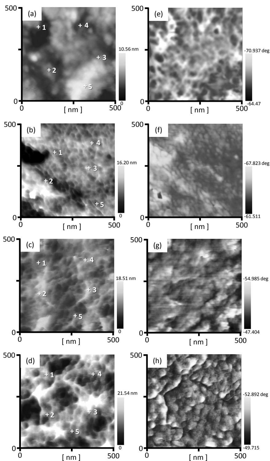
**Fig. S2.** AFM (a-d) topographic and (e-h) phase-shift images of the (a, e) **0w**- (b, f) **1w**- (c, g) **5w**- and (d, h) **10w**-films in an observation area of 500 x 500 nm<sup>2</sup>, and the marks numbered with 1–5 were the measured pints for the force curves in Fig. 3 in the manuscript.
