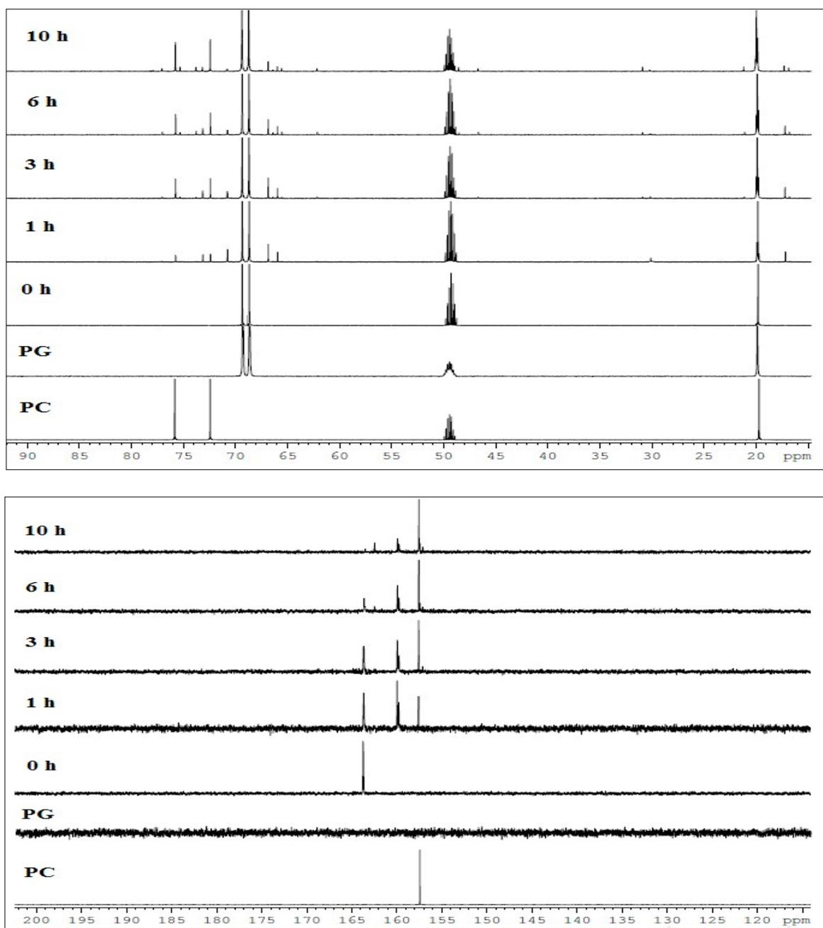
**Fig. S3:**  $^{13}\text{C}$  NMR Overlay of Time Online Analysis of Propylene Carbonate Synthesis using Propylene Glycol and Urea.
