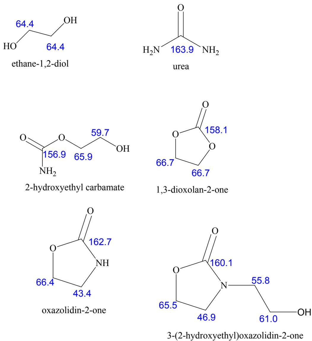
**Fig. S2:** <sup>13</sup>C NMR of Reactants, Intermediate and Products Labelled in ppm for Ethylene Carbonate Synthesis.
