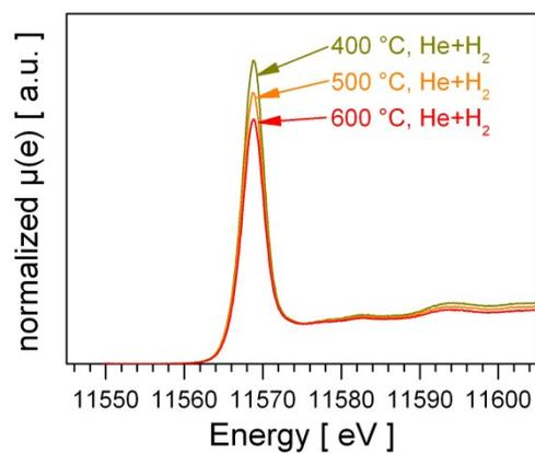
ESI 3 - TPR-XANES spectra recorded from Pt:SnO<sub>2</sub> GI sensor in 2 % vol. H<sub>2</sub> in He at 400, 500 and 600 °C. The raw data was taken from reference 25 of the main manuscript and treated in the same way as the data shown in in figure 4.
