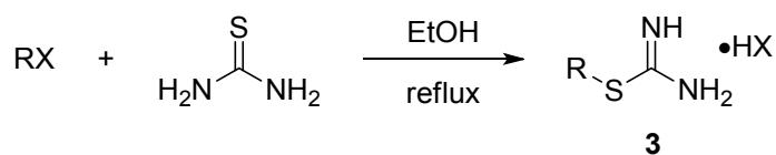
To the solution of thiourea (3.806 g, 50 mmol) in EtOH (50 mL) was added alkyl halide (55 mmol). The mixture was kept refluxing in oil bath. The completion of the reaction was monitored by TLC. The solvent was removed and the residue was recrystallized from EtOH/EtOAc.
