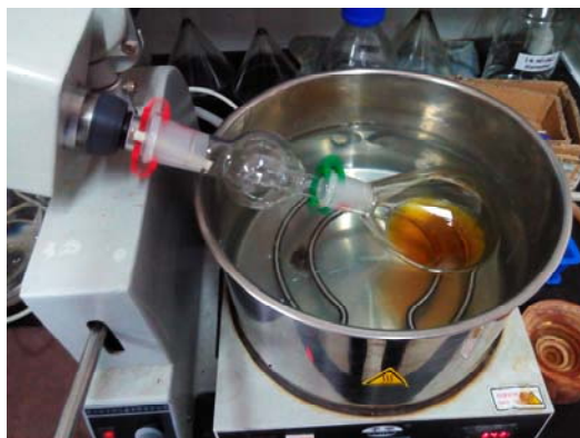
Fig. S4. Left: The organic layer was concentrated under reduced pressure after extraction (EA/H 2 O). Right: The crude product was dissolved by CH 2 Cl 2 .
