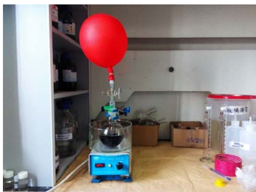
Fig. S2. Left: The reaction was stirred at r.t. under argon atmosphere. Right: The reaction was monitored by TLC (PE/EA = 2/1).
