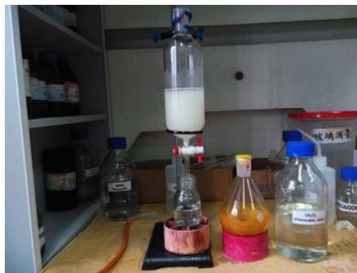
Fig. S4. Left: The organic layer was concentrated under reduced pressure after extraction (EA/H 2 O). Right: The crude product was dissolved by CH 2 Cl 2 .
