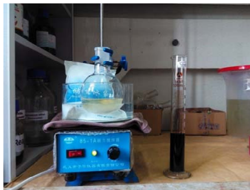
Fig. S1. Left: Materials and reagents. Right: To a solution of mifepristone (2.5 g) and LiOAc (1.92 g) in 90 mL THF was added I 2 /MeOH (46 mL) at 0 °C.
