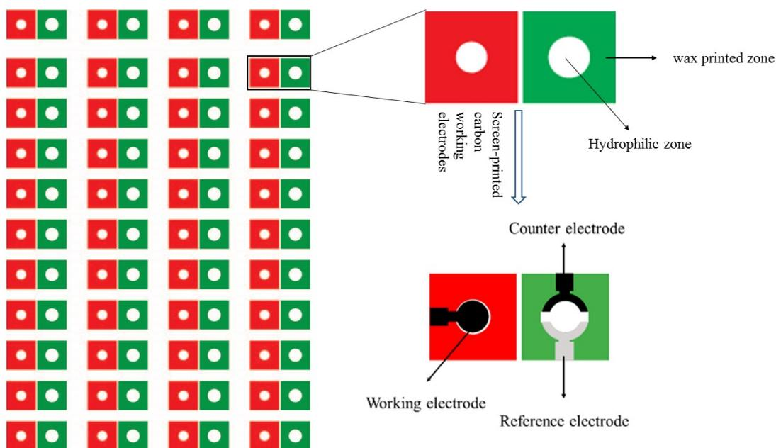
**Fig.S1.** Paper sheets were firstly patterned in bulk using a wax printer. The schematic representation and shape of this  $\mu$ -PAD with the screen-printed reference and counter electrode, and the working electrode on the other side.
