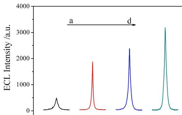
**Fig. S5.** ECL curves (a) neither CdTe@AuPd composites nor Au-PWE, (b) Au-PWE, but only CdTe/Ab<sub>2</sub> is used as the ECL tag, (c) with AuPd but not Au-PWE, (d) both CdTe@AuPd composites and Au-PWE
