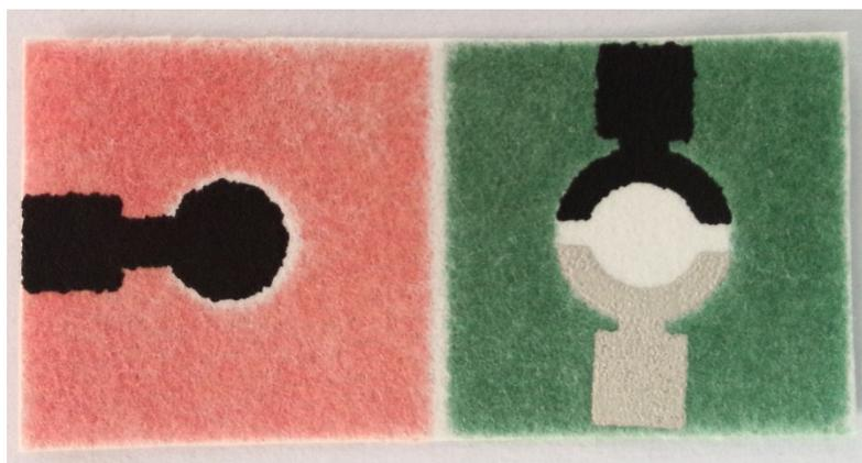
**Fig.S4.** After screen-printing of electrode, including working electrode, one counter electrode, and one Ag/AgCl reference electrode.
