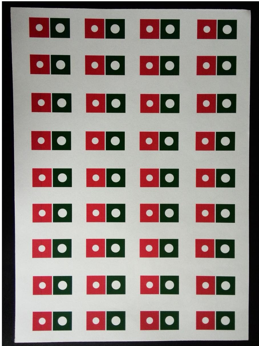
**Fig.S2.** Wax-patterns of this paper device on a paper sheet (A4) before baking
