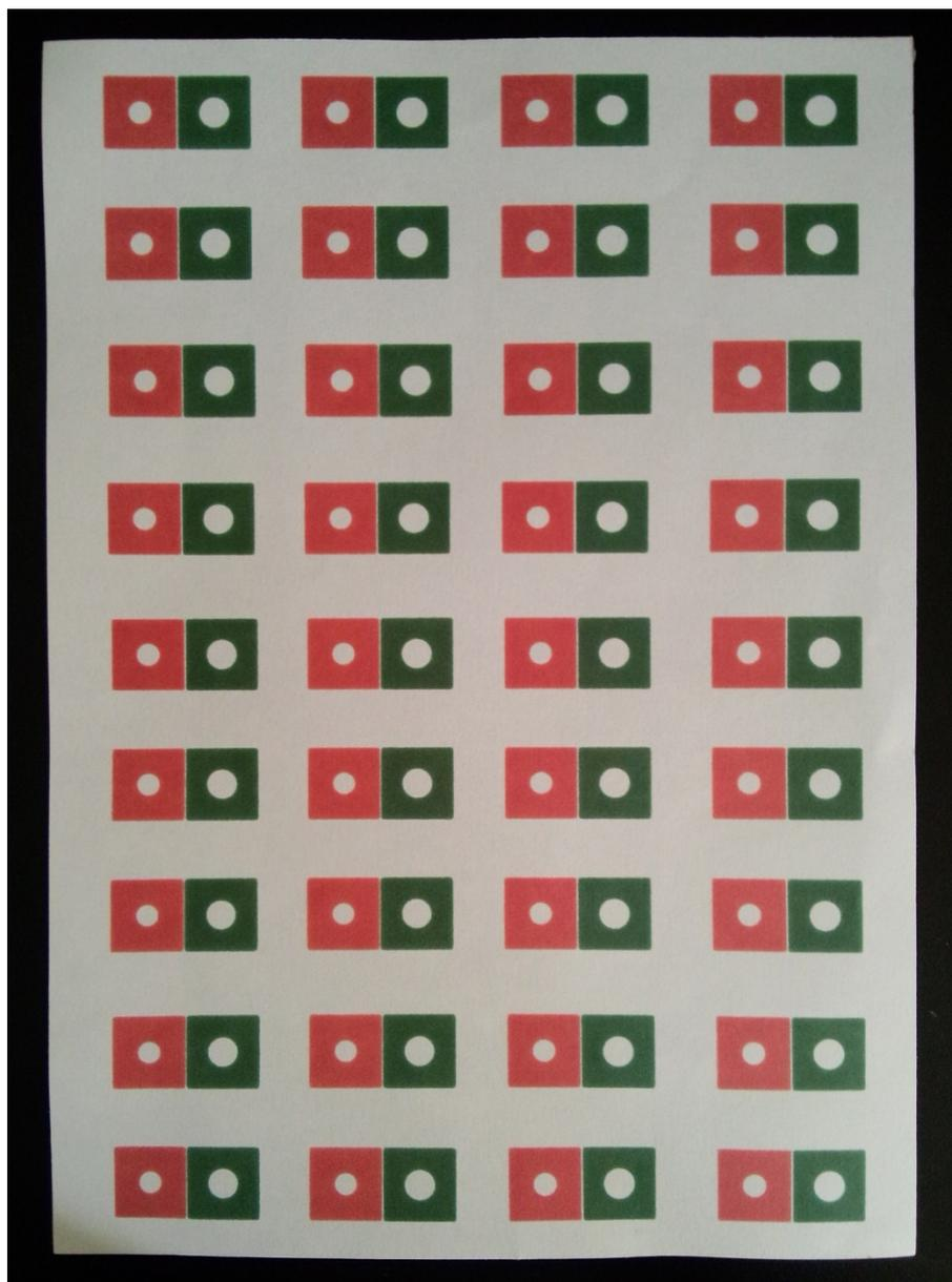
**Fig.S3.** Wax-patterns of this paper device on a paper sheet (A4) after baking.
