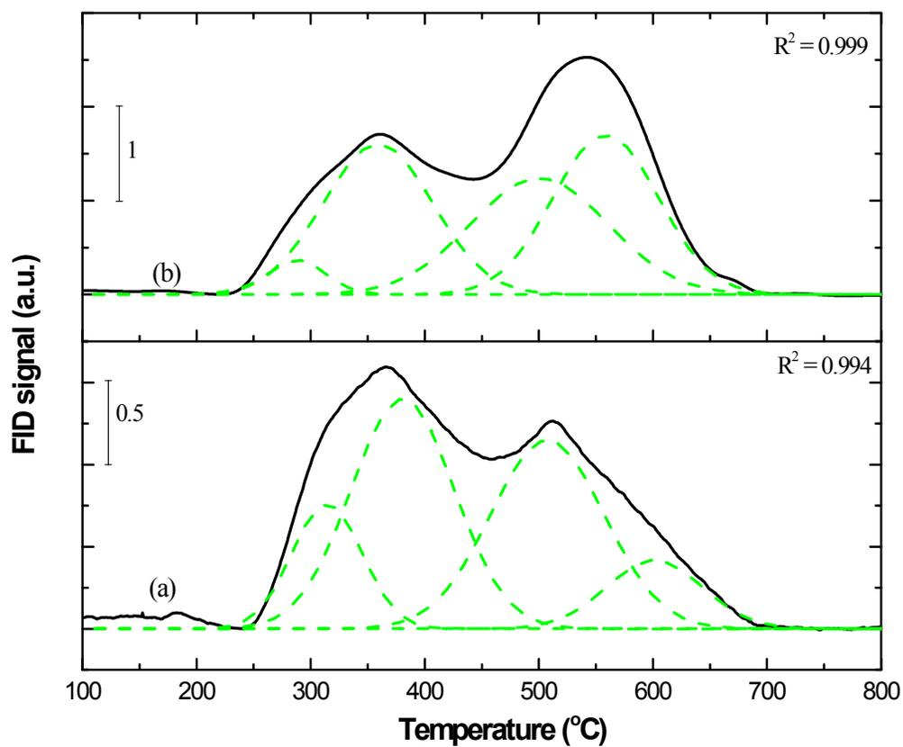
**Figure S5** TPSR profiles for 0.7K/10Fe/SiO<sub>2</sub> and 0.7K/10Fe/SiO<sub>2</sub>-MW catalysts. Microwave pretreatment conditions: 10 s, 450 W.
