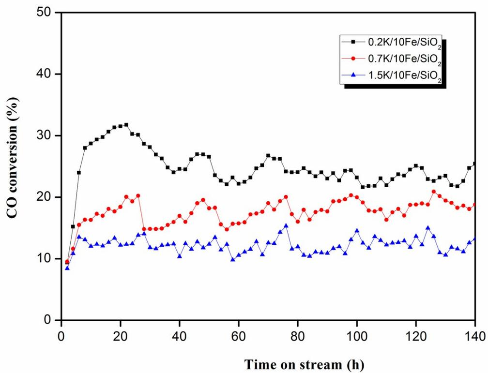
**Figure S9** CO conversions for the 0.2K/10Fe/SiO<sub>2</sub>, 0.7K/10Fe/SiO<sub>2</sub> and 1.5K/10Fe/SiO<sub>2</sub> catalysts that were not microwaved.
