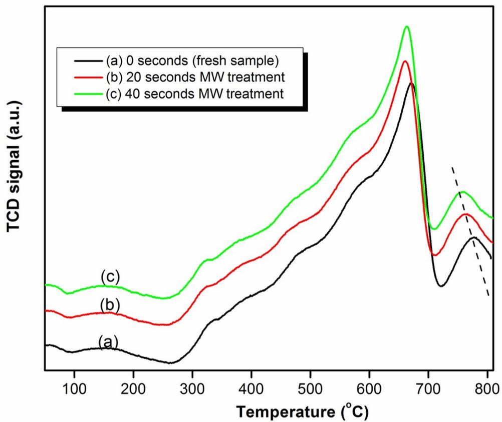
**Figure S8** TPR profiles for a 1.0K/10Fe/SiO<sub>2</sub> catalyst that was microwave pretreated for various periods.
