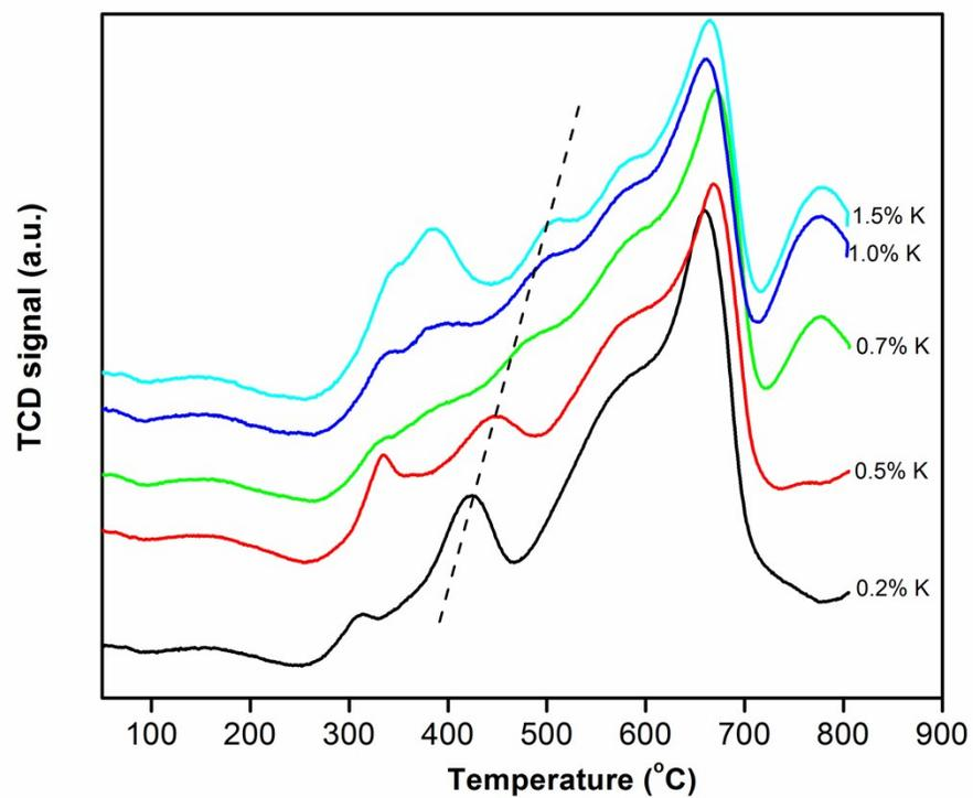
**Figure S1** H<sub>2</sub>-TPR profiles for the catalysts of the composition xK/10Fe/SiO<sub>2</sub>, where x varies from 0 to 1.5 wt%.
