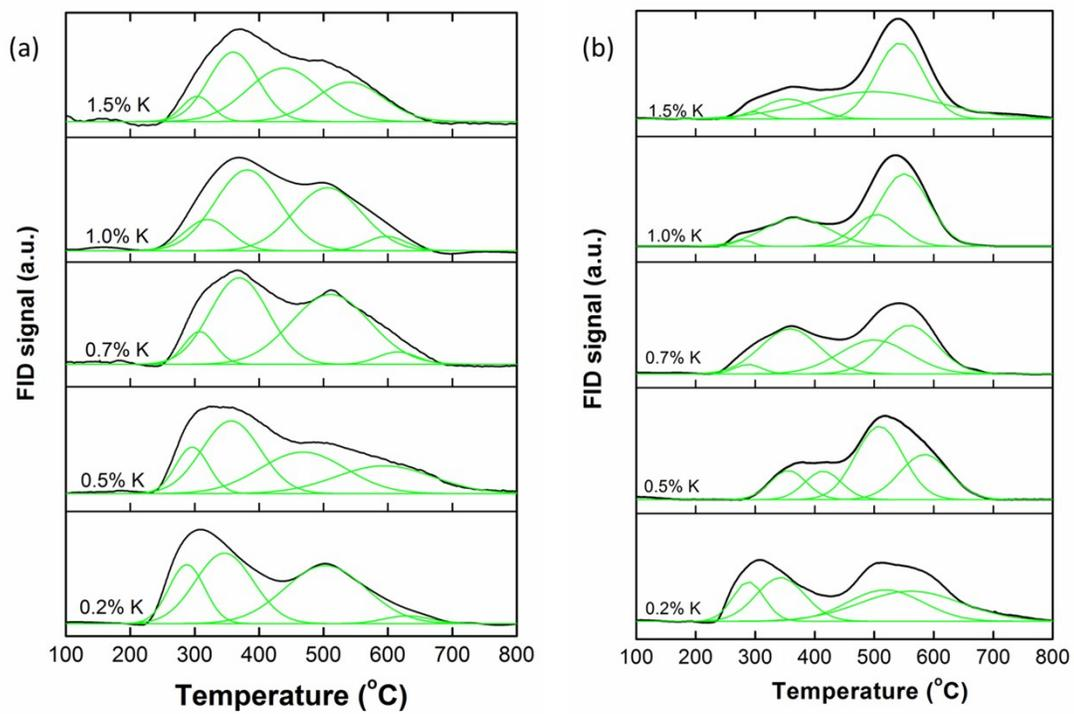
**Figure S3** TPSR profiles of (a)  $x\text{K}/10\text{Fe}/\text{SiO}_2$ -type and (b)  $x\text{K}/10\text{Fe}/\text{SiO}_2$ -MW catalysts,  $x$  varies from 0.2 to 1.5 wt%.
