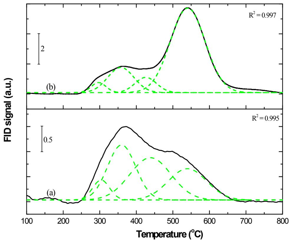
**Figure S7** TPSR profiles of the 1.5 K/10 Fe/SiO<sub>2</sub> catalyst (a) before and (b) after microwave treatment.
