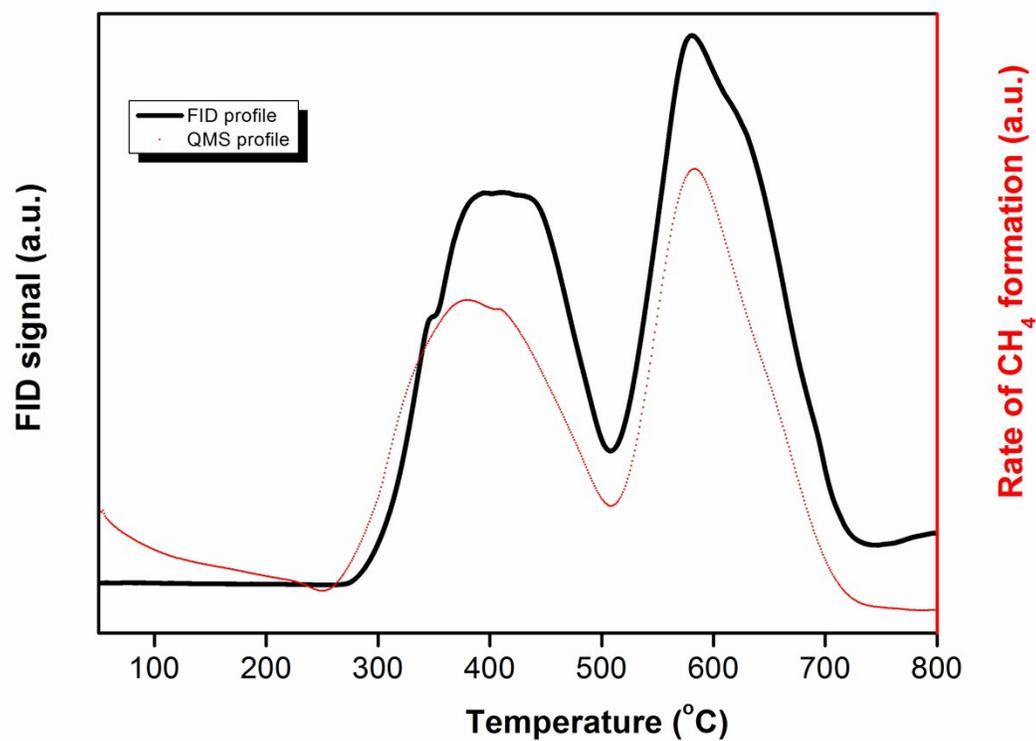
**Figure S2** A comparison of typical TPSR profiles obtained from an FID (—) and by QMS (···) performed simultaneously when using the 0.2K/10Fe/SiO<sub>2</sub> catalyst.
