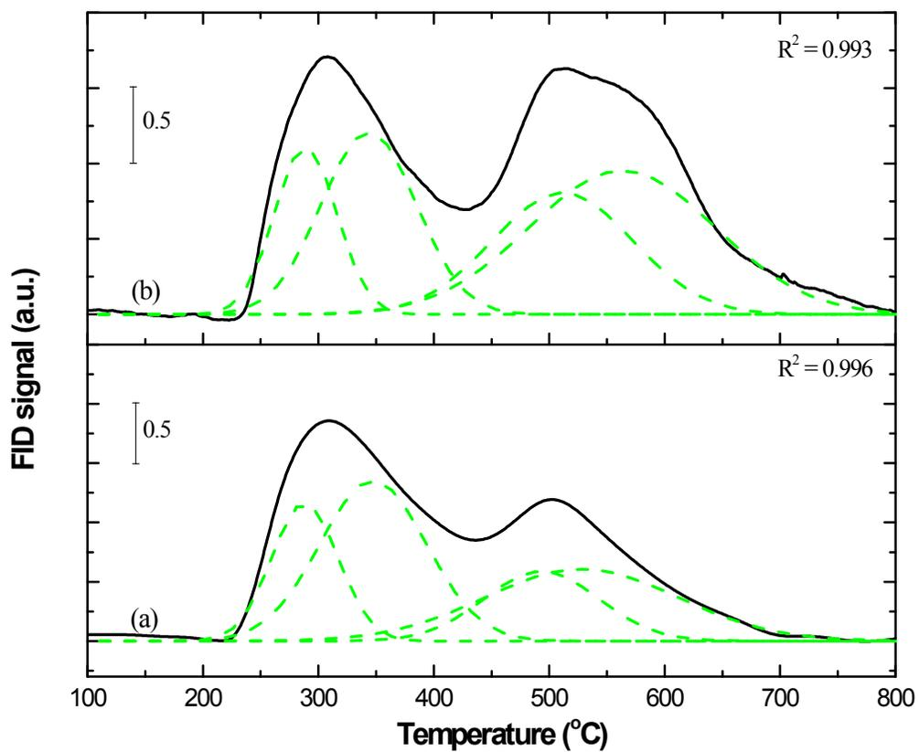
**Figure S4** TPSR profiles of (a) 0.2K/10Fe/SiO<sub>2</sub> and (b) 0.2K/10Fe/SiO<sub>2</sub>-MW catalysts. Pretreatment conditions: 10 s, 450 W.
