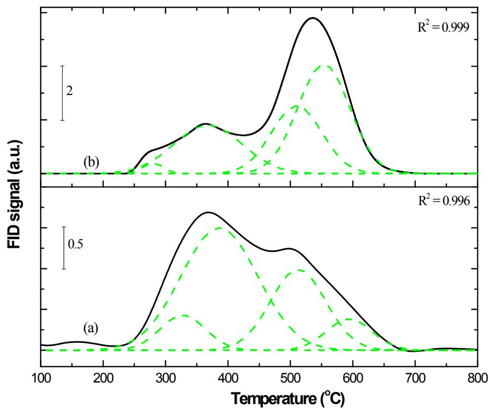
**Figure S6** TPSR profiles of 1.0K/10Fe/SiO<sub>2</sub> catalyst (a) before and (b) after microwave (MW) pretreatment. Pretreatment conditions: 10 s, 450 W.
