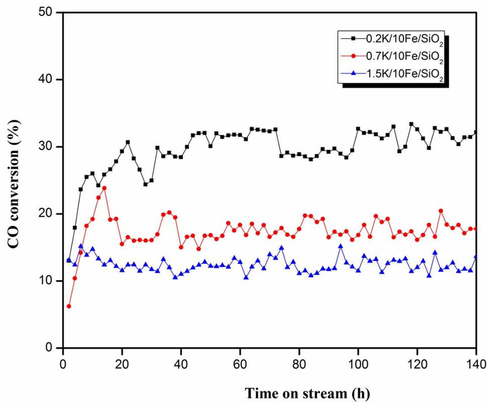
**Figure S10** CO conversions for the various microwave pretreated catalysts. Pretreatment conditions: 450 W, 10 s.
