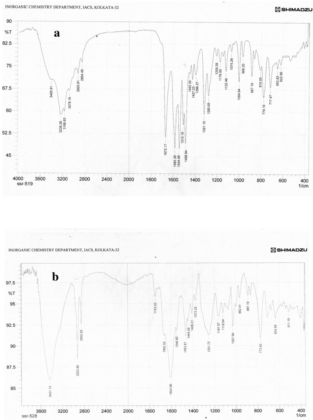
**Figure S1:** IR spectra of a) BPPTP and b) Cu xerogel of BPPTP.
