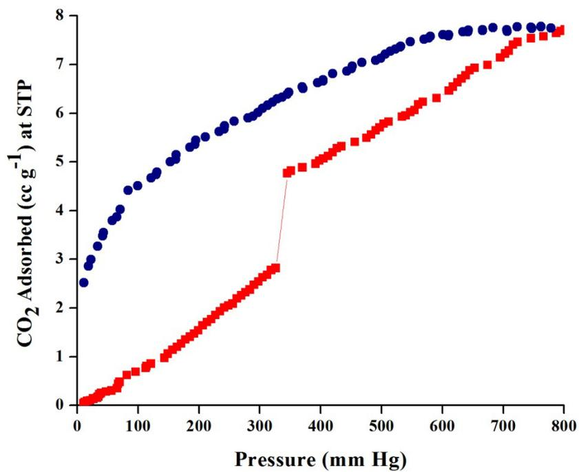
Figure S3: CO<sub>2</sub> adsorption-desorption isotherm of copper triflate xerogel.
