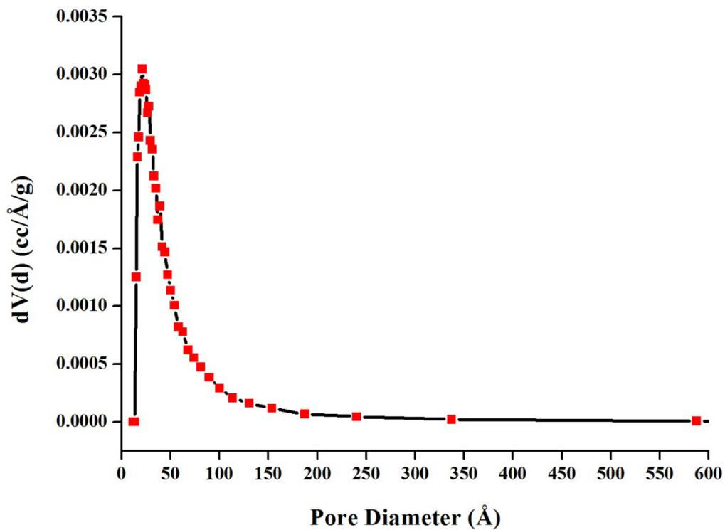
Figure S2: BJH pore distribution for copper triflate xerogel.
