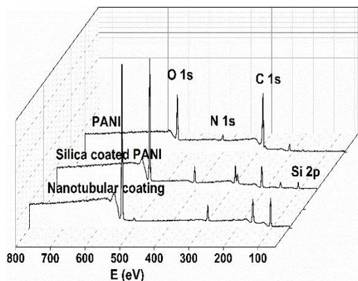
**Figure S1.** X-ray photoelectron spectra of PANI coating, silica coated PANI coating and nanotubular coating.
