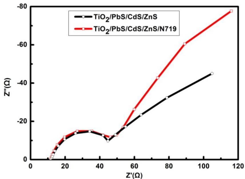
**Figure S1.** Typical electrochemical impedance spectra of cells in the forms of Nyquist plots. The spectra were measured with an external potential of -0.7V in the dark.
