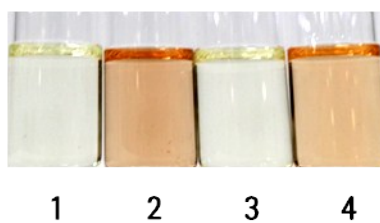
Figure S26. (a) Absorption spectra and (b) color changes of 1 , 1-S 2- , 1-S 2- + Al 3+ and 1-S 2- + Al 3+ + S 2- in a mixture of bis-tris buffer/DMSO (1:9, v/v). Conditions: 1 = 10 \mu M, S 2- 88 equiv, and Al 3+ 30 equiv.
