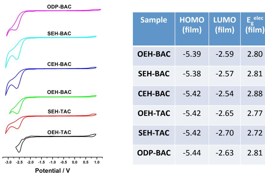
Figure S1. Left: Cyclic voltammetry of **BACs** and **TACs** (Scan rate: 100 mV/s). Right: HOMO, LUMO and Electrical gaps determined by CV.
