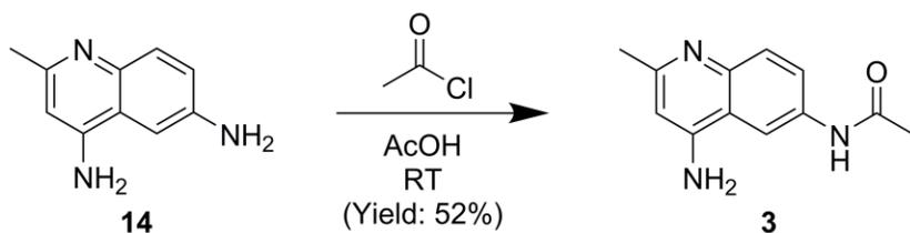
**6-Acetamido-4-aminoquinoline (Acetyl-hemisurfen) (3).** 4,6-diamino-2-methylquinoline (**14**) (40 mg, 0.23 mmol) was dissolved in glacial acetic acid (0.5 ml) under argon. Acetyl
