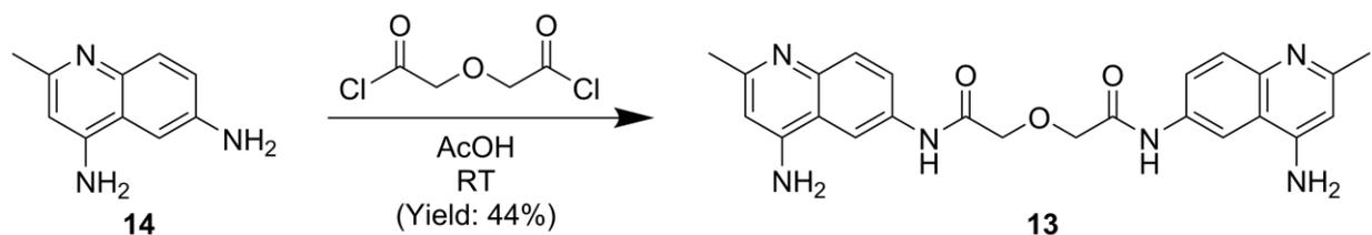
**2,2'-oxybis(N-(4-amino-2-methylquinolin-6-yl)acetamide) (Diglycolyl Surfen) (13).** 4-6-diamino-2-methyl-quinoline (**14**) (40 mg, 0.23 mmol) was dissolved in glacial acetic acid (0.3 ml) under argon. Diglycolyl chloride (13.7  $\mu$ l, 0.12 mmol) was slowly added to this solution. A heavy precipitate formed, and the mixture was stirred for 1 hour at room temperature. After
