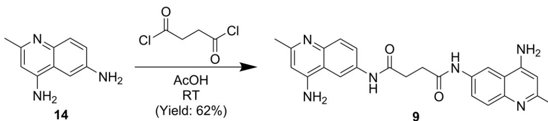
**N,N'-bis(4-amino-2-methyl-6-quinolyl)-butanediamide (Succinyl Surfen) (9).** 4-6-diamino-2-methyl-quinoline (**14**) (100 mg, 0.58 mmol) was dissolved in glacial acetic acid (0.6 ml) under argon. Succinyl chloride (32  $\mu$ l, 0.29 mmol) was slowly added to this solution. A heavy precipitate formed, and the mixture was stirred for 2 hours at room temperature. After addition of diethyl ether (5 ml), the solid was filtered, washed with diethyl ether and dried under high
