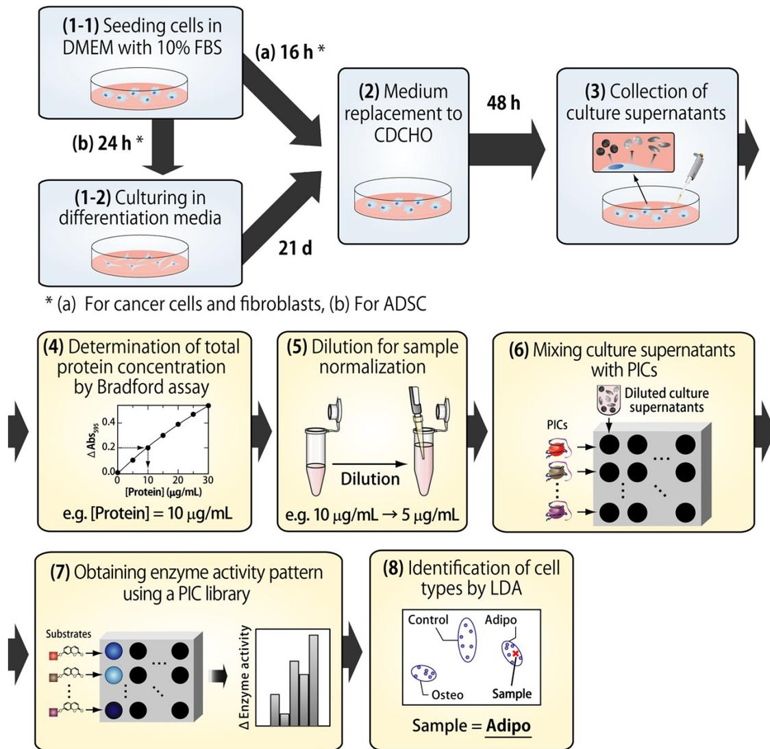
**Figure S3.** Schematic representation for the sensing procedure of the culture supernatants using a PIC sensor array.
