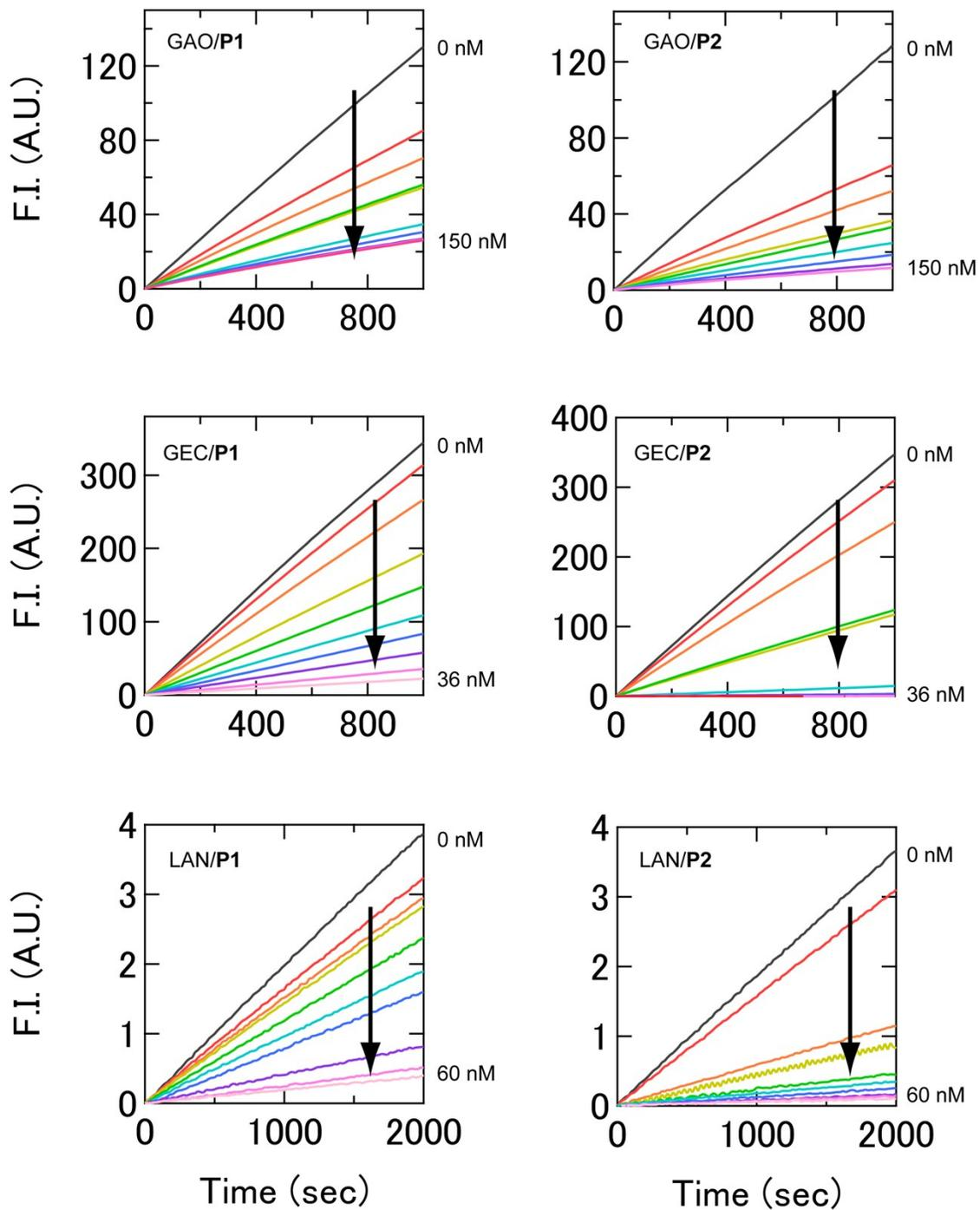
**Figure S1.** Time courses of increase in fluorescence intensity in the presence of various concentrations of PEGylated polyamines. Titration of PEGylated polyamines to 0.5 nM GAO, 0.2 nM GEC, and 10 nM LAN in 10 mM MOPS (pH 7.0) with 5% chemically defined serum-free CDCHO medium.
