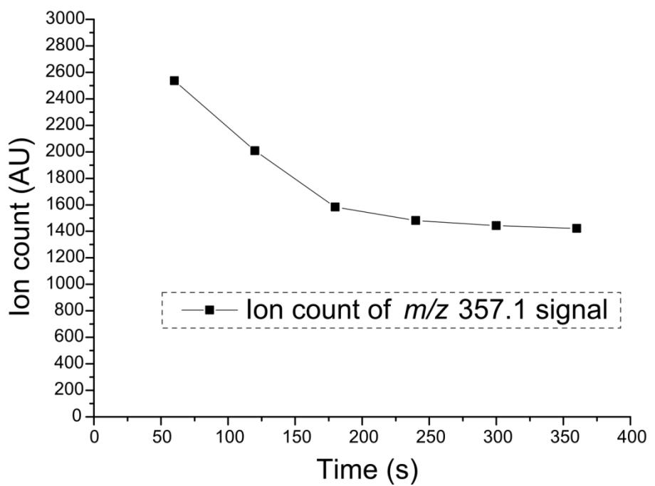
**Fig. S32** Ion counts of the ESI-MS signal at  $m/z$  357.1 assigned to  $[\text{Fe}^{\text{IV}}(\text{L1})(\text{O})(\text{OH})]^+$  at different reaction times for the reaction of **1** (1.5 mM) with CAN (7.5 mM) in 0.1 M  $\text{HNO}_3$  at room temperature.
