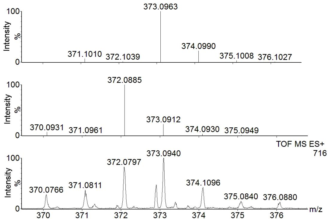
**Fig. S20** Electrospray ionization mass measurement of species at  $m/z$  373.0940 in reaction of **1** with NaIO<sub>4</sub> (800 equiv) in 0.1 M HNO<sub>3</sub>. Upper: Simulated isotopic pattern for  $[\text{Fe}^{\text{III}}(\text{L1})(\text{OO}^\bullet)(\text{OH})]^+$ . Middle: Simulated isotopic pattern for  $[\text{Fe}^{\text{IV}}(\text{L1})(\text{OO}^\bullet)(\text{O})]^+$ . Bottom: Experimental isotopic pattern.
