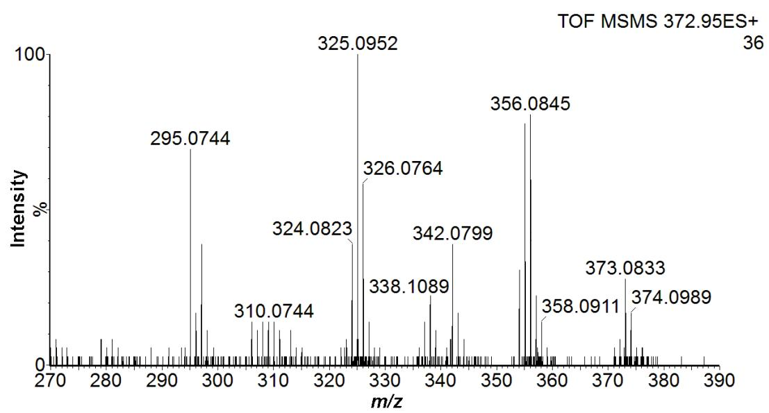
**Fig. S22** Collision-induced dissociation of the ion with  $m/z \sim 373.1$  (for the reaction of **1** with NaIO<sub>4</sub> in 0.1 M HNO<sub>3</sub>) recorded at the collision energy of 15 eV.
