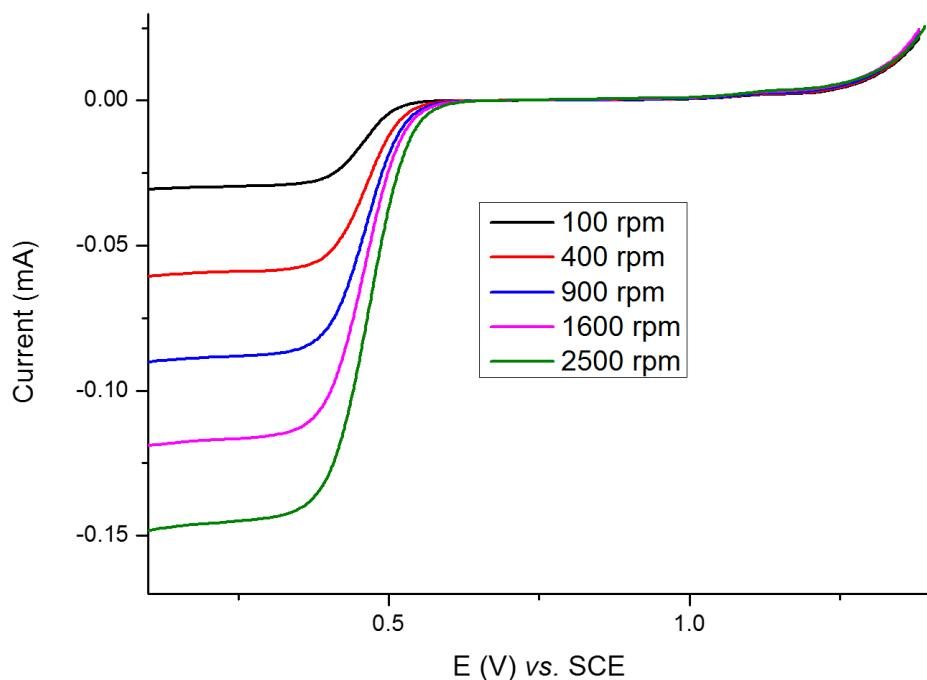
**Fig. S30** Linear scan voltammogram of **1**·ClO<sub>4</sub> in 0.1 M HNO<sub>3</sub> (pH 1) at various rotation rates. Working electrode: rotating glassy carbon disk; rotation rate: 100 to 2500 rpm (as denoted in the voltammogram); scan rate: 5 mV/s.
