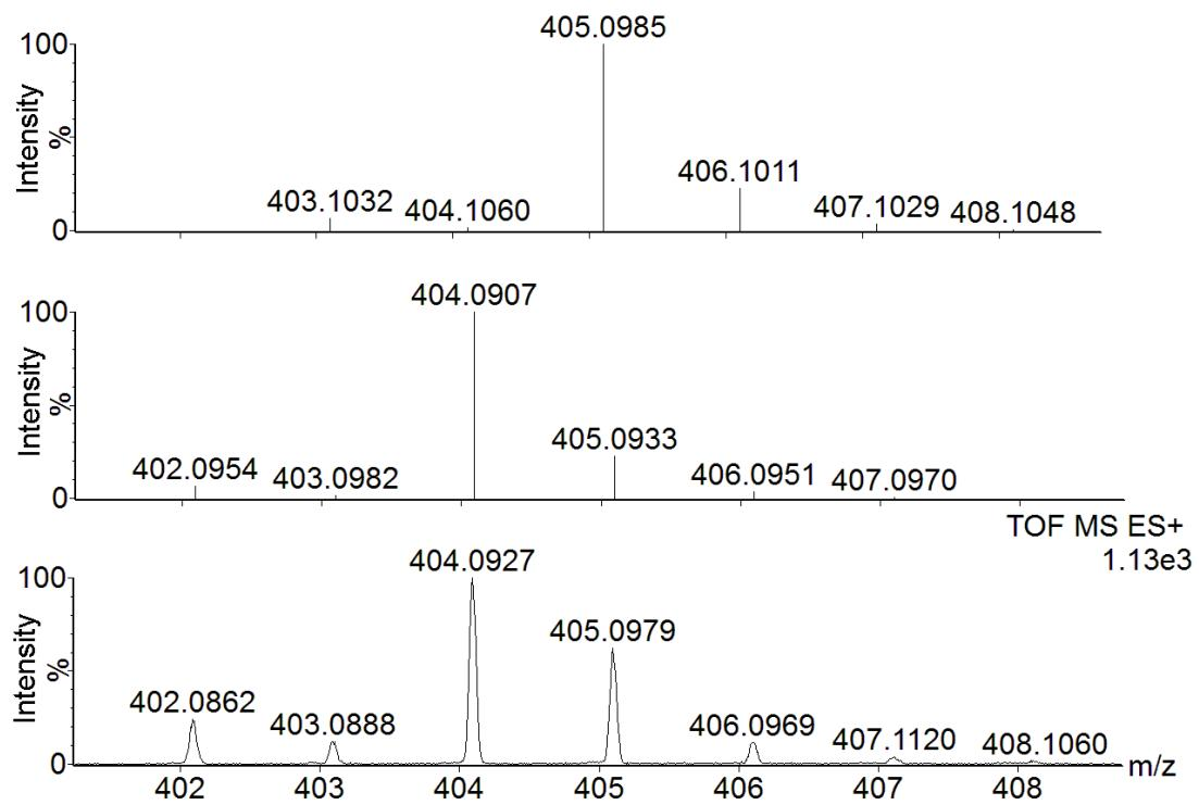
**Fig. S19** ESI-MS measurement of species at  $m/z$  404.0927 in reaction of **1** with CAN (200 equiv) in  $\text{H}_2^{18}\text{O}$ . Upper: Simulated isotopic pattern for  $[\text{Fe}^{\text{III}}(\text{L1})(^{18}\text{OH})(\text{N}^{16}\text{O}_3)]^+$ . Middle: Simulated isotopic pattern for  $[\text{Fe}^{\text{IV}}(\text{L1})(^{18}\text{O})(\text{N}^{16}\text{O}_3)]^+$ . Bottom: Experimental isotopic pattern.
