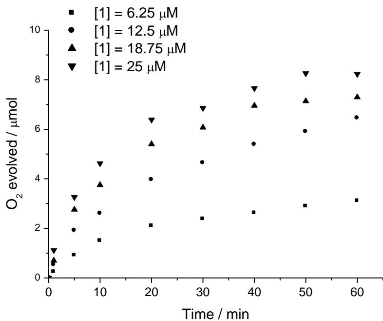
**Fig. S2** Plot of  $O_2$  evolution in **1**-catalysed water oxidation with CAN in 0.1 M  $HNO_3$  with time for different concentrations of **1**. Concentration of CAN: 125 mM.
