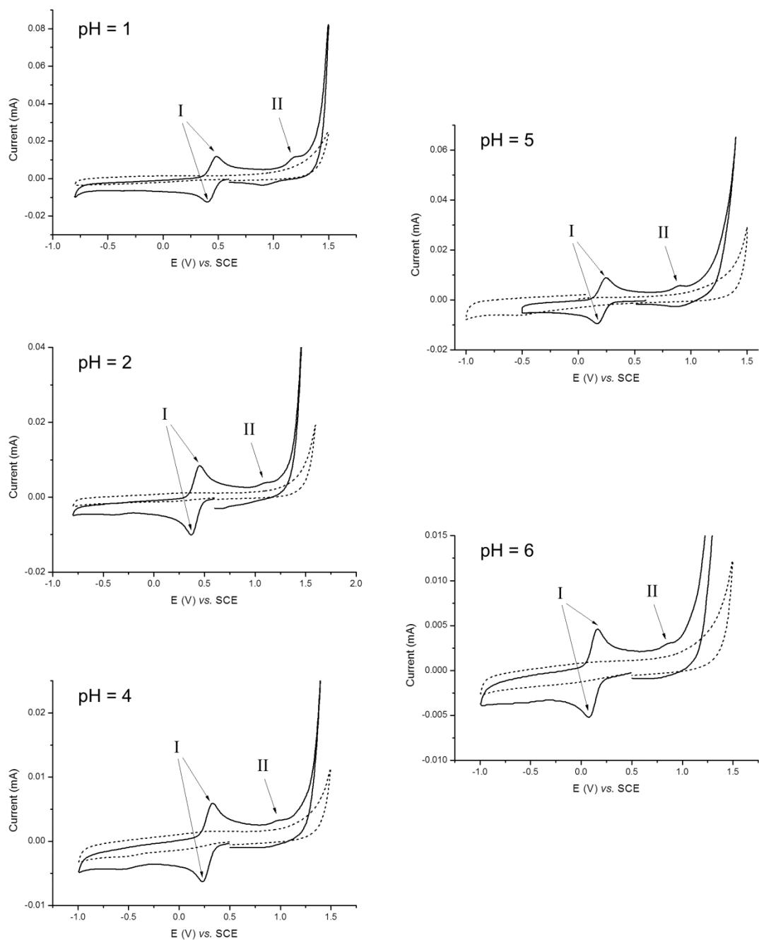
**Fig. S27** Solid lines: cyclic voltammograms of **1**· $\text{ClO}_4$  in 0.1 M  $\text{HNO}_3$  at pH 1, in 0.1 M  $\text{CF}_3\text{SO}_3\text{H}/\text{CF}_3\text{SO}_3\text{Li}$  at pH 2, and in 0.1 M acetate buffer at pH 4–6. Dotted lines: cyclic voltammograms of the acid/buffer background.
