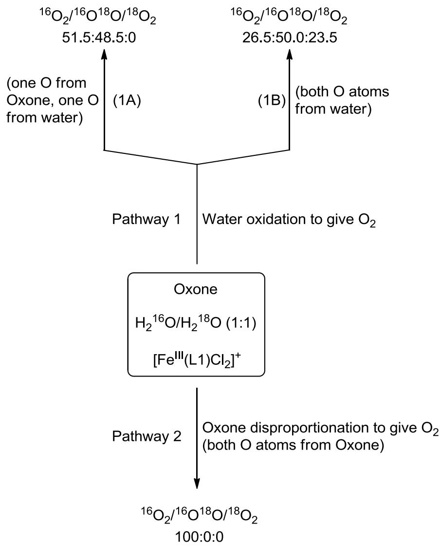
**Scheme S1** Possible pathways for  $O_2$  evolution in the reaction mixture of **1** with Oxone in  $H_2^{16}O/H_2^{18}O$  (1:1,  $H_2^{18}O$  used had 97 atom%  $^{18}O$ ). The calculated  $^{16}O_2/^{16}O^{18}O/^{18}O_2$  ratios for these pathways are shown.
