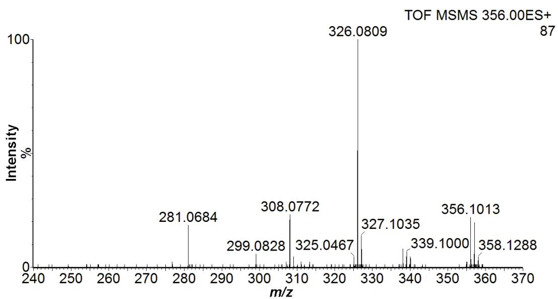
**Fig. S21** Collision-induced dissociation of the ion with  $m/z \sim 356.1$  (for the reaction of **1** with NaIO<sub>4</sub> in 0.1 M HNO<sub>3</sub>) recorded at the collision energy of 12 eV.
