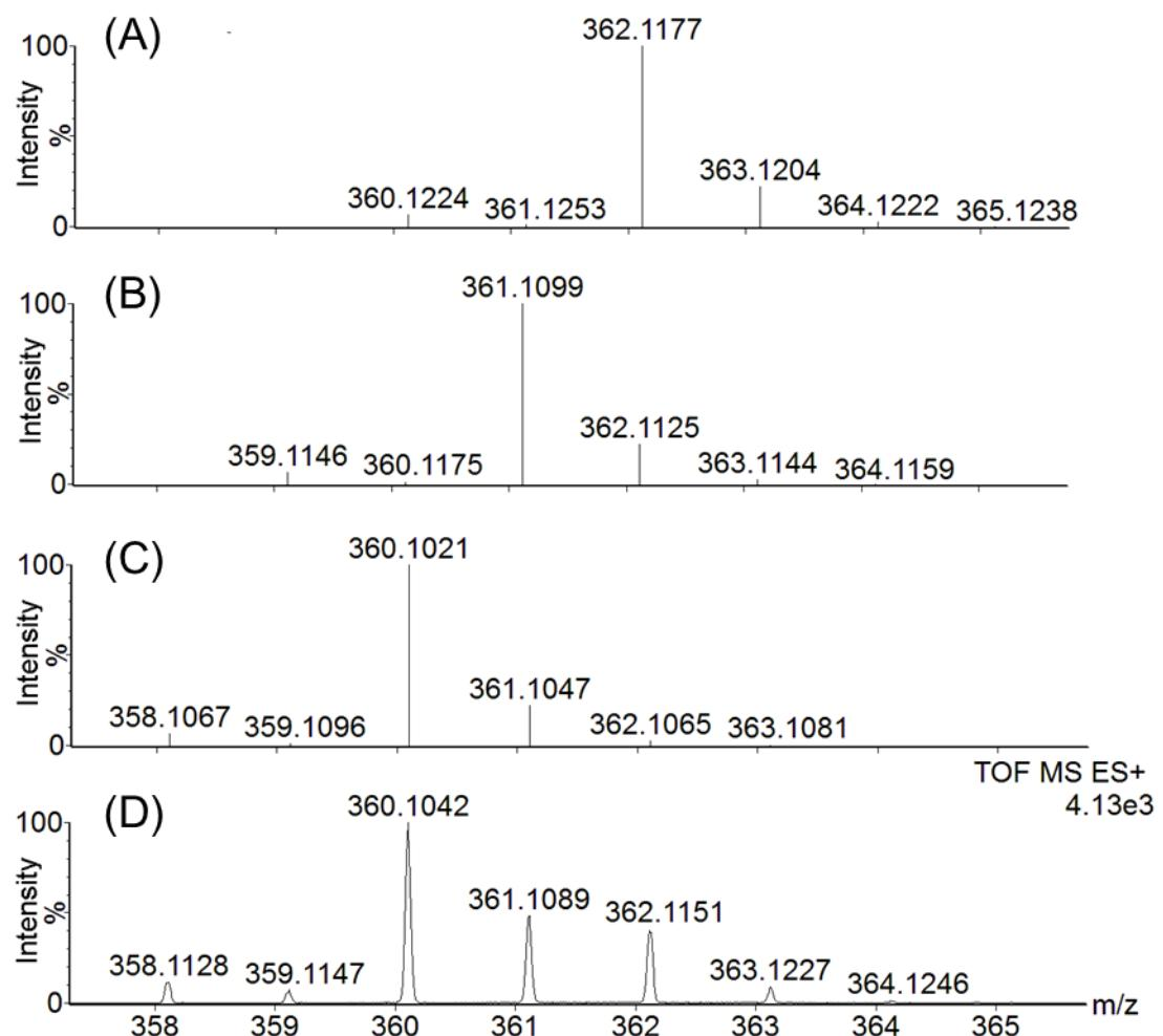
**Fig. S24** ESI-MS measurement of the species at  $m/z$  360.1042 in reaction of **1** with NaIO<sub>4</sub> (800 equiv) in H<sub>2</sub><sup>18</sup>O. (A) Simulated isotopic pattern for [Fe<sup>III</sup>(L1)(<sup>18</sup>OH)<sub>2</sub>]<sup>+</sup>. (B) Simulated isotopic pattern for [Fe<sup>IV</sup>(L1)(<sup>18</sup>O)(<sup>18</sup>OH)]<sup>+</sup>. (C) Simulated isotopic pattern for [Fe<sup>V</sup>(L1)(<sup>18</sup>O)<sub>2</sub>]<sup>+</sup>. (D) Experimental isotopic pattern.
