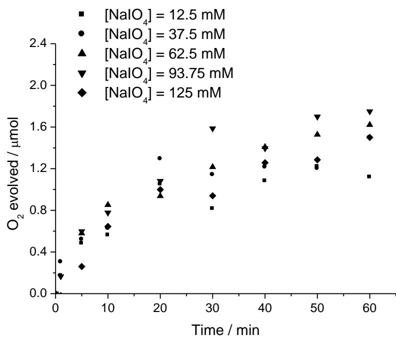
**Fig. S3** Plot of O<sub>2</sub> evolution in **1**-catalysed water oxidation with NaIO<sub>4</sub> in 0.1 M HNO<sub>3</sub> with time for different concentrations of NaIO<sub>4</sub>. Concentration of **1**: 12.5 μM.
