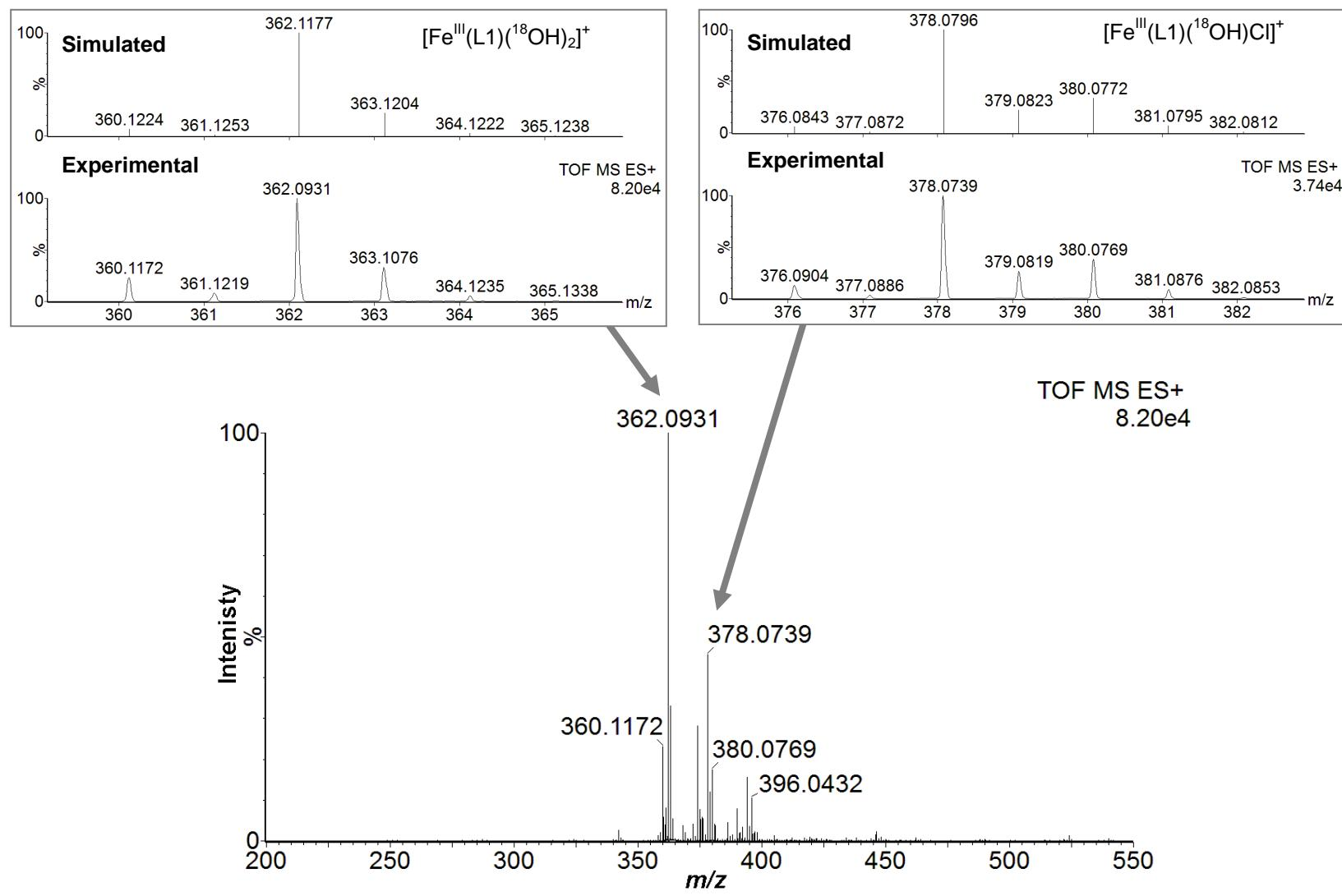
**Fig. S12** ESI mass spectrum of **1** in H<sub>2</sub><sup>18</sup>O.
