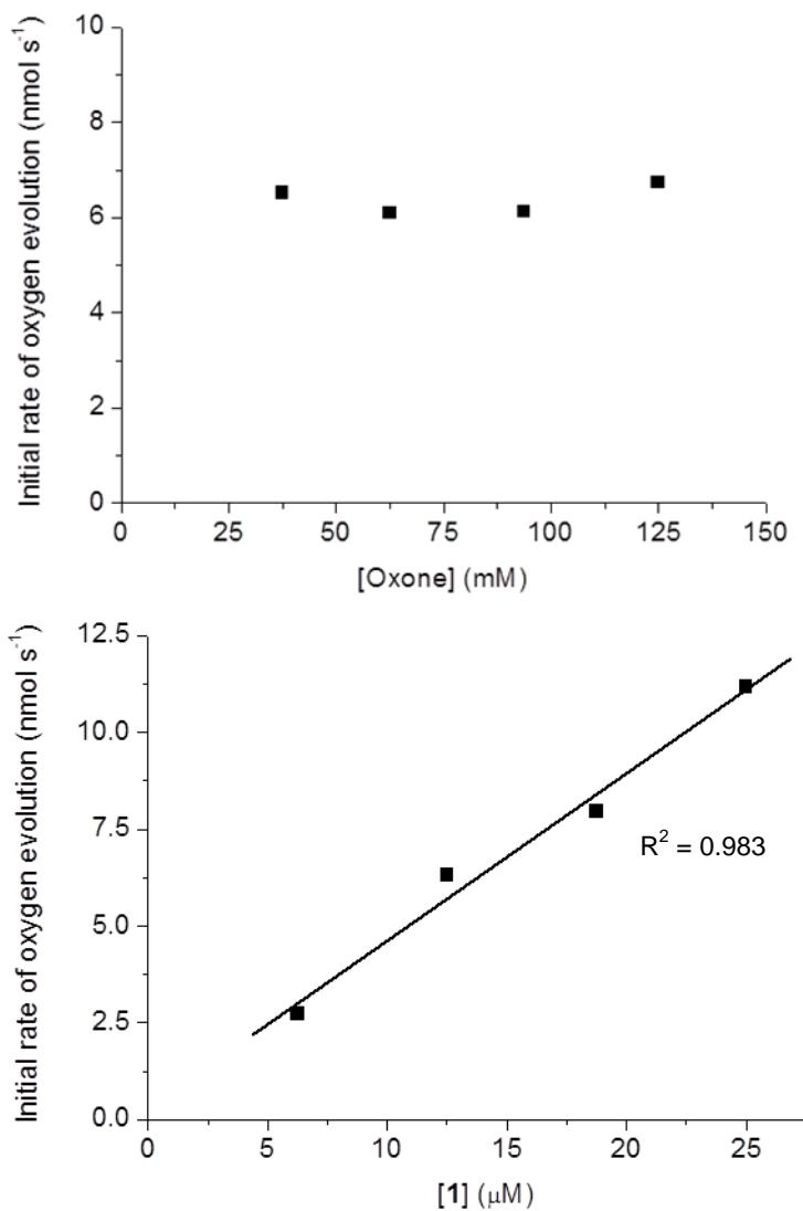
**Fig. S8** Upper: Plot of initial rate of O<sub>2</sub> evolution against different [Oxone] (37.5–125 mM) at fixed [1] (12.5 μM) in 0.1 M HNO<sub>3</sub>. Lower: Plot of initial rate of O<sub>2</sub> evolution against different [1] (6.25–25.0 μM) at fixed [Oxone] (125 mM) in 0.1 M HNO<sub>3</sub>.
