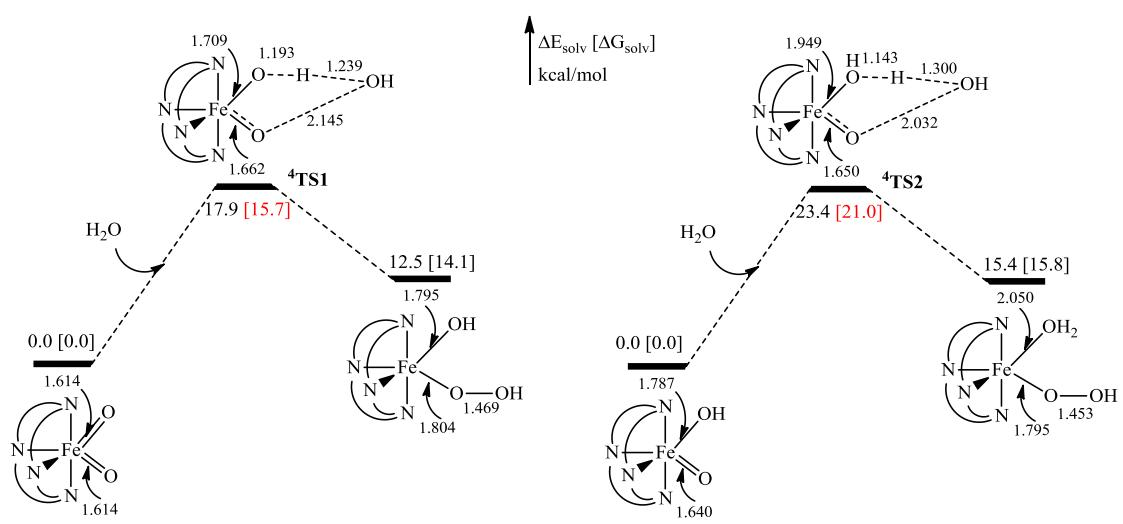
**Fig. S34** Comparison of potential energy surfaces of the first step of water oxidation based on  $[\text{Fe}^{\text{V}}(\text{L1})(\text{O})_2]^+$  and  $[\text{Fe}^{\text{V}}(\text{L1})(\text{O})(\text{OH})]^{2+}$  (free energy in kcal/mol and bond distance in Å ).
