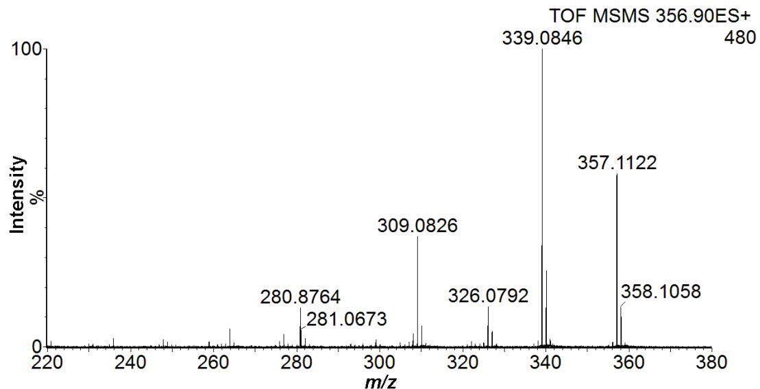
**Fig. S15** Collision-induced dissociation of the ion with  $m/z$   $\sim$ 357.1 (for the reaction of **1** with CAN (200 equiv) in 0.1 M  $\text{HNO}_3$ ) recorded at the collision energy of 15 eV.
