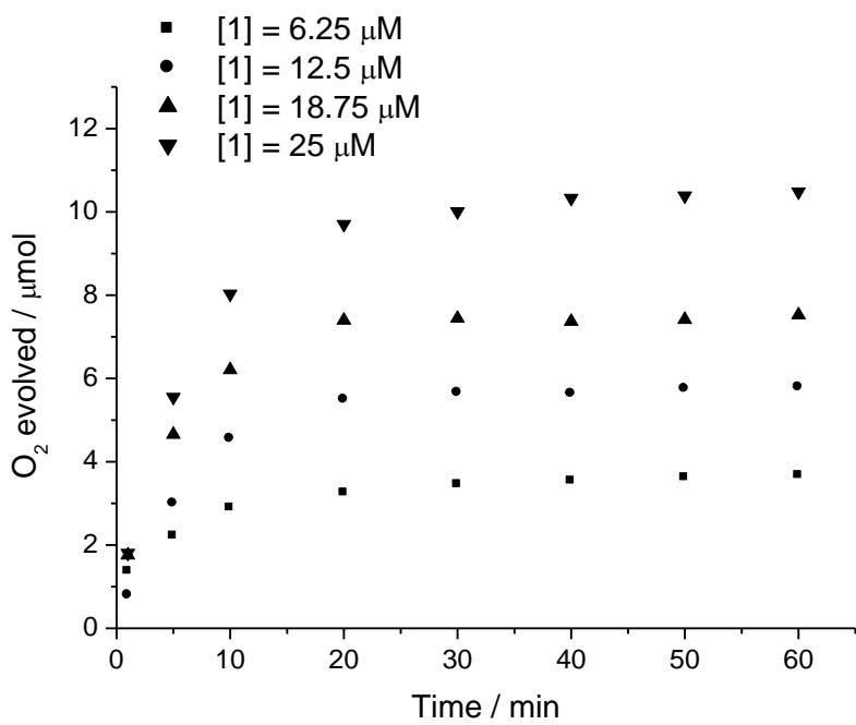
**Fig. S6** Plot of  $\text{O}_2$  evolution in **1**-catalysed water oxidation with Oxone in 0.1 M  $\text{HNO}_3$  with time for different concentrations of **1**. Concentration of Oxone: 125 mM.
