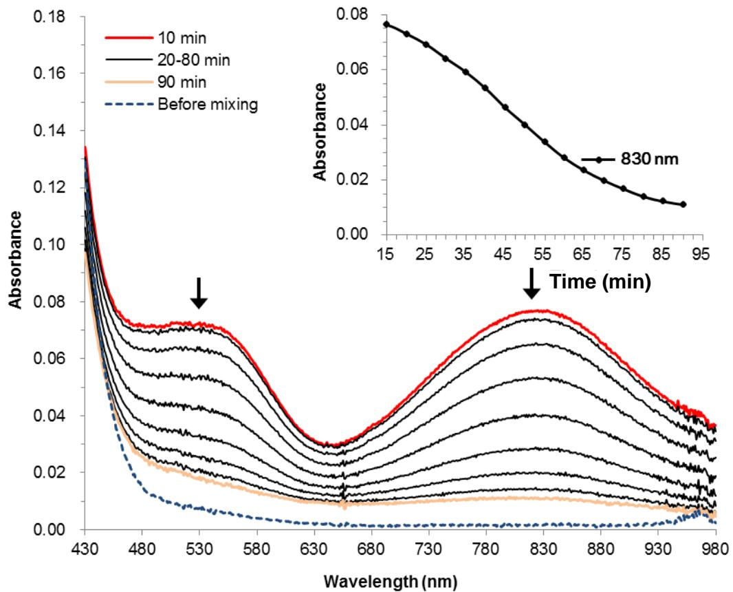
**Fig. S26** UV-vis absorption spectral changes for the reaction of **1** (1.5 mM) with NaIO<sub>4</sub> (7.5 mM) in 0.1 M HNO<sub>3</sub> at room temperature at reaction times of 10–90 min. Inset: Time course of the decay of absorption band monitored at 830 nm.
