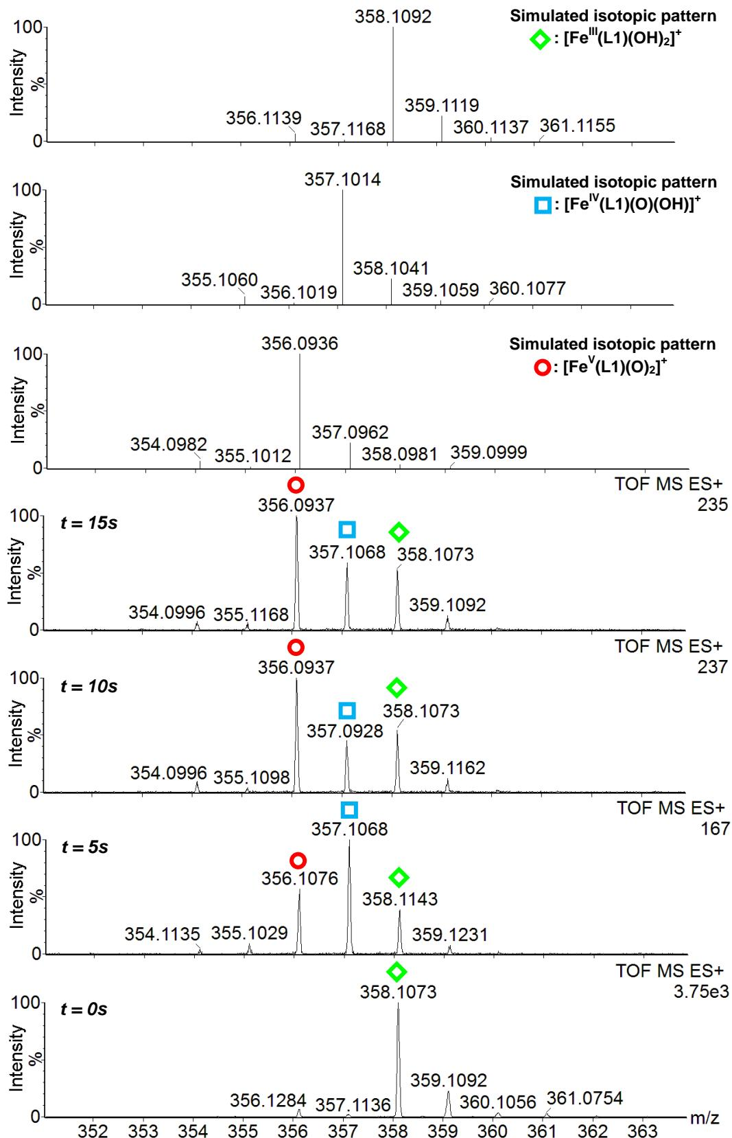
**Fig. S23** ESI-MS measurements of the reaction mixture of **1** with  $\text{NaIO}_4$  (800 equiv) in  $\text{H}_2\text{O}$  at different reaction time ( $t$ ): 0 sec (without  $\text{NaIO}_4$ ), 5 sec, 10 sec and 15 sec.
