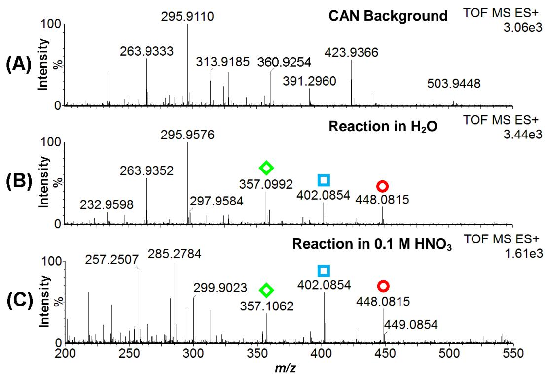
**Fig. S13** ESI-MS analysis of the reaction mixture of **1** with CAN in  $\text{H}_2\text{O}$  and in 0.1 M  $\text{HNO}_3$ : (A) CAN in  $\text{H}_2\text{O}$  only, (B) Reaction of **1** with CAN (200 equiv) in  $\text{H}_2\text{O}$  and (C) Reaction of **1** with CAN (200 equiv) in 0.1 M  $\text{HNO}_3$ .
