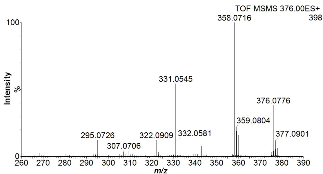
**Fig. S11** Collision-induced dissociation of  $[\text{Fe}^{\text{III}}(\text{L1})(\text{OH})\text{Cl}]^+$  generated in the solution of **1** in  $\text{H}_2\text{O}$  recorded at the collision energy of 20 eV.
