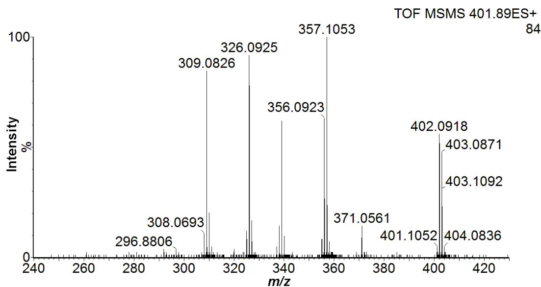
**Fig. S16** Collision-induced dissociation of the ion at  $m/z \sim 402.1$  (for the reaction of **1** with CAN (200 equiv) in 0.1 M HNO<sub>3</sub>) recorded at the collision energy of 12 eV.
