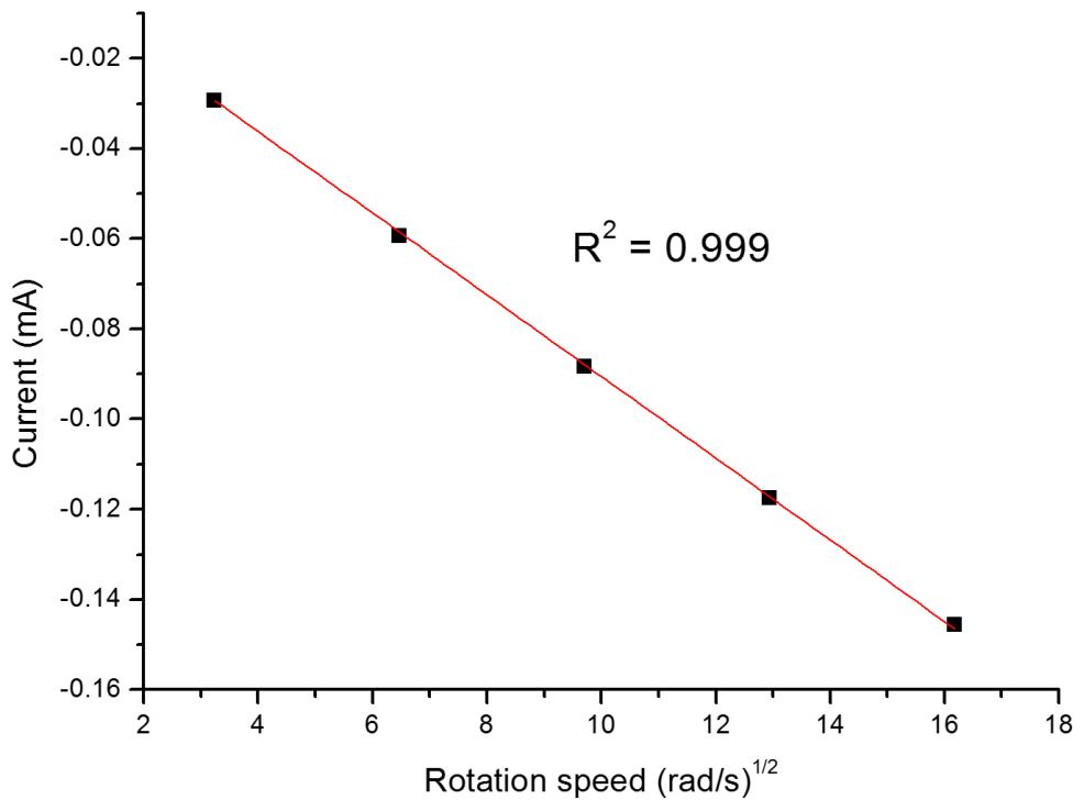
**Fig. S31** Levich plot for the limiting current of the redox process corresponding to the reversible couple I.
