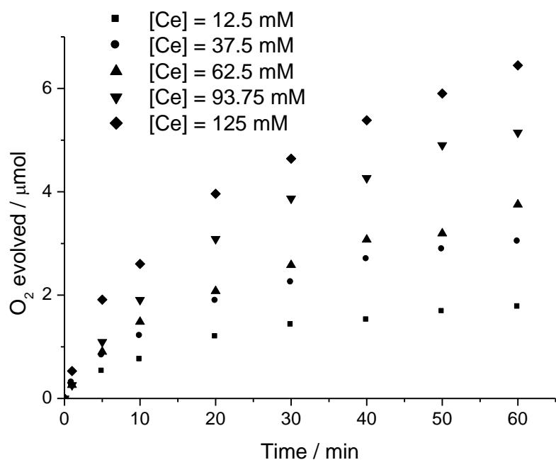
**Fig. S1** Plot of  $O_2$  evolution in **1**-catalysed water oxidation with CAN in 0.1 M  $HNO_3$  with time for different concentrations of CAN. Concentration of **1**: 12.5  $\mu M$ .
