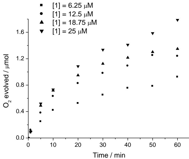
**Fig. S4** Plot of O<sub>2</sub> evolution in **1**-catalysed water oxidation with NaIO<sub>4</sub> in 0.1 M HNO<sub>3</sub> with time for different concentrations of **1**. Concentration of NaIO<sub>4</sub>: 125 mM.
