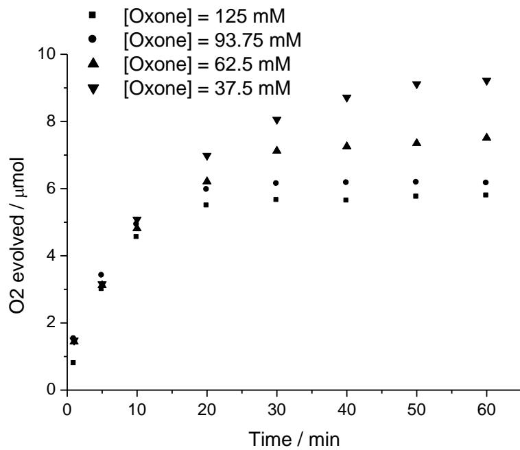
**Fig. S7** Plot of  $\text{O}_2$  evolution in **1**-catalysed water oxidation with Oxone in 0.1 M  $\text{HNO}_3$  with time for different concentrations of Oxone. Concentration of **1**: 12.5  $\mu\text{M}$ .
