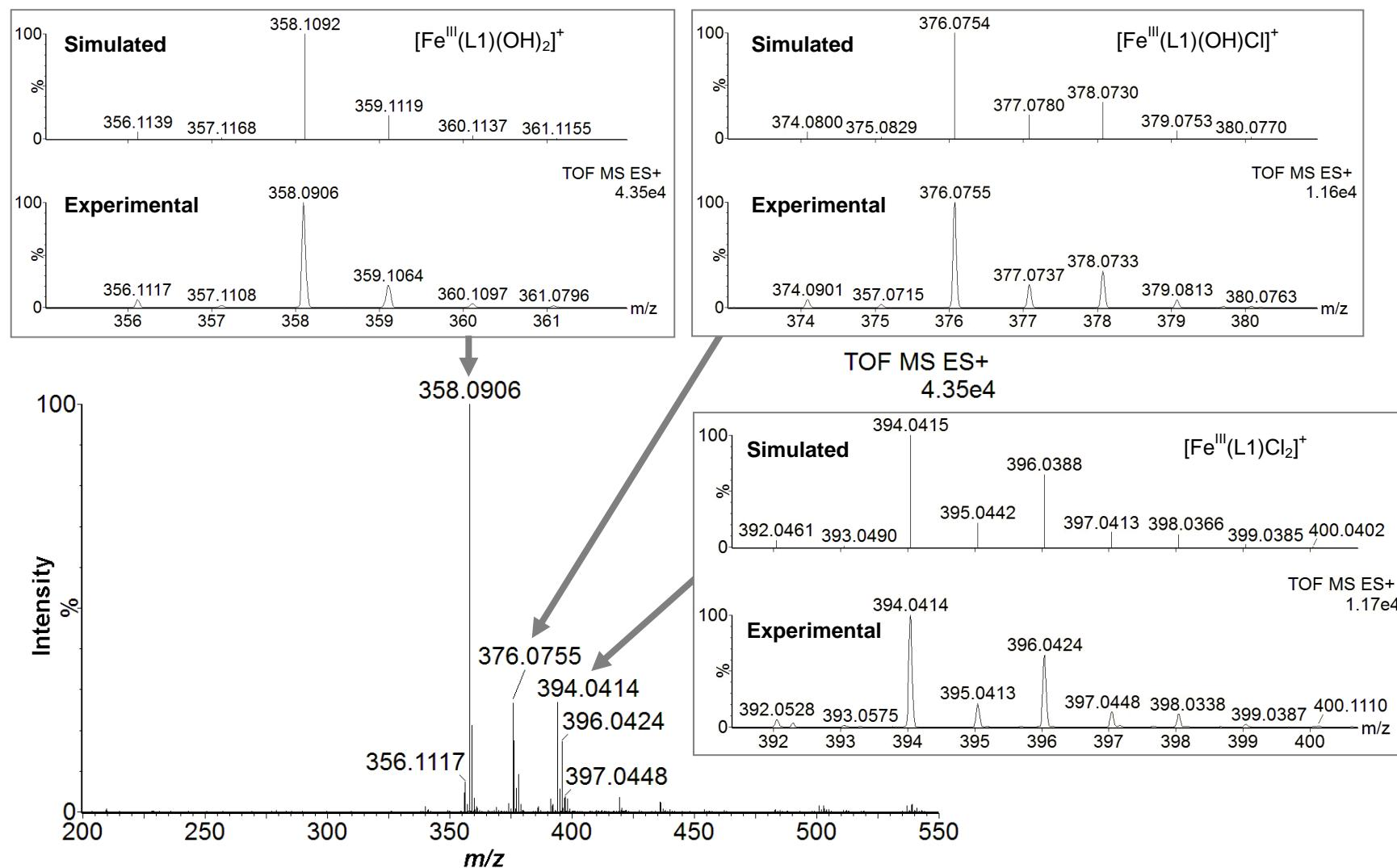
**Fig. S9** ESI mass spectrum of **1**· $\text{FeCl}_4$  in  $\text{H}_2\text{O}$ .
