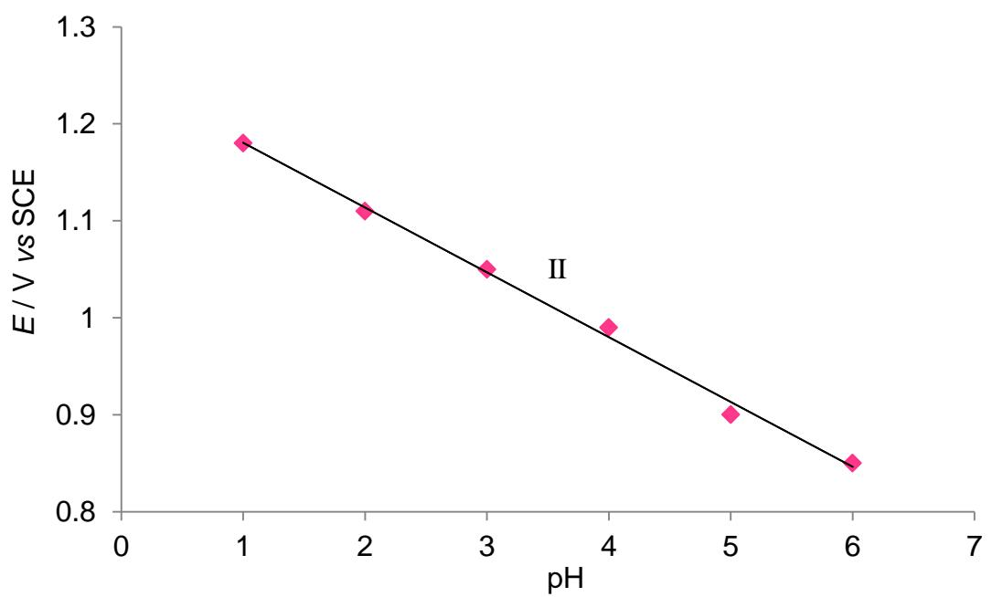
**Fig. S28** Redox potentials (the irreversible wave II) of **1**· $\text{ClO}_4$  in solutions at various pH.
