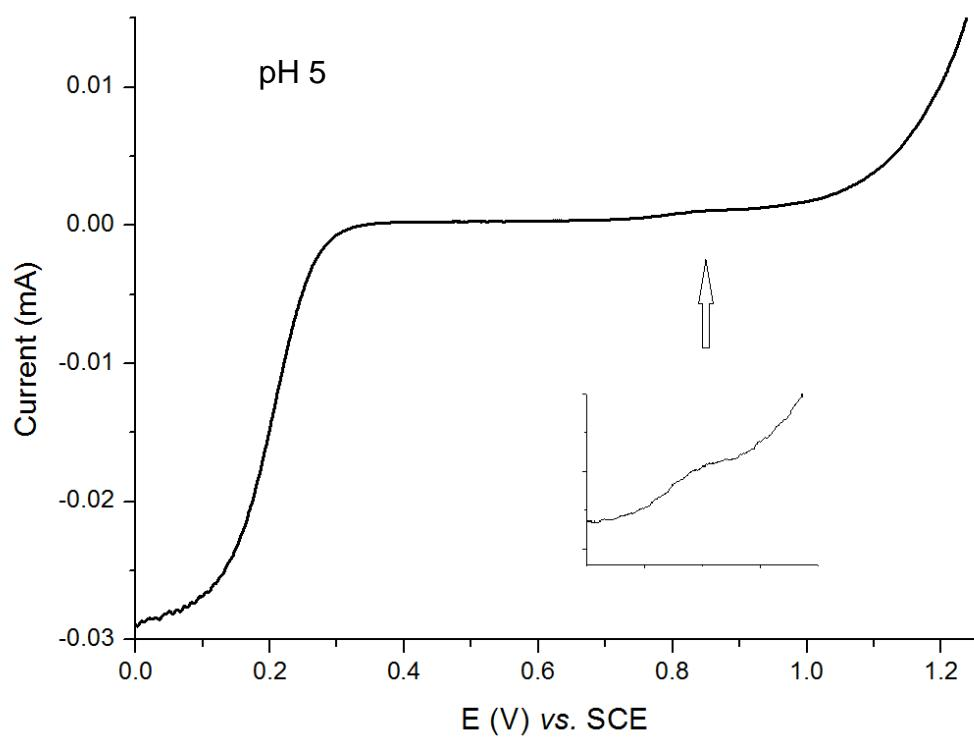
**Fig. S29** Linear scan voltammograms of **1**·ClO<sub>4</sub> in 0.1 M HNO<sub>3</sub> at pH 1 (rotation rate: 100 rpm; inset: magnified region at approximately 1.1 V) and at pH 5 (rotation rate: 400 rpm; inset; magnified region at approximately 0.9 V). Working electrode: rotating glassy carbon disk; scan rate: 5 mV/s.
