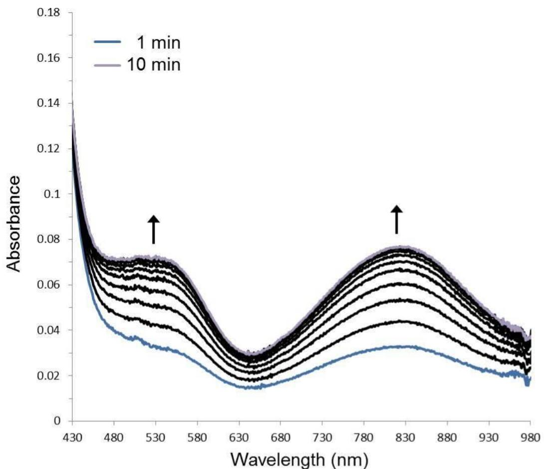
**Fig. S25** UV-vis absorption spectral changes for the reaction of **1** (1.5 mM) with NaIO<sub>4</sub> (7.5 mM) in 0.1 M HNO<sub>3</sub> at room temperature at reaction times of 1–10 min.
