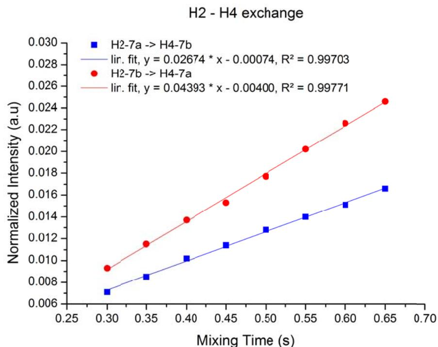
**Figure SI-4:** Arrhenius plot of the mixing series H<sub>2</sub>→H<sub>4</sub> (blue, H<sub>2</sub> of **7a** was irradiated at 5.60 ppm and the intensity of H<sub>4</sub>-**7b** at 3.58 ppm was measured) and H<sub>2</sub>→H<sub>4</sub> (red, H<sub>2</sub> of **7b** was irradiated at 5.99 ppm and intensity of H<sub>4</sub>-**7a** at 3.95 ppm was measured) at  $T = 320$  K.
