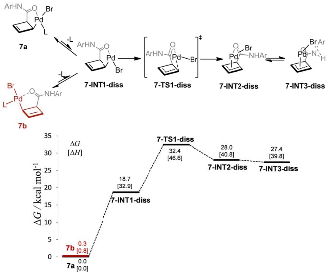
**Figure S1.** Computed Gibbs free energy profile (298.15 K) for phosphine dissociation and subsequent  $\eta^1 \rightarrow \eta^3$  transition. SMD(THF)-B3LYP-D3/def2-TZVP//B3LYP-D3/def2-SVP(def2-TZVP for Pd). L=L2c.
