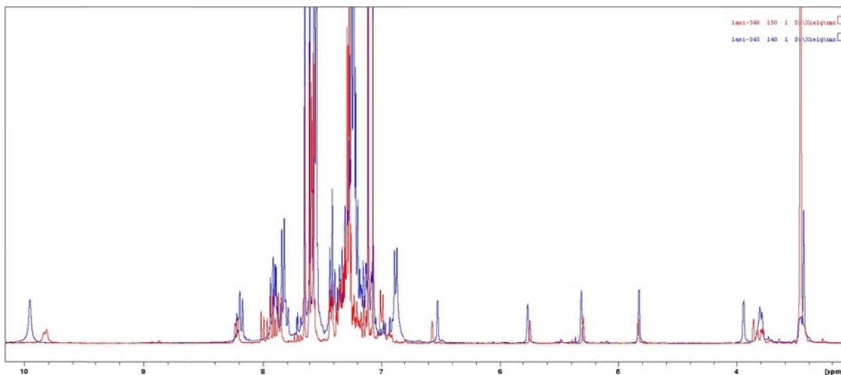
Figure SI-9:  $^1\text{H}$  NMR spectrum of **7a/b**. Blue: 0.1 M, red: 0.01 M in  $\text{THF}-d_8$ .
