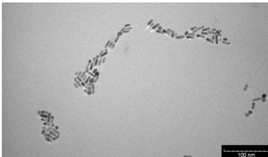
Figure S9. TEM image of short Au nanorods formed at the low \text{Ag}^+ concentration (i.e., 0.04 mM) without the addition of toluene.
