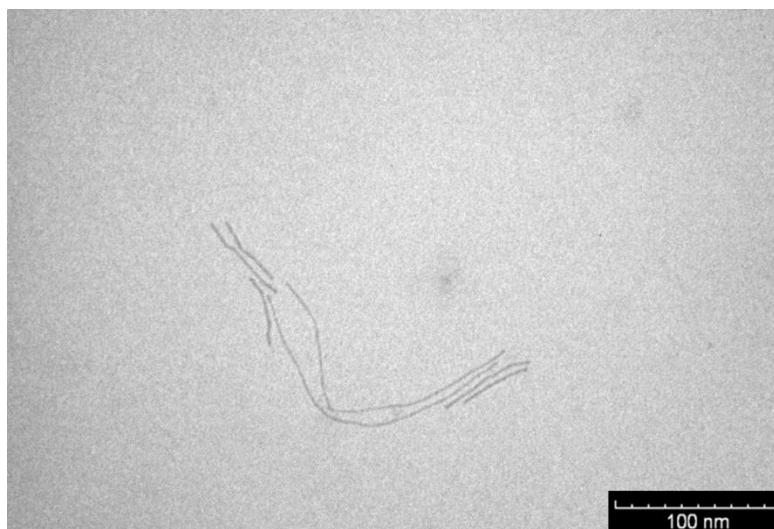
Figure S12. TEM image of ultrathin Au nanowires formed by adding a 80- \mu l chloroform to the Au growth solution after adding the Au seed solution. The growth solution was prepared by mixing 10 ml 0.1M CTAB aqueous solution with 0.5 ml 10 mM HAuCl 4 , 40 \mu l 0.1 M AgNO 3 and 0.5 ml 0.1 M hydroquinone aqueous solution.
