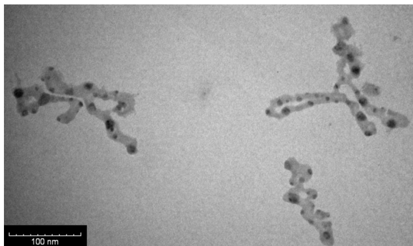
Figure S7. TEM image of Au nanostructures with irregular shapes formed at low \text{Ag}^+ ion concentration (i.e., 0.04 mM by adding 40- \mu\text{l} 0.01M \text{Ag}^+ solution to a 10-ml Au growth solution) with the addition of 100- \mu\text{l} toluene. The concentration of CTAB was 0.1M.
