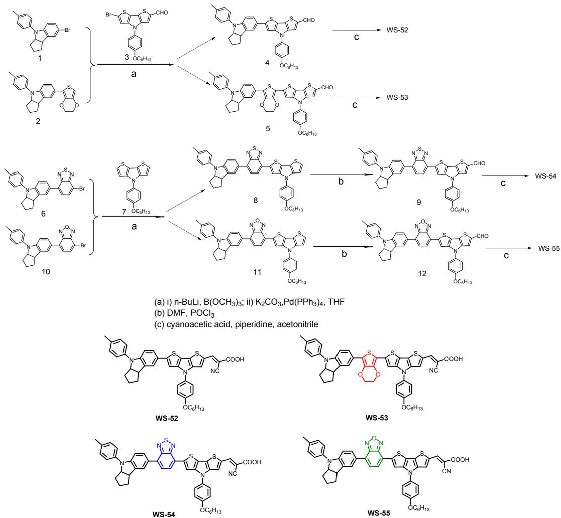
**Scheme 1.** Synthetic route of target dyes **WS-52**, **WS-53**, **WS-54** and **WS-55** containing different auxiliary groups for targeted customization of molecular energy levels.
