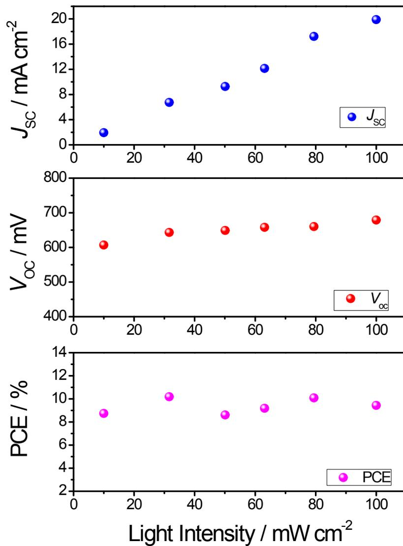
**Figure S7.** Photoelectric parameters ( $J_{SC}$ ,  $V_{OC}$  and PCE) under different light intensity based on Dye WS-55.
