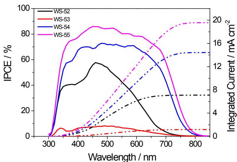
**Figure S3.** (Above) IPCE spectra of **WS-52**, **WS-53**, **WS-54** and **WS-55** (solid line), and their corresponding integrated current curves (dash dot line). Note: the integrated current for different dyes **WS-52**, **WS-53**, **WS-54** and **WS-54** are 7.10, 1.17, 14.43 and 19.56 mA cm<sup>-2</sup>, respectively, which are in good agreement with the measured photocurrent  $J_{SC}$  (7.88, 1.22, 15.84 and 19.66 mA cm<sup>-2</sup>).
