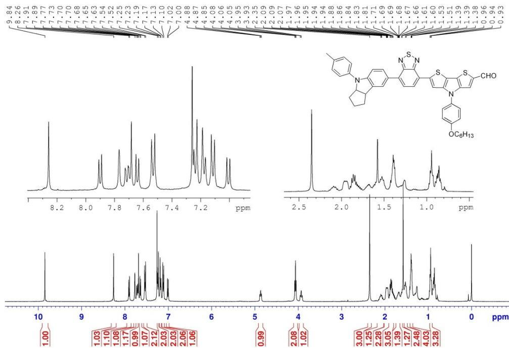
Figure S21. <sup>1</sup>H NMR of compound 9 in CDCl<sub>3</sub>
