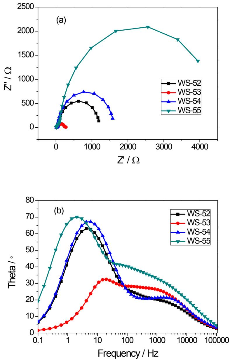
**Figure S5.** Impedance spectra of DSSCs based on WS-52, WS-53, WS-54 and WS-55 measured at 0.55 V bias in the dark. (a) Nyquist plots; (b) Bode phase plots.
