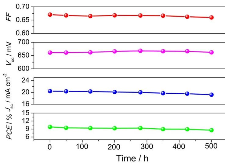
**Figure S4.** Variations of the photovoltaic parameters ( $FF$ ,  $V_{oc}$ ,  $J_{sc}$  and  $PCE$ ) with aging time for the DSSC device based on **WS-55** under visible-light soaking.
