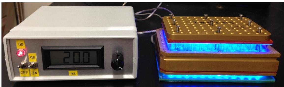
**Figure S6.** LED Driver – Exterior View
