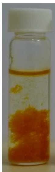
Figure S1. The precipitation of the complex formed by PEG ( M_w = 6000 ) and iodine.
