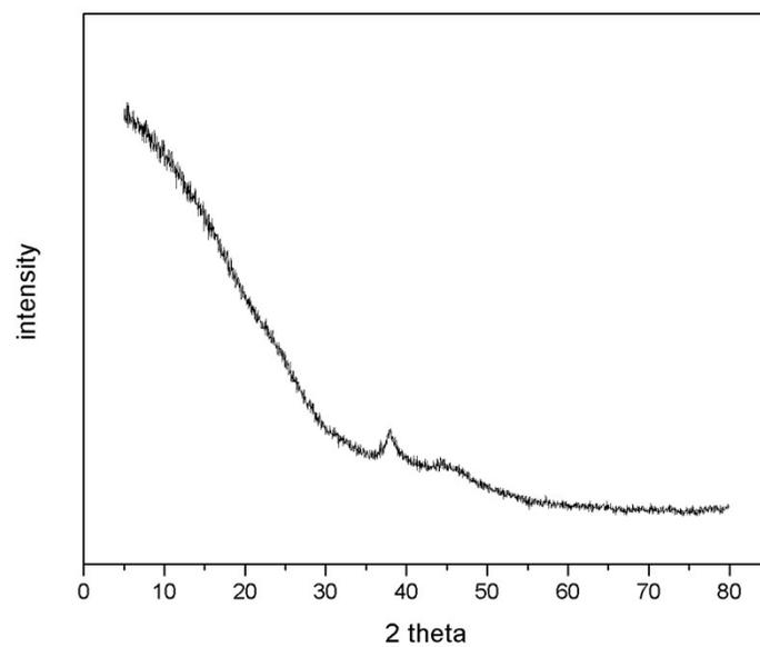
**Figure S3.** XRD pattern of Au@BnCD-HCPP.
