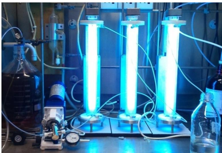
Figure 1. FEP flow photochemical reactor
