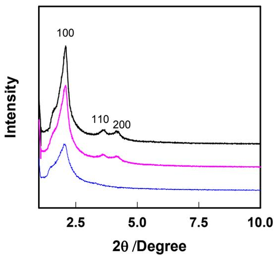
**Fig. S8.** Small-angle powder XRD patterns of MSN-Cl (black line), MSN-CD (pink line) and Rhod-H-NO@MSN-CD (blue line).
