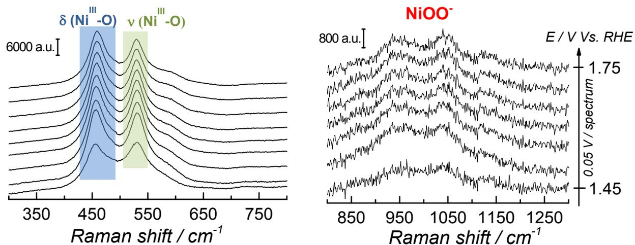
**Figure S5.** SER spectra obtained at constant potential during the electrochemical oxidation of Ni(OH)<sub>2</sub> and the subsequent OER on NiOOH at pH 13. The electrolyte was prepared in H<sub>2</sub><sup>18</sup>O. The left panel presents the spectra in the wavenumber region 300 – 800 cm<sup>-1</sup> and the right panel presents the wavenumber region 800 – 1300 cm<sup>-1</sup>.
