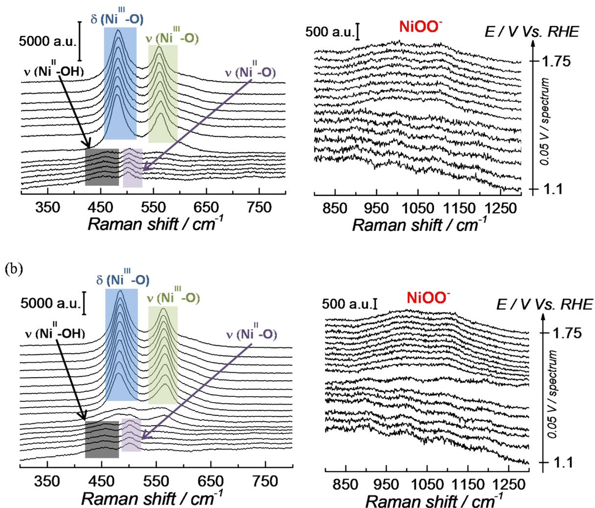
**Figure S4.** SER spectra obtained at constant potential during the electrochemical oxidation of Ni(OH)<sub>2</sub> and the subsequent OER on NiOOH at different pH's. The ionic strength of the solution was fixed to 0.1 M with NaClO<sub>4</sub>. The left panel presents the spectra in the wavenumber region 300 – 800 cm<sup>-1</sup> and the right panel presents the wavenumber region 800 – 1300 cm<sup>-1</sup>: a) pH 11.5, b) pH 14.0.
