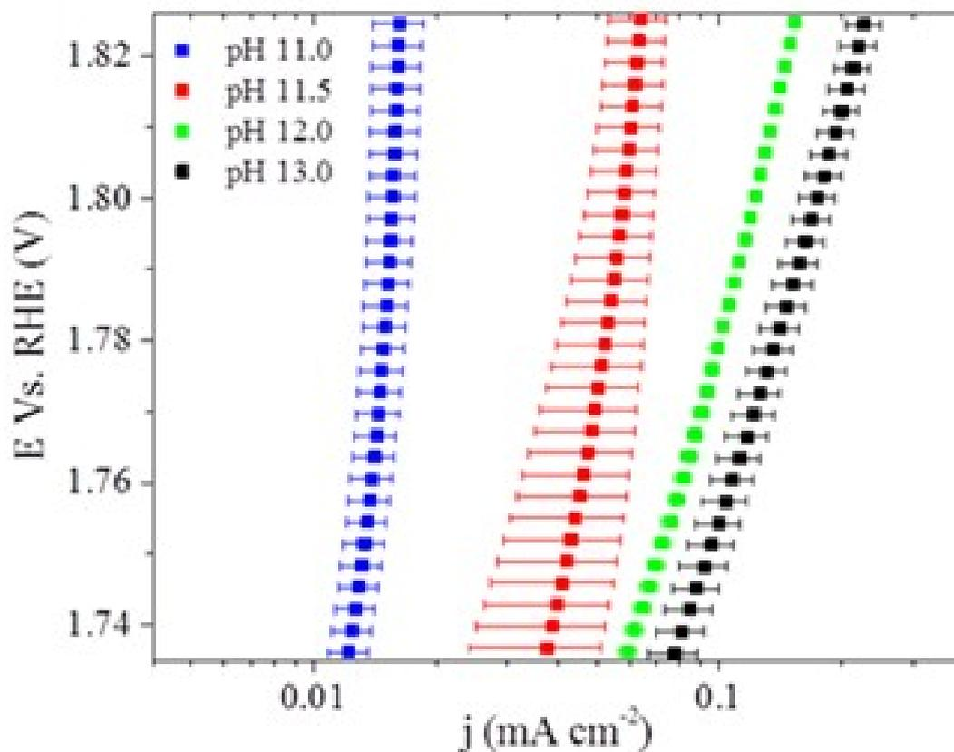
**Figure S2.** OER activity obtained from the average of the current measured in the forward and backward scan in the polarization curves of NiOOH deposited on Au (capacitance-corrected). Measurements at pH's 11 – 13 were performed at constant ionic strength, adjusted to 0.1 M with NaClO<sub>4</sub> except for pH 13, that solution was NaOH 0.1 M.
